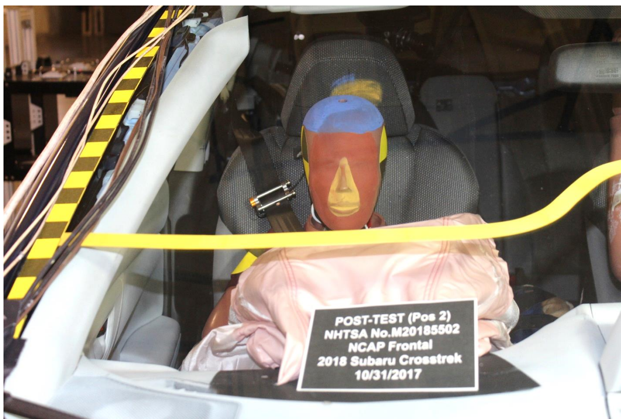
Figure A-52: Post-Test Passenger Dummy Front View
