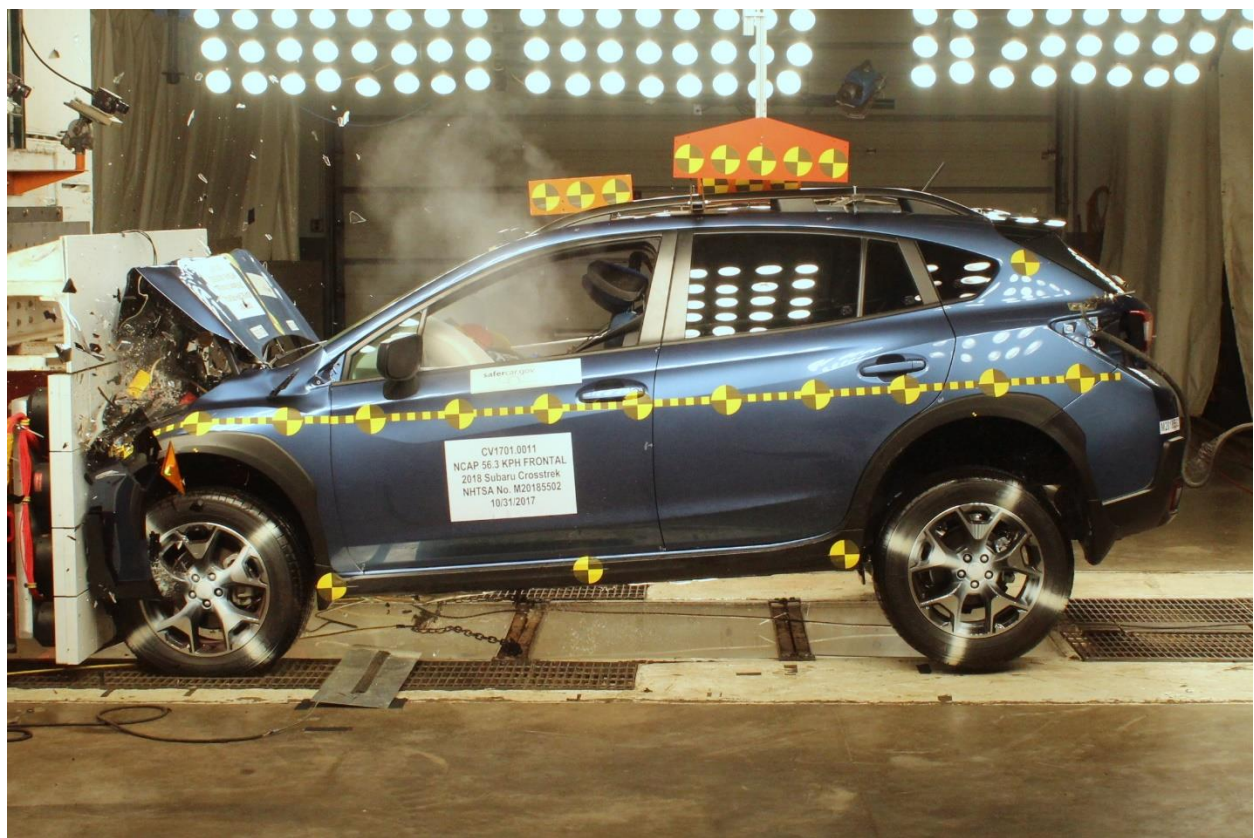
Figure A-78: 2018 Subaru Crosstrek Frontal Impact Event
