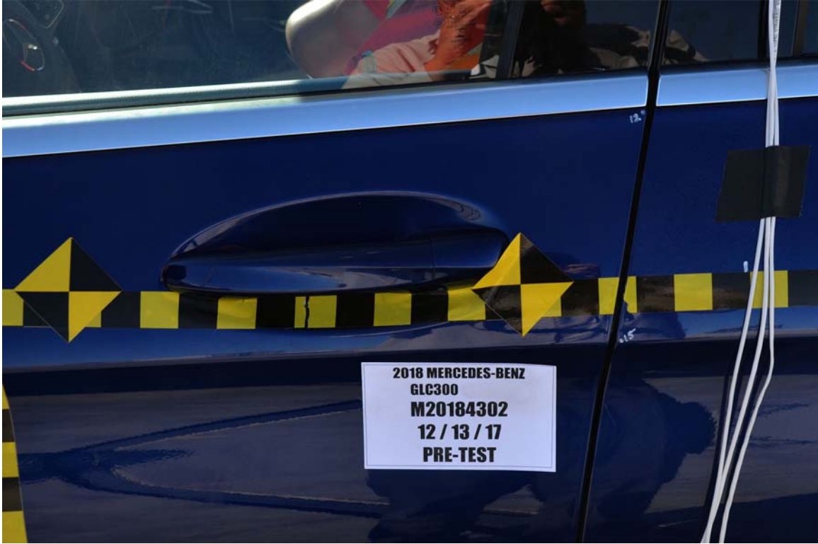
FIGURE 21. Pre-Test Left Front Door Latch Close-Up
