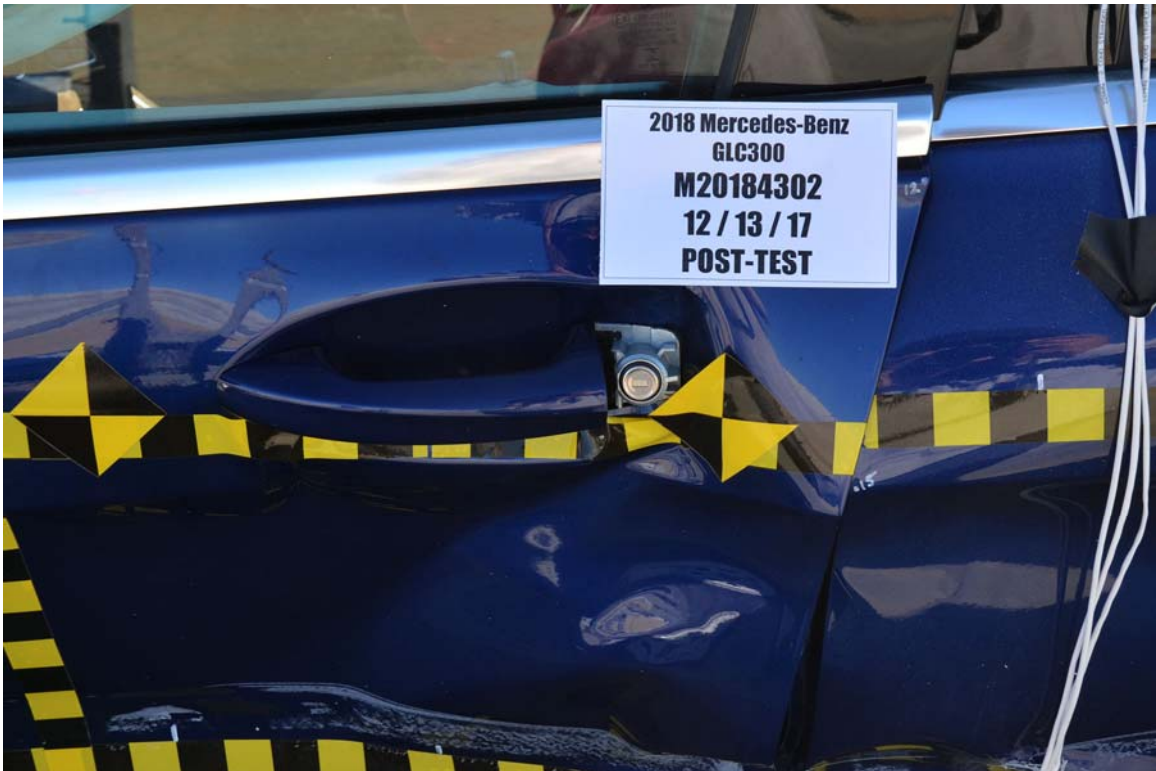
FIGURE 22. Post-Test Left Front Door Latch Close-Up
