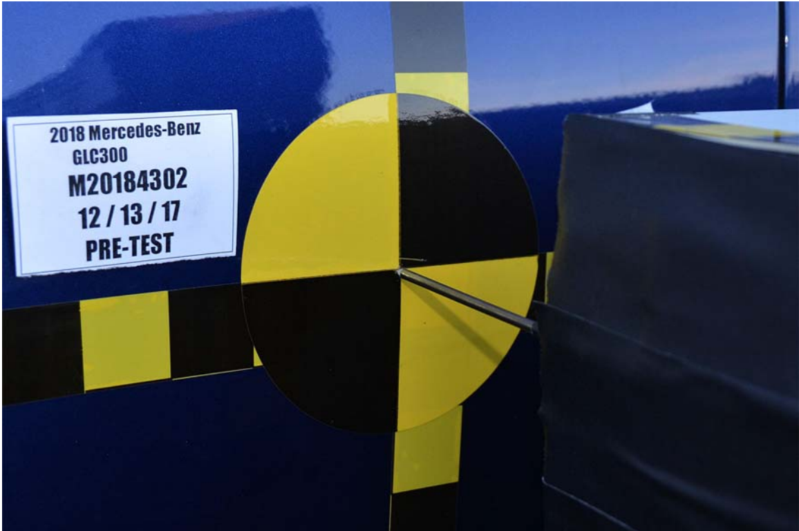
FIGURE 19. Pre-Test Close-Up View of Impact Point Target
