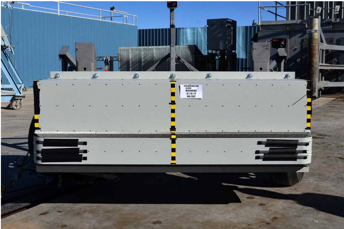
FIGURE 84. Pre-Test Front View of MDB Impactor Face
