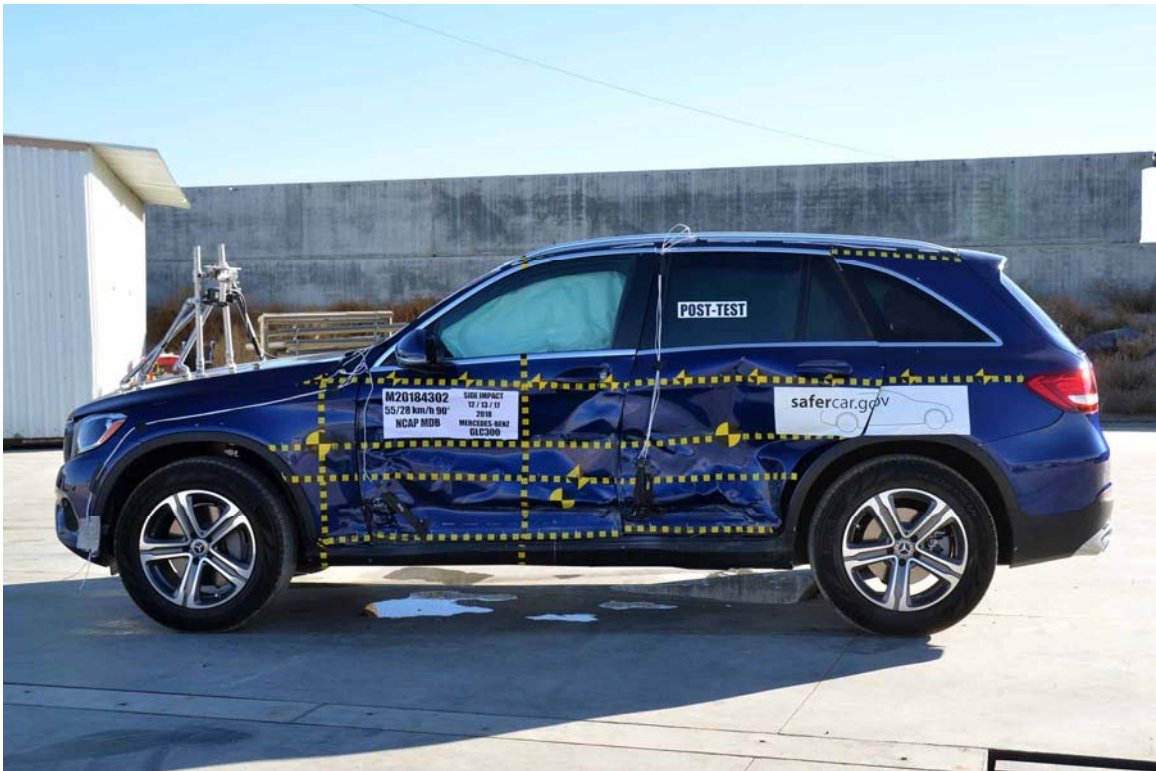
FIGURE 8. Post-Test Left Side View of Test Vehicle
