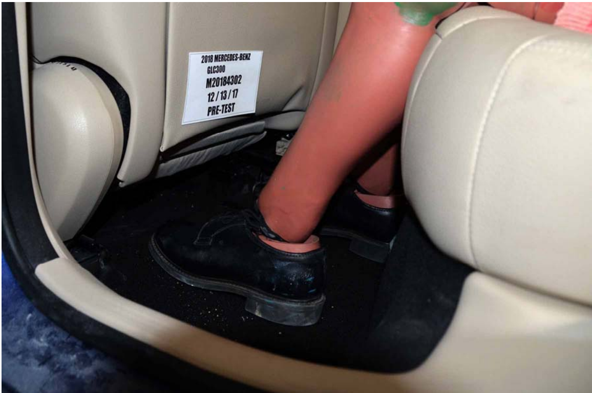
FIGURE 64. Pre-Test Placement of Rear Passenger Dummy's Feet
