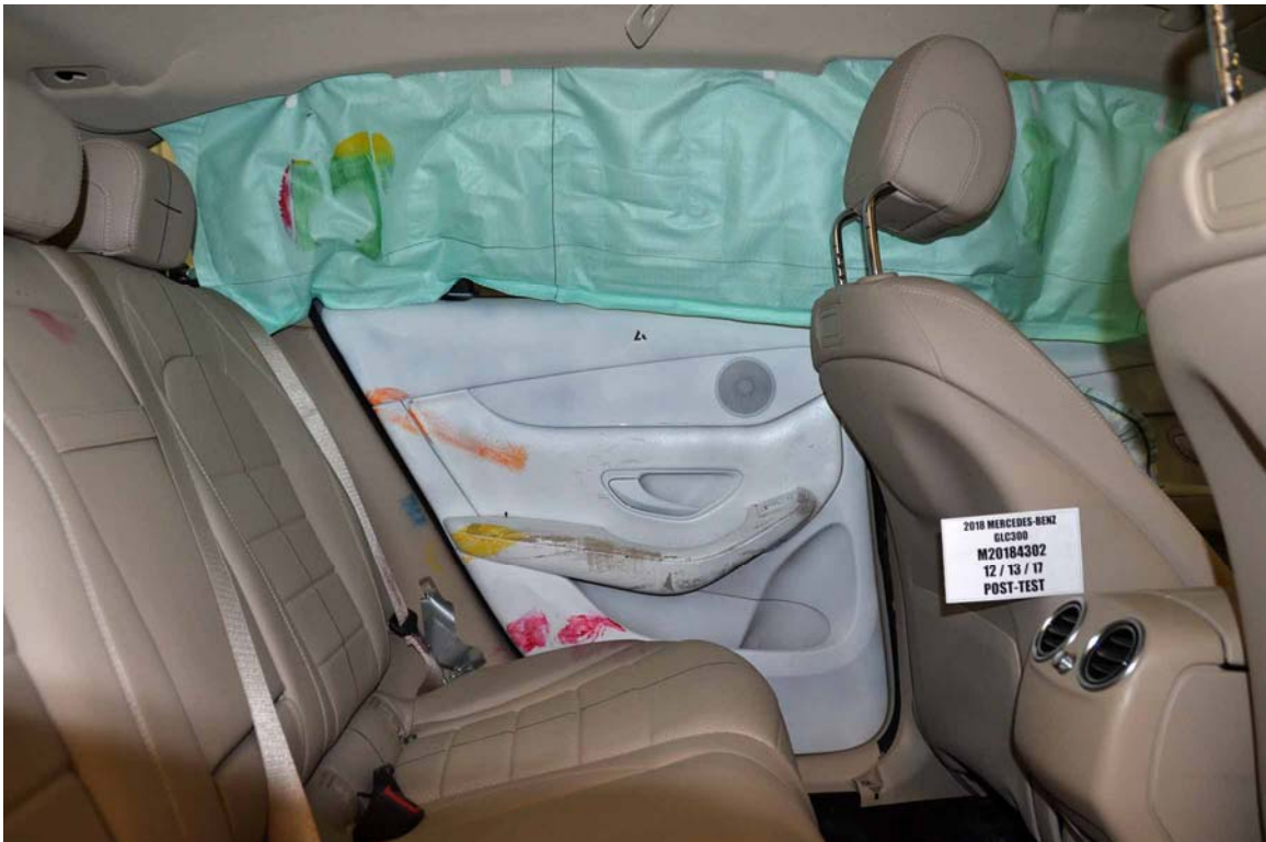
FIGURE 74. Post-Test Rear Passenger Inner Door Panel View Showing Rear Passenger Dummy Contact Locations
