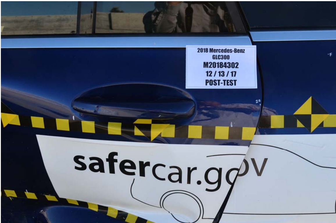
FIGURE 24. Post-Test Left Rear Door Latch Close-Up
