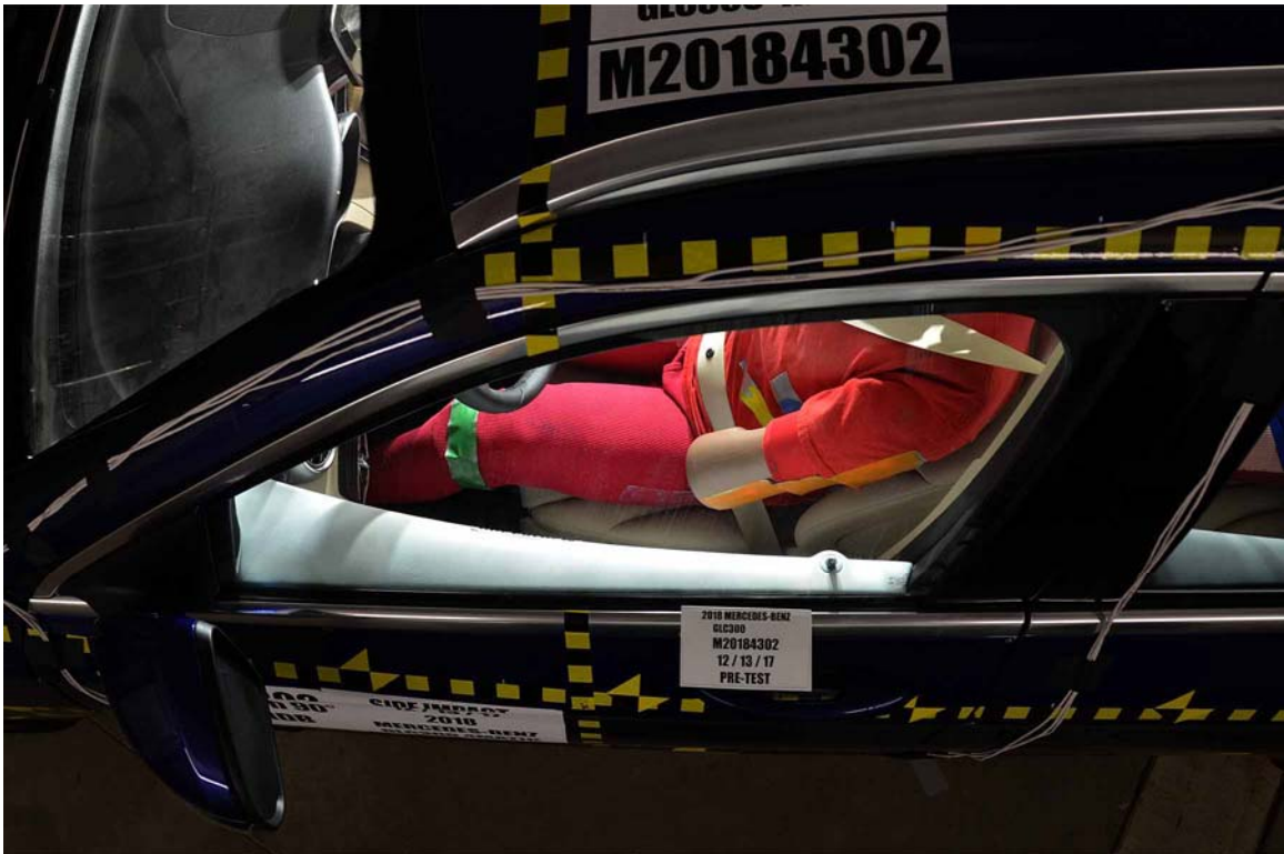
FIGURE 42. Pre-Test Driver Dummy and Door Clearance View
