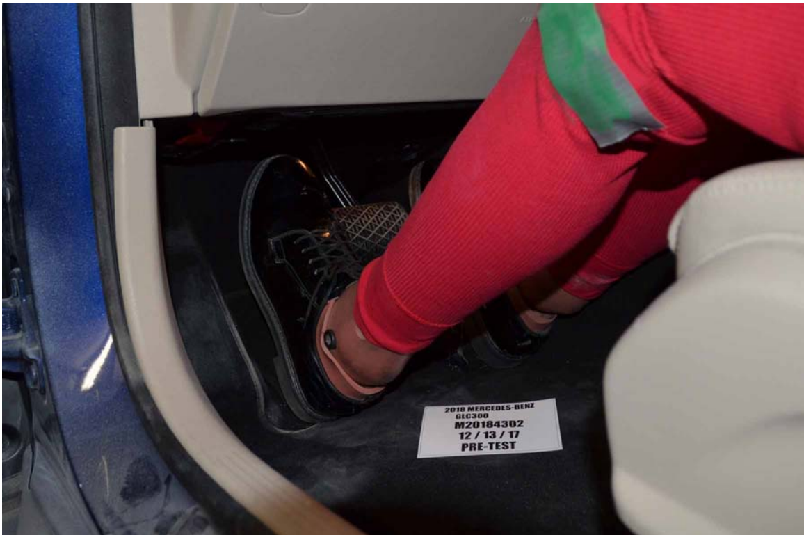
FIGURE 34. Pre-Test Placement of Driver Dummy's Feet
