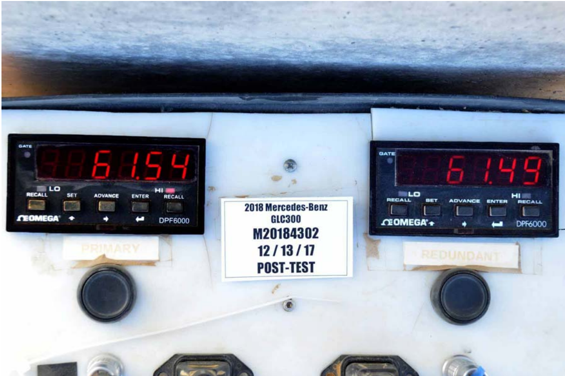
FIGURE 95. Post-Test Primary and Redundant Speed Trap Read-Out
