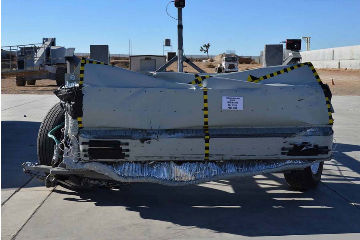
FIGURE 85. Post-Test Front View of MDB Impactor Face
