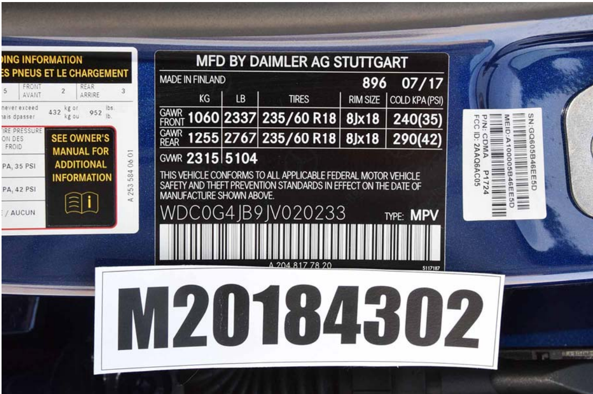
FIGURE 92. Close-Up View of Vehicle's Certification Label
