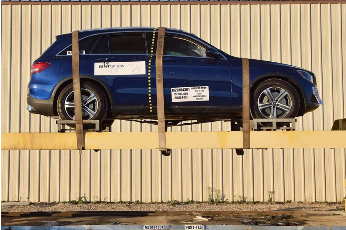
FIGURE 63. FMVSS No. 301 Static Rollover 0 Degrees
