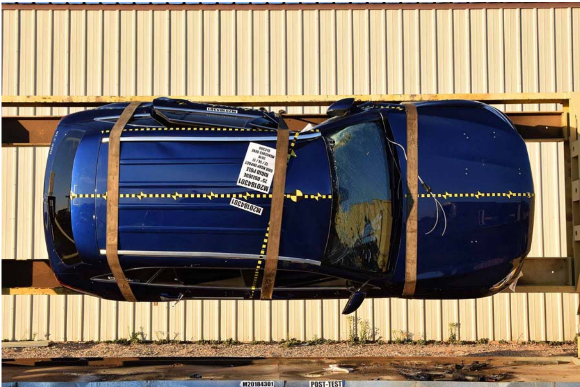
FIGURE 64. FMVSS No. 301 Static Rollover 90 Degrees
