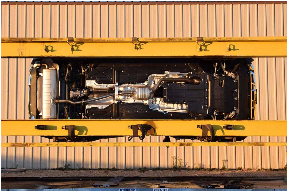
FIGURE 66. FMVSS No. 301 Static Rollover 270 Degrees
