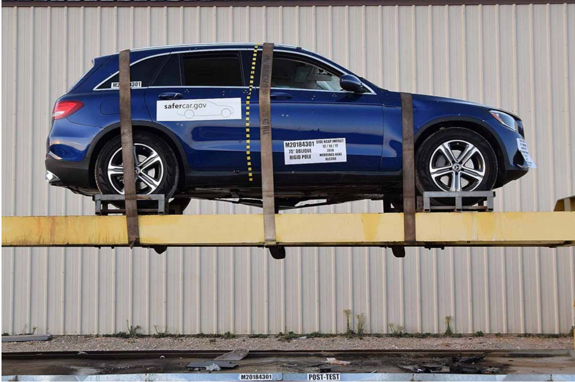
FIGURE 67. FMVSS No. 301 Static Rollover 360 Degrees
