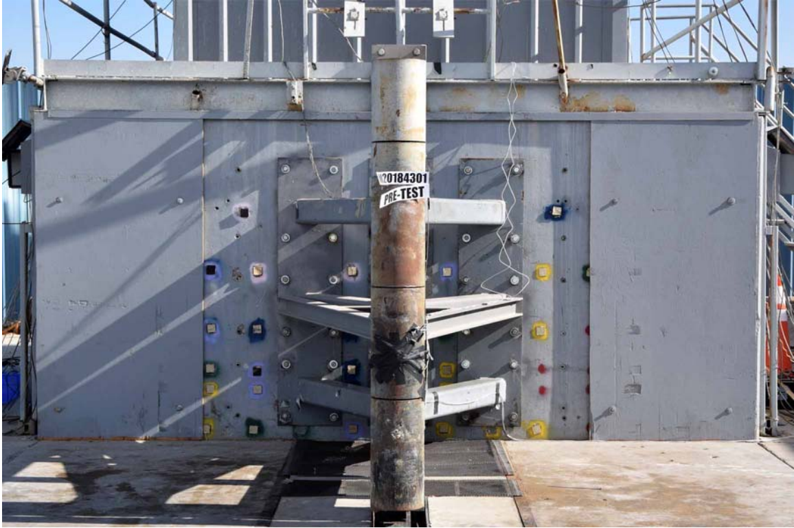
FIGURE 57. Pre-Test Pole Barrier Front View
