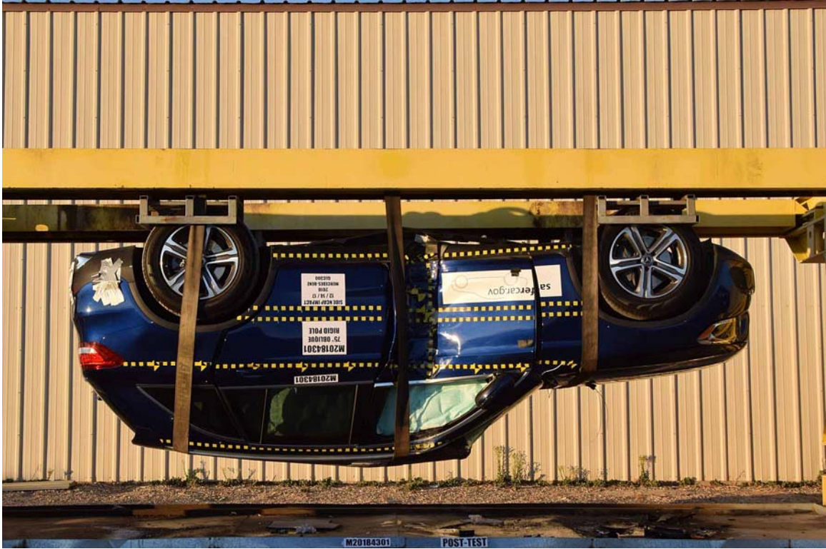
FIGURE 65. FMVSS No. 301 Static Rollover 180 Degrees
