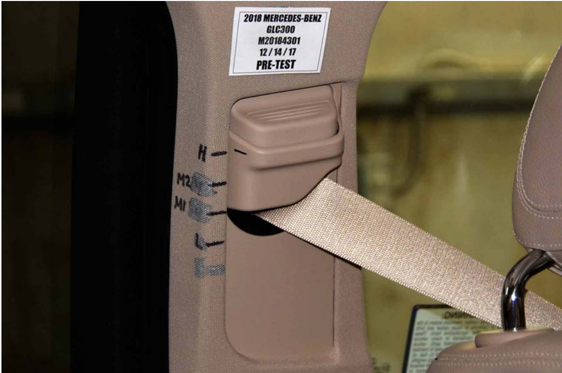
FIGURE 33. Pre-Test View of Belt Anchorage for Dummy
