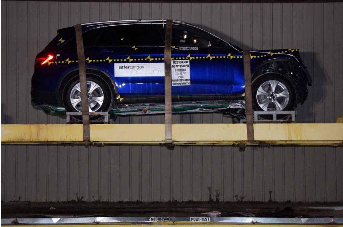
FIGURE 77. Vehicle at 360° on Static Rollover Device
