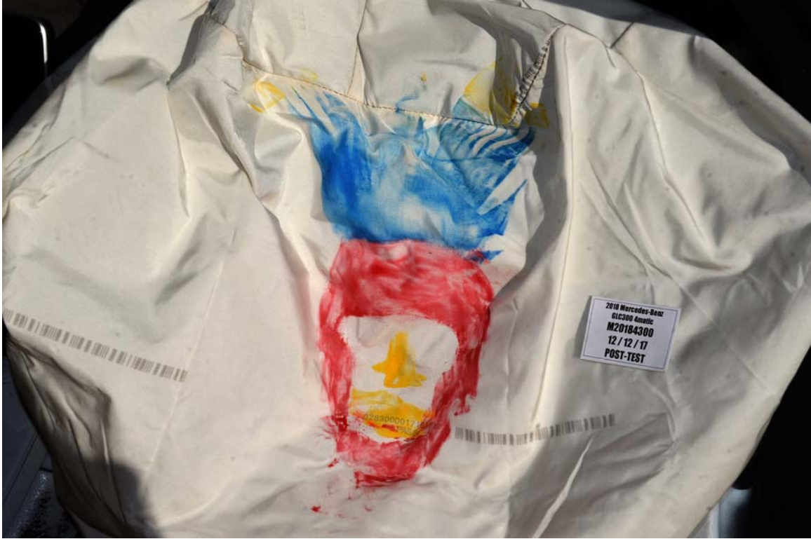
FIGURE 68. Post-Test Passenger Dummy Contact with Airbag
