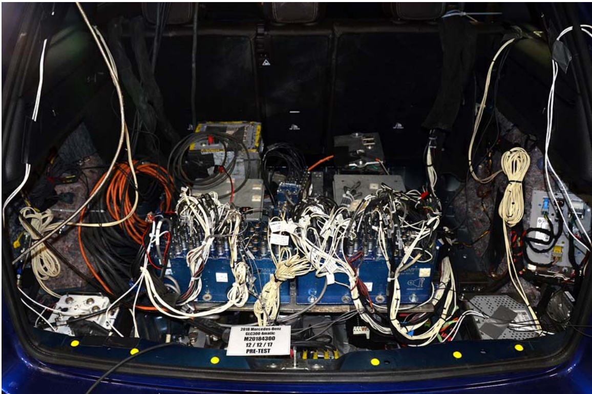
FIGURE 70. Photograph of Ballast Installed in Vehicle
