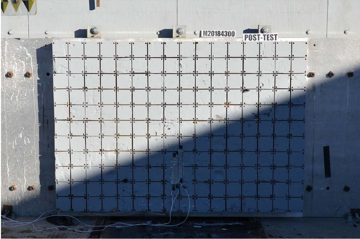
FIGURE 3. Post-Test Load Cell Wall
