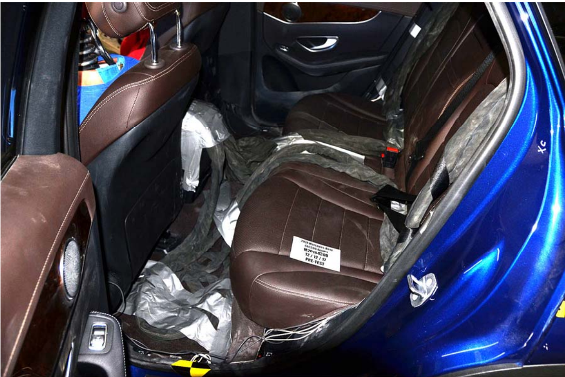
FIGURE 28. Pre-Test Dummy Cable Routing
