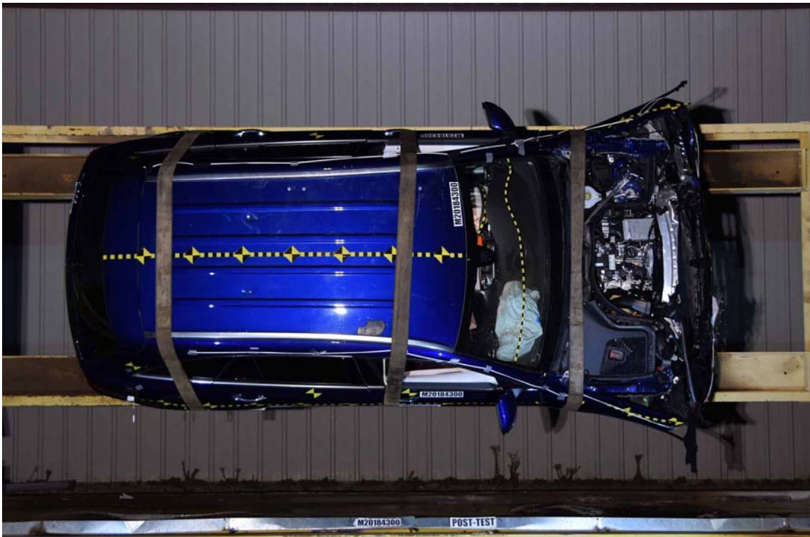
FIGURE 74. Vehicle at 90° on Static Rollover Device
