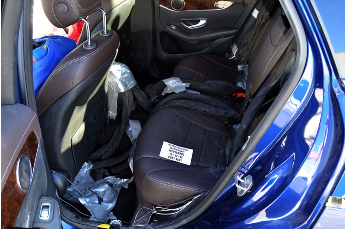
FIGURE 29. Post-Test Dummy Cable Routing
