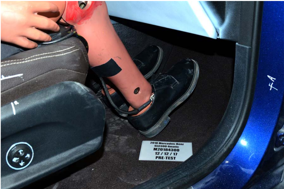
FIGURE 61. Pre-Test Passenger Dummy Feet
