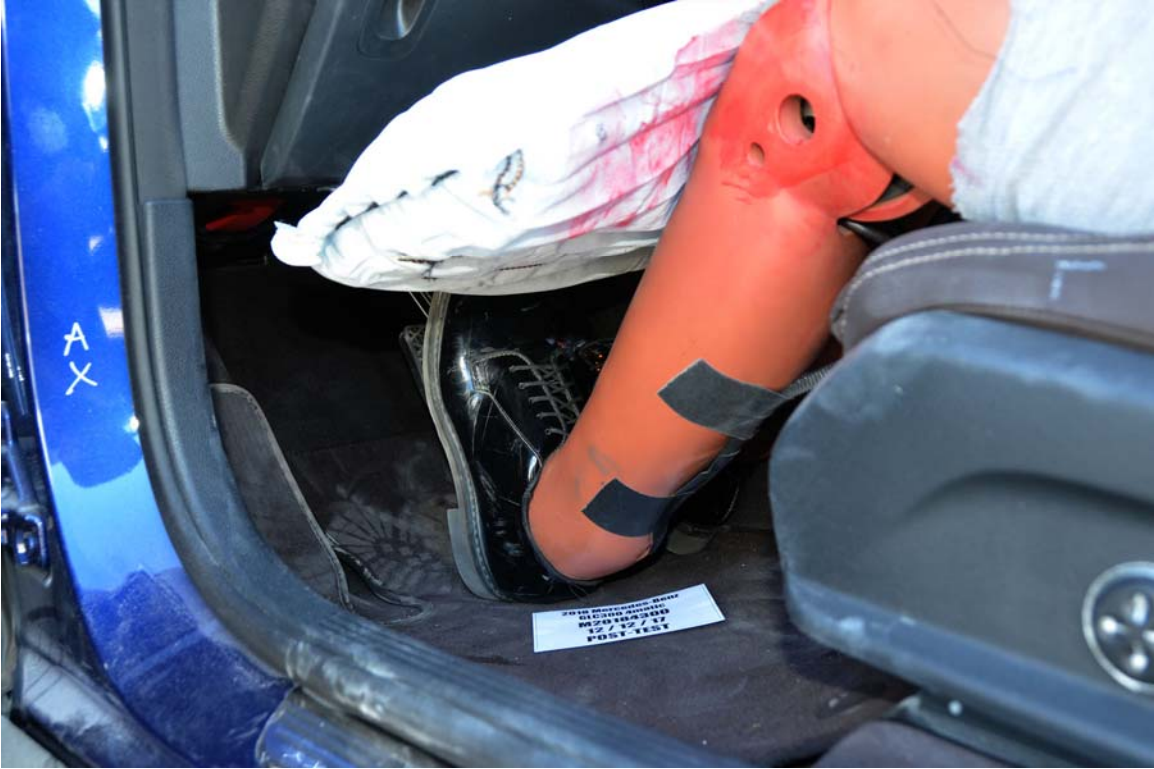
FIGURE 41. Post-Test Driver Dummy Feet
