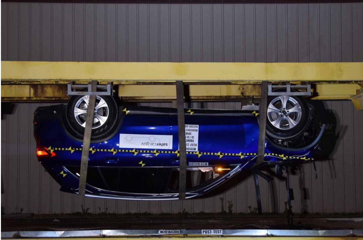
FIGURE 75. Vehicle at 180° on Static Rollover Device
