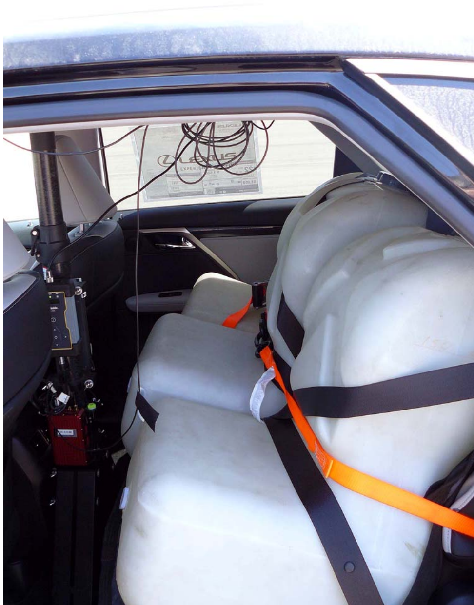
Figure A8. Ballast Condition
