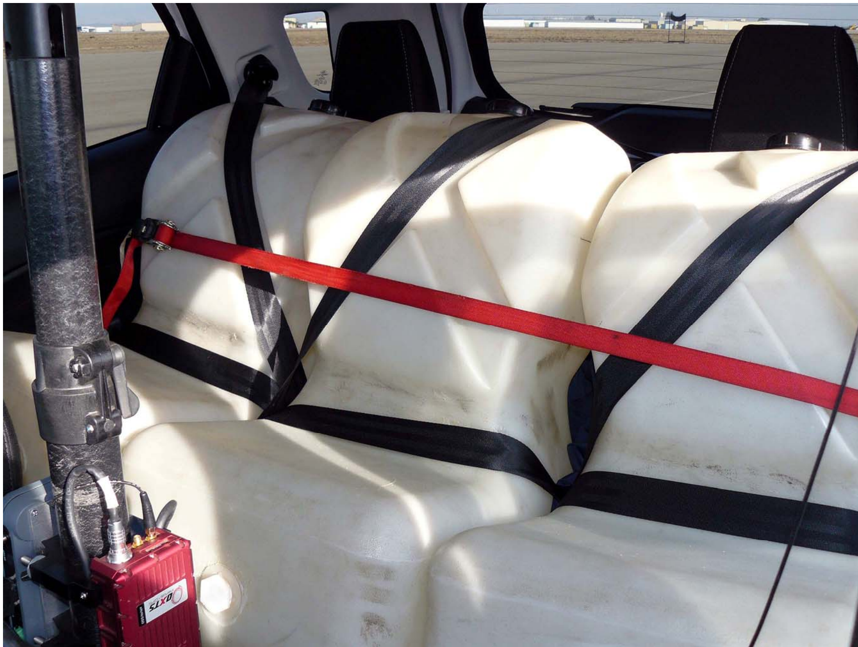
Figure A8. Ballast Condition
