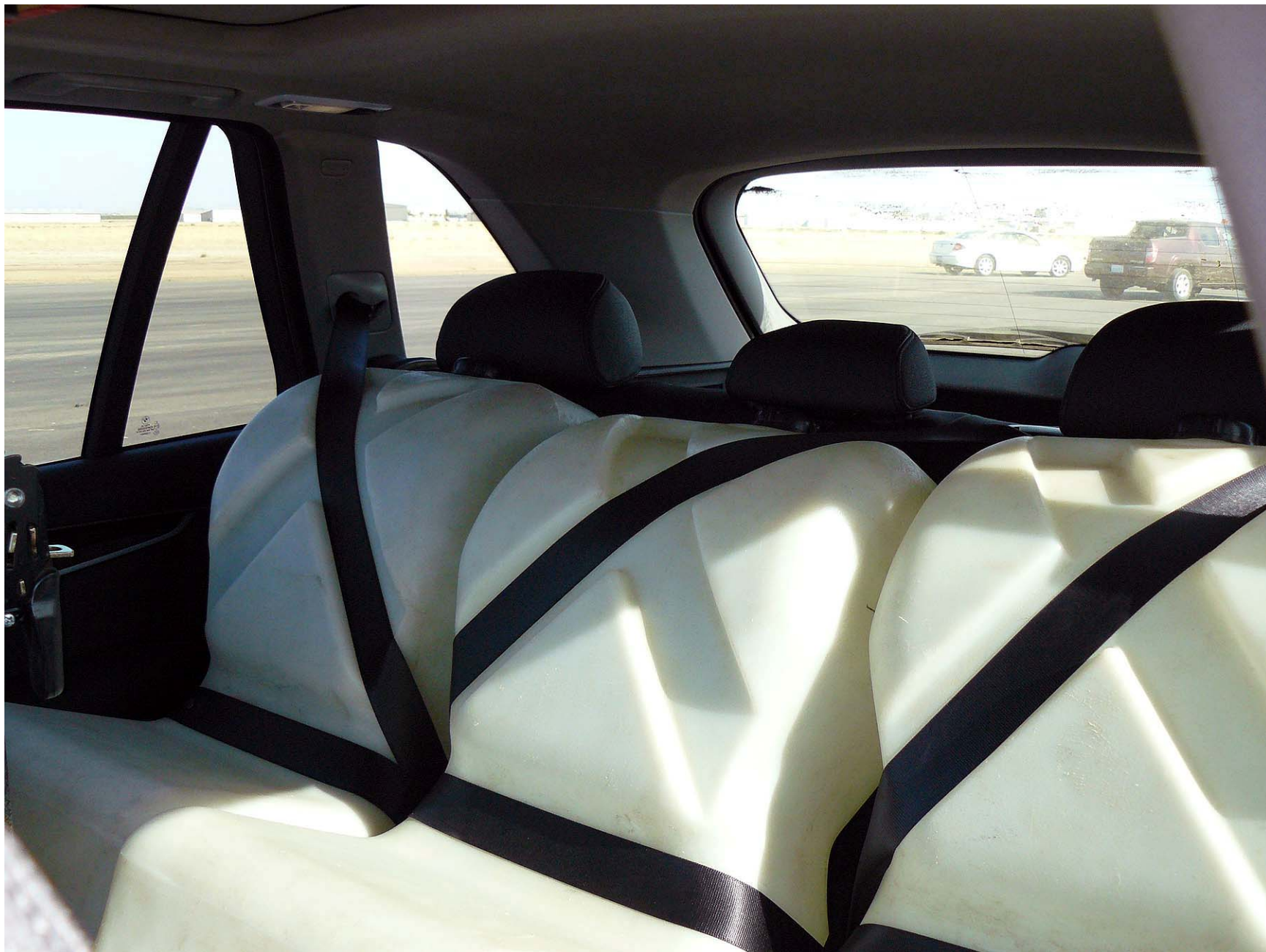
Figure A7. Ballast Condition
