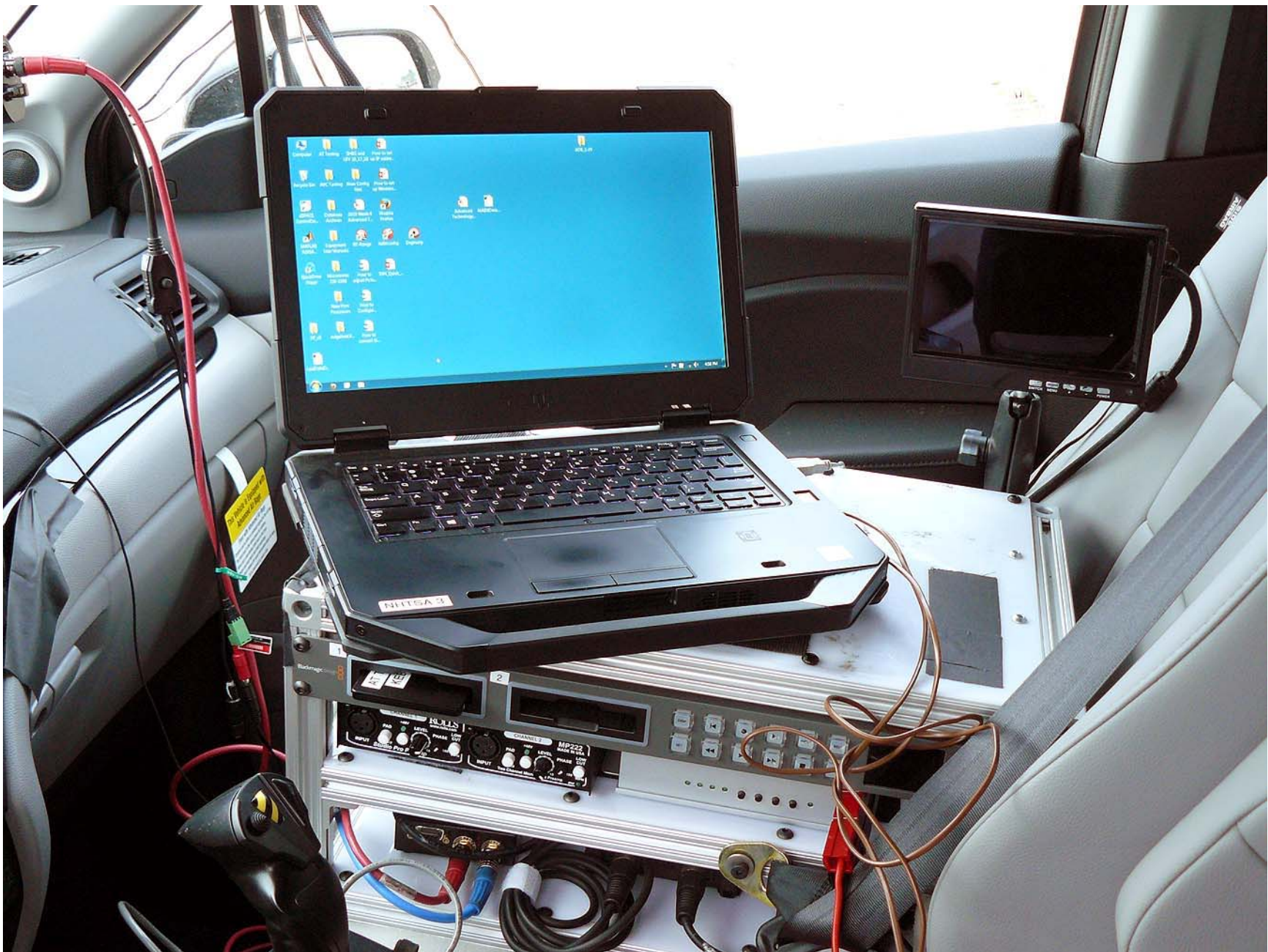
Figure A12. Computer Installed in Subject Vehicle
