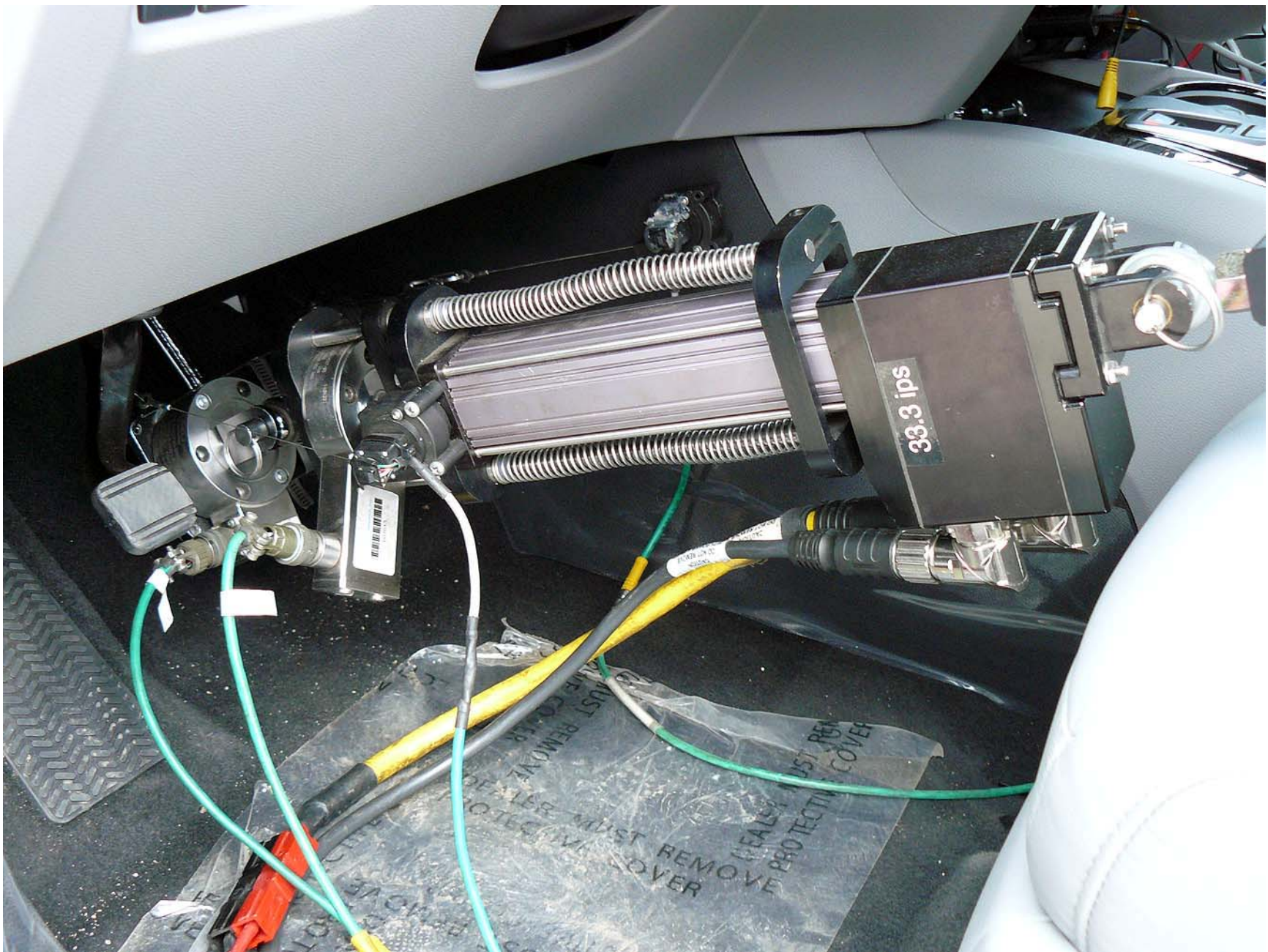
Figure A13. Brake Actuator Installed in Subject System
