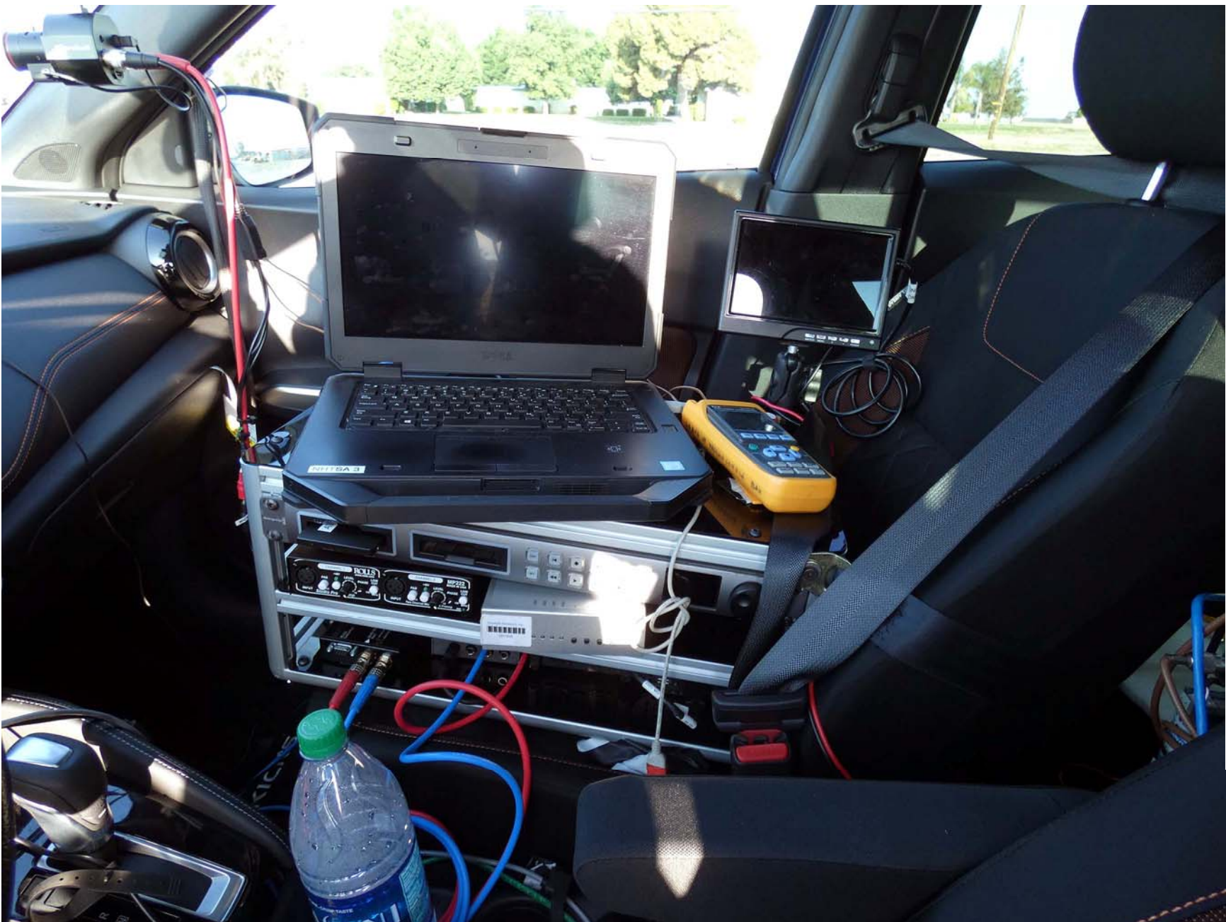
Figure A12. Computer Installed in Subject Vehicle
