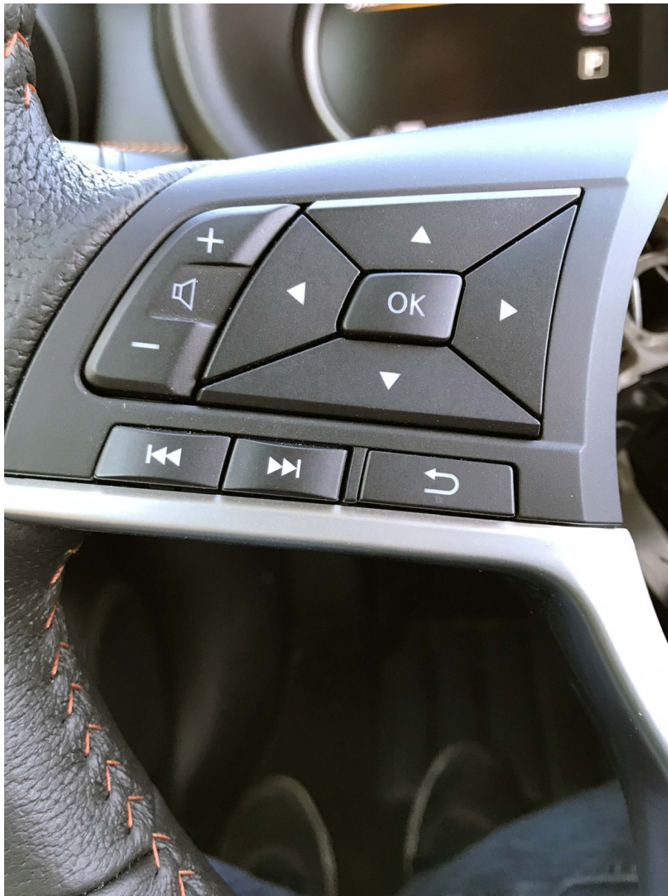
Figure A16. Steering Wheel Mounted Controls for Changing Parameters
