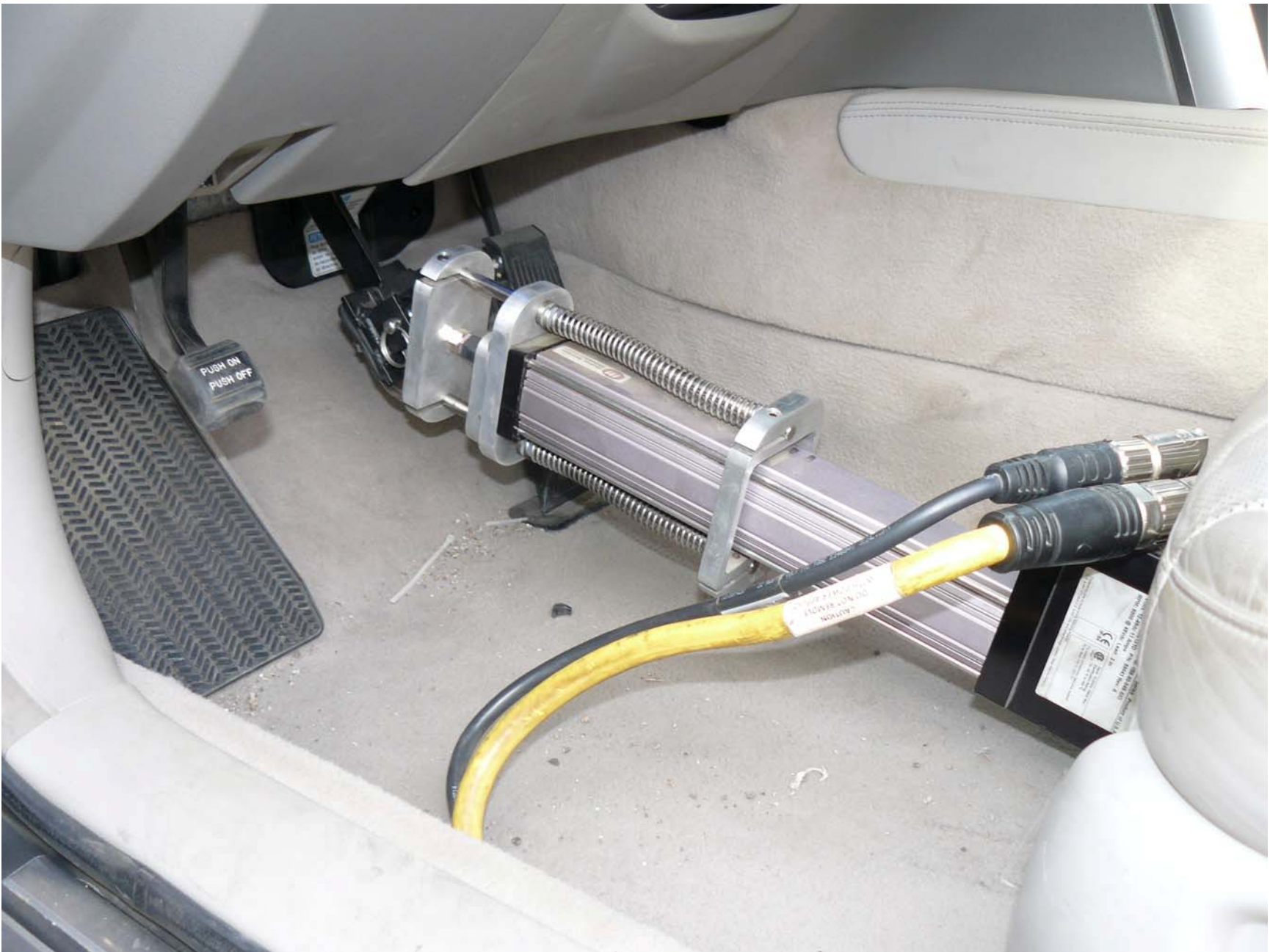
Figure A13. Brake Actuator Installed in POV System
