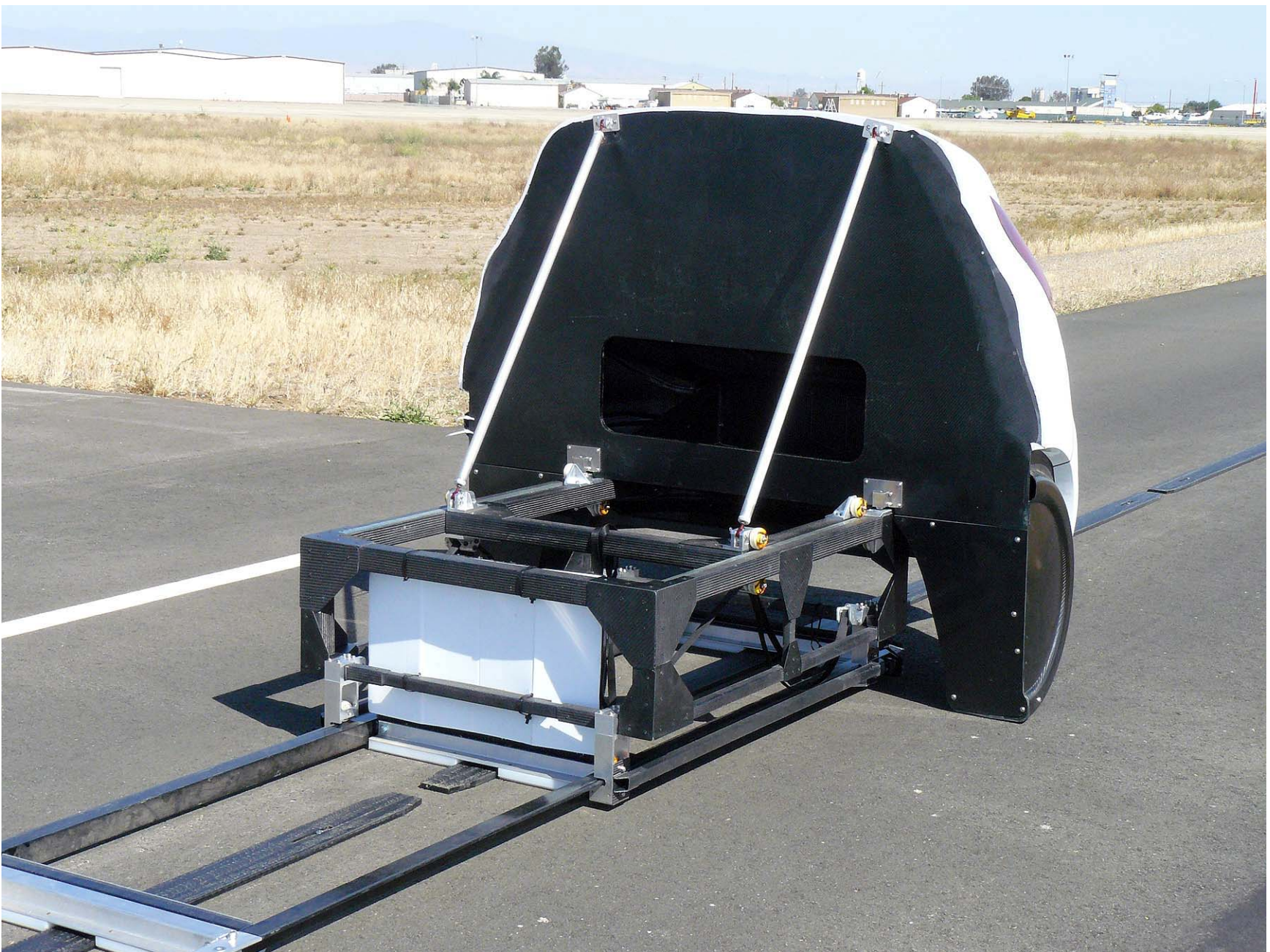
Figure A7. Load Frame/Slider of SSV
