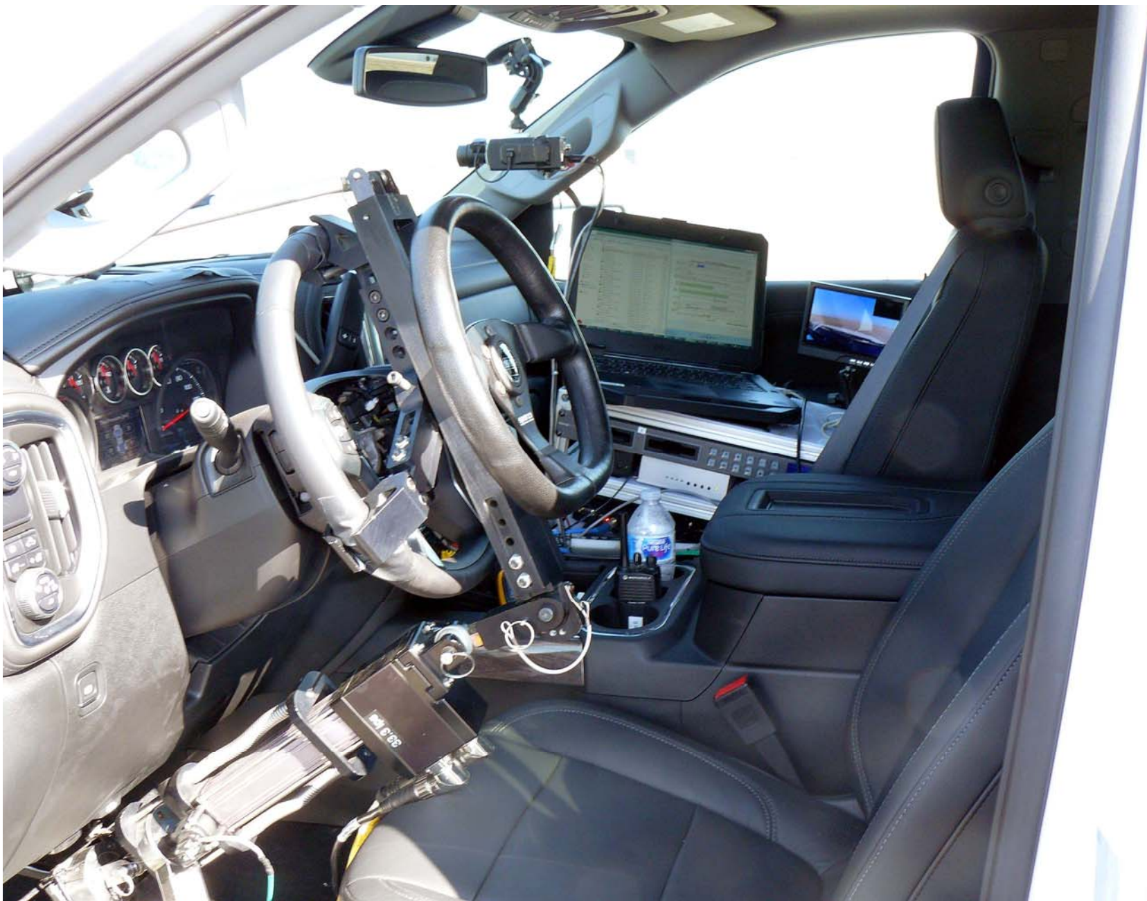
Figure A12. Computer and Brake Actuator Installed in Subject Vehicle
