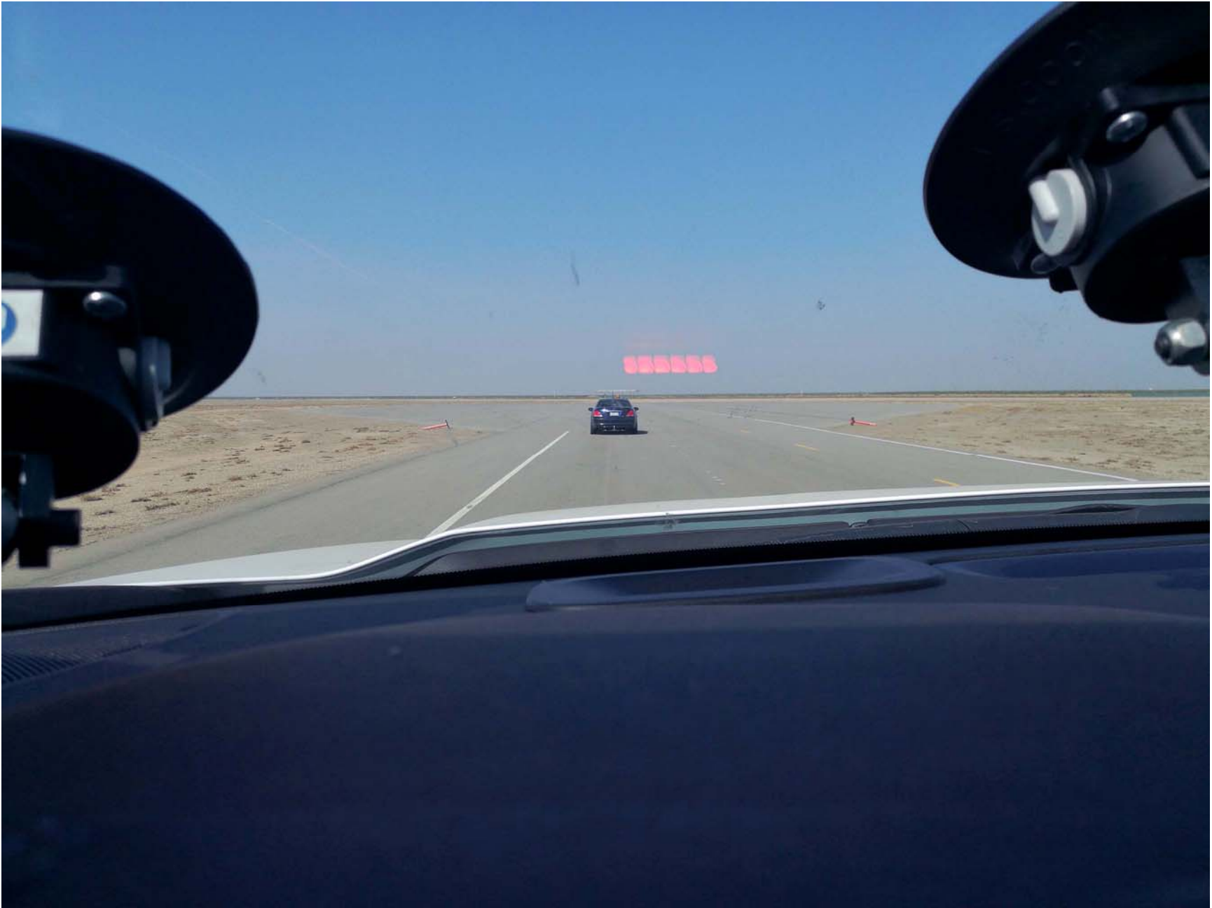
Figure A14. Heads-Up Visual AEB Alert
