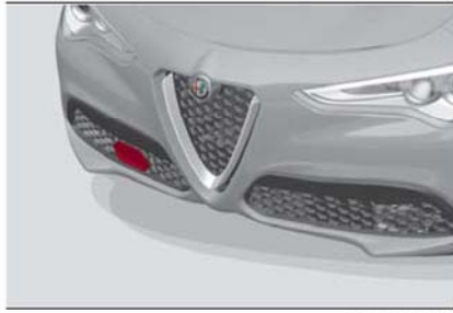
Front Bumper Radar Location
