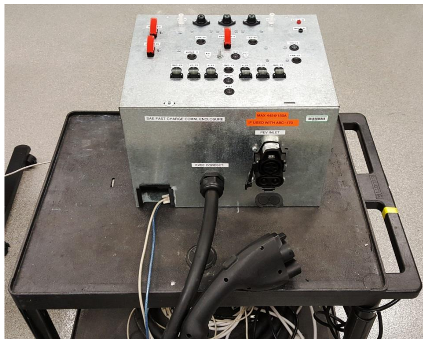
Figure 29: Prototype Breakout Box Constructed by ANL Engineers
