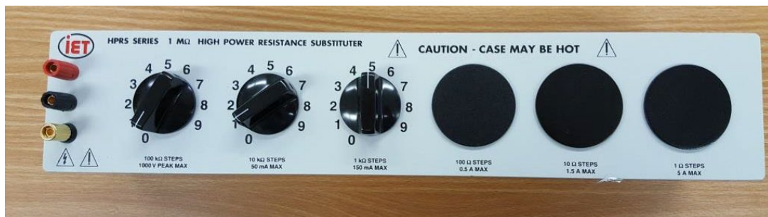
Figure 31: IET Labs HPRS Series High Power Resistance Decade Box
