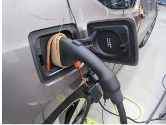
Figure 15: Example Heater Tape Installation
