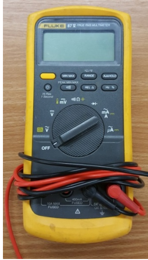
Figure 30: Fluke 87V Digital Multi-Meter
