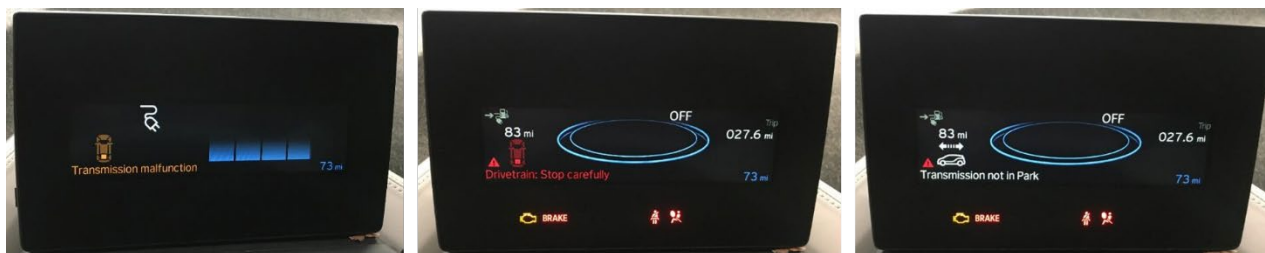
Figure 58: BMW i3 Fault Codes Displayed on Dash When Attempting to Charge With an Open Parking Pawl
