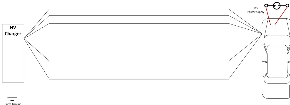
Figure 9: 12V System Overvoltage Test - 12V Power Supply Connection
