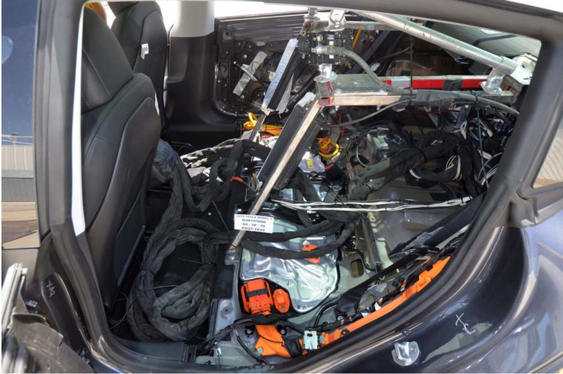
FIGURE 29. Post-Test Dummy Cable Routing
