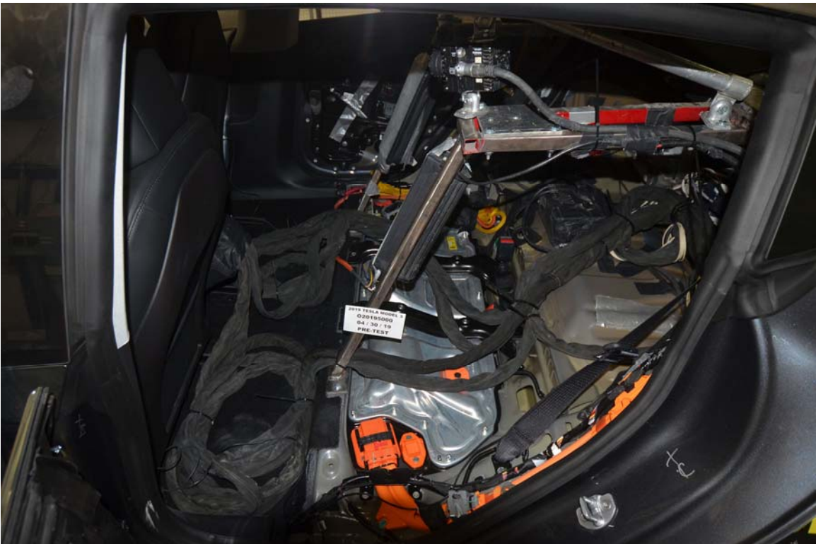
FIGURE 28. Pre-Test Dummy Cable Routing
