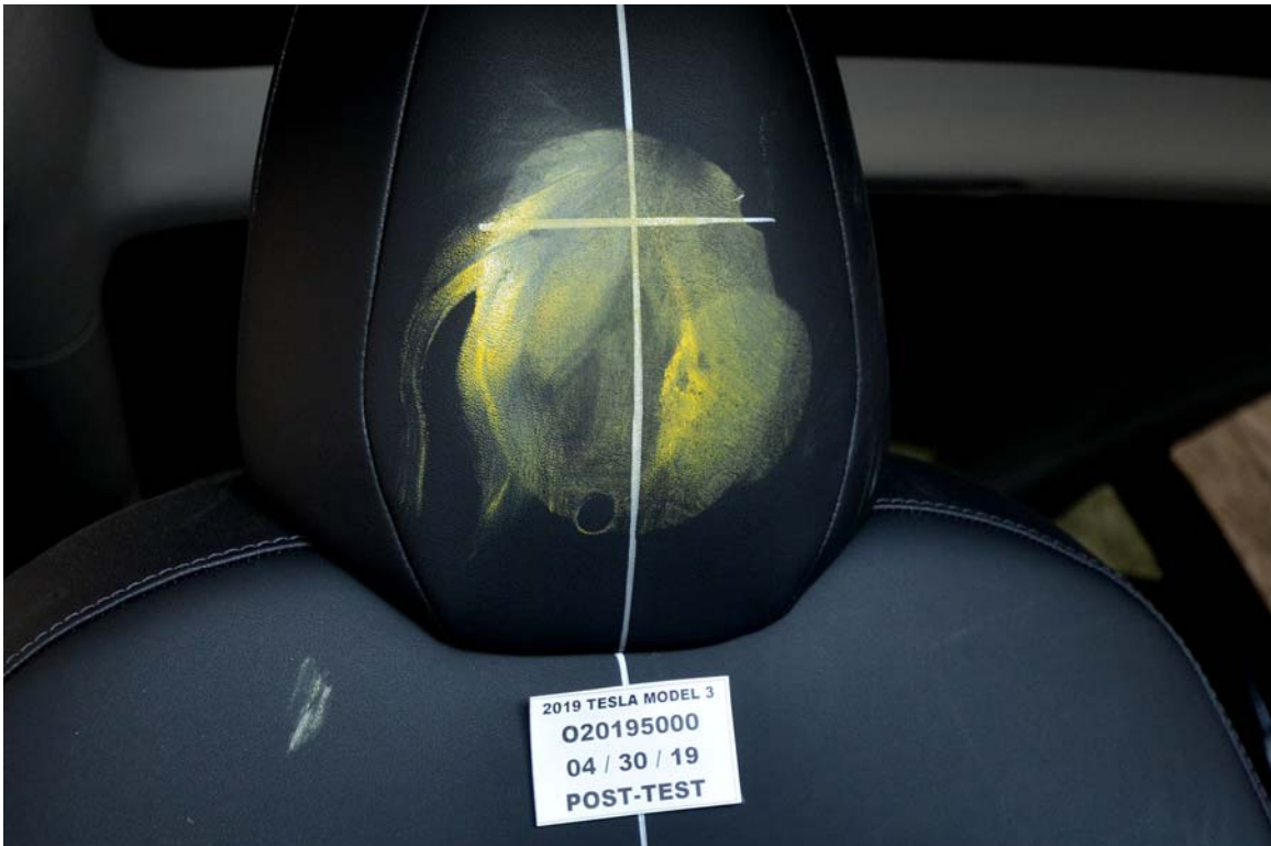
FIGURE 69. Post-Test Passenger Dummy Contact with Headrest
