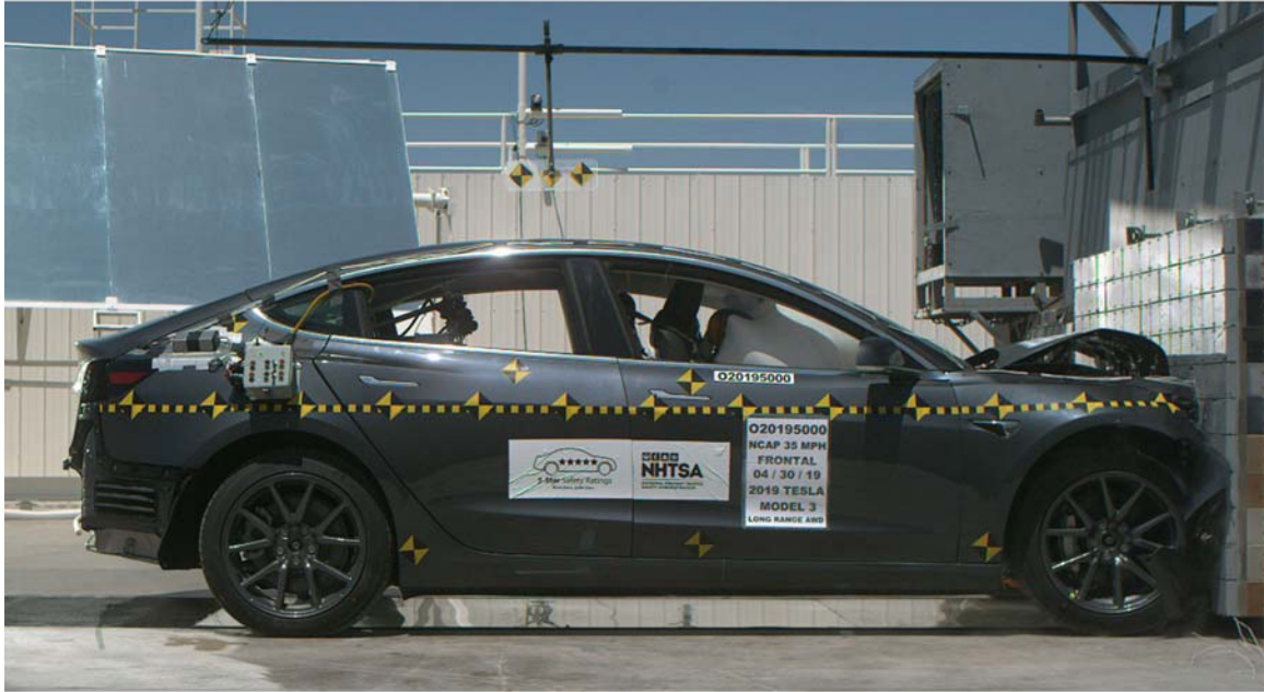
FIGURE 78. 2019 Tesla Model 3 Long Range AWD Frontal Impact Event
