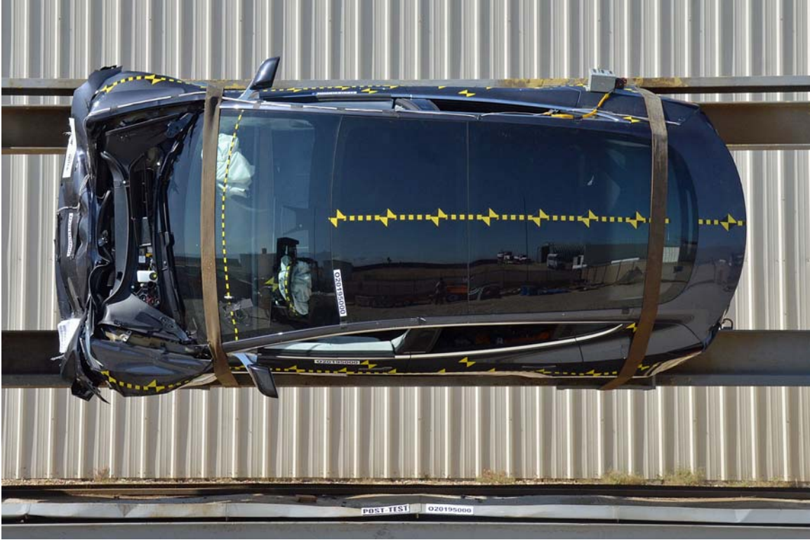
FIGURE 74. Vehicle at 90° on Static Rollover Device
