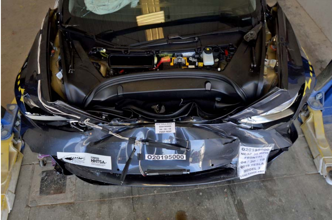
FIGURE 21. Post-Test Front Storage Compartment View
