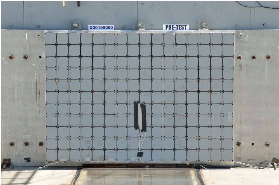
FIGURE 2. Pre-Test Load Cell Wall
