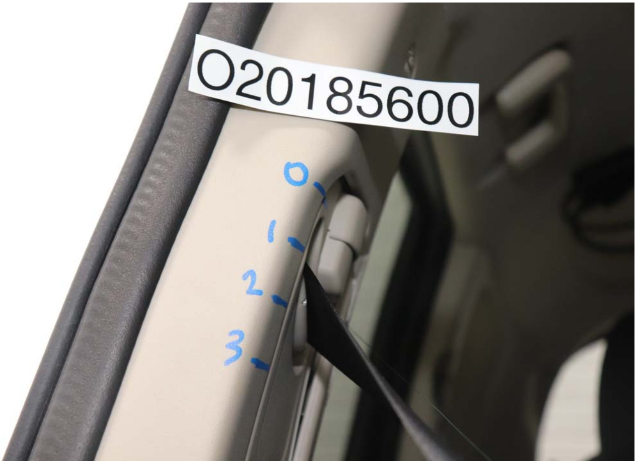
Photo No. 059 - Pre-Test View of Belt Anchorage for Passenger Dummy
