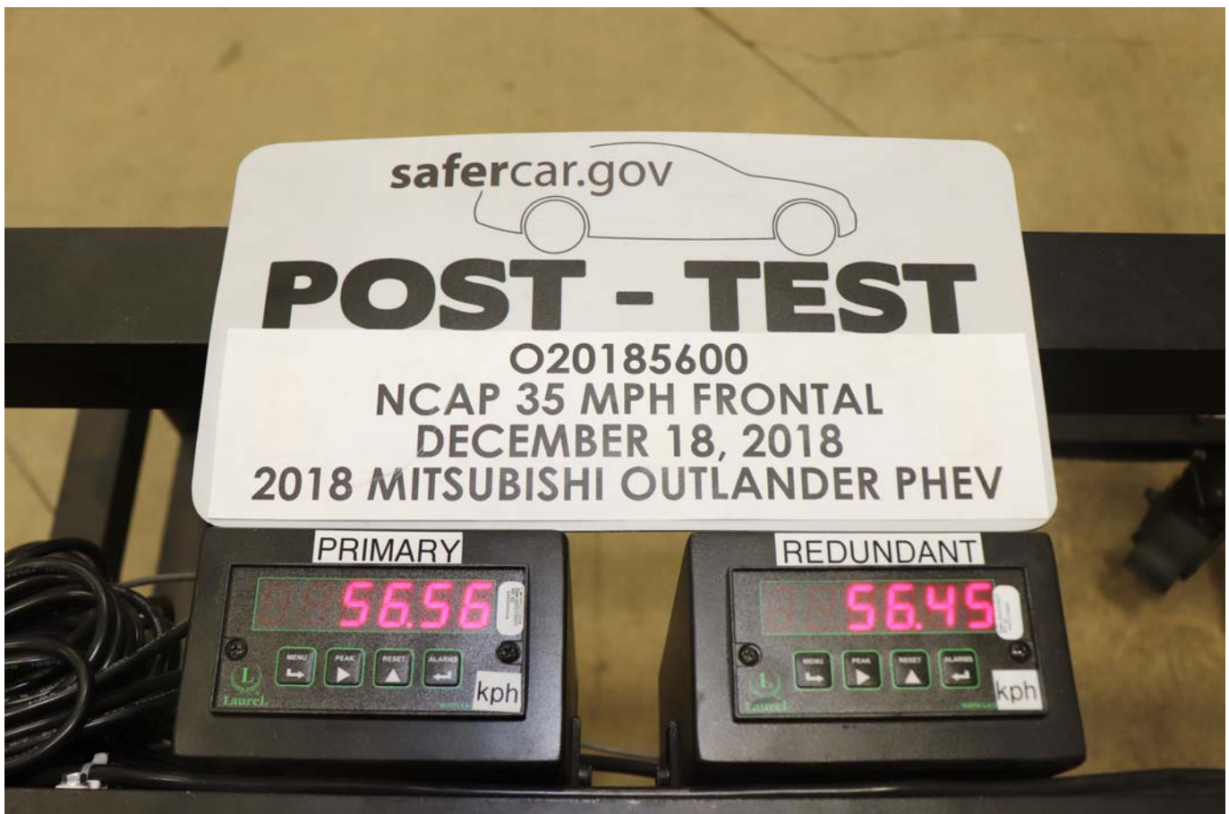
Photo No. 072 - Post-Test Speed Trap Read-Out
