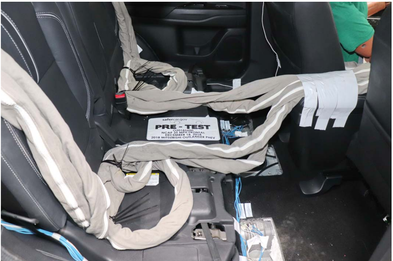
Photo No. 028 - Pre-Test Dummy Cable Routing
