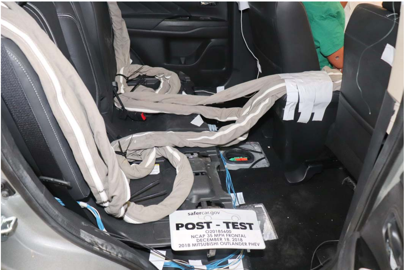
Photo No. 029 - Post-Test Dummy Cable Routing
