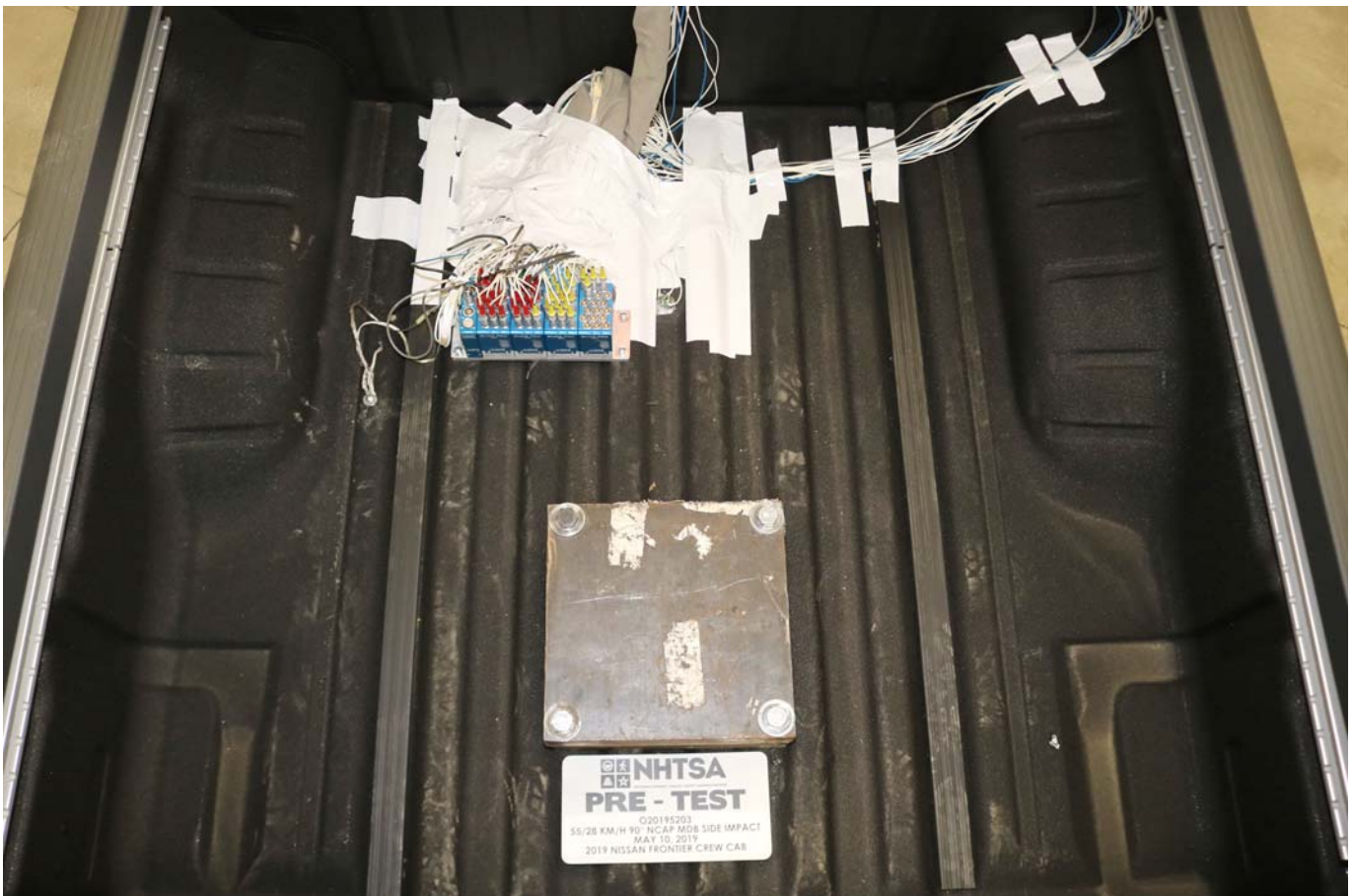
Photo No. 094 - Pre-Test Ballast View
