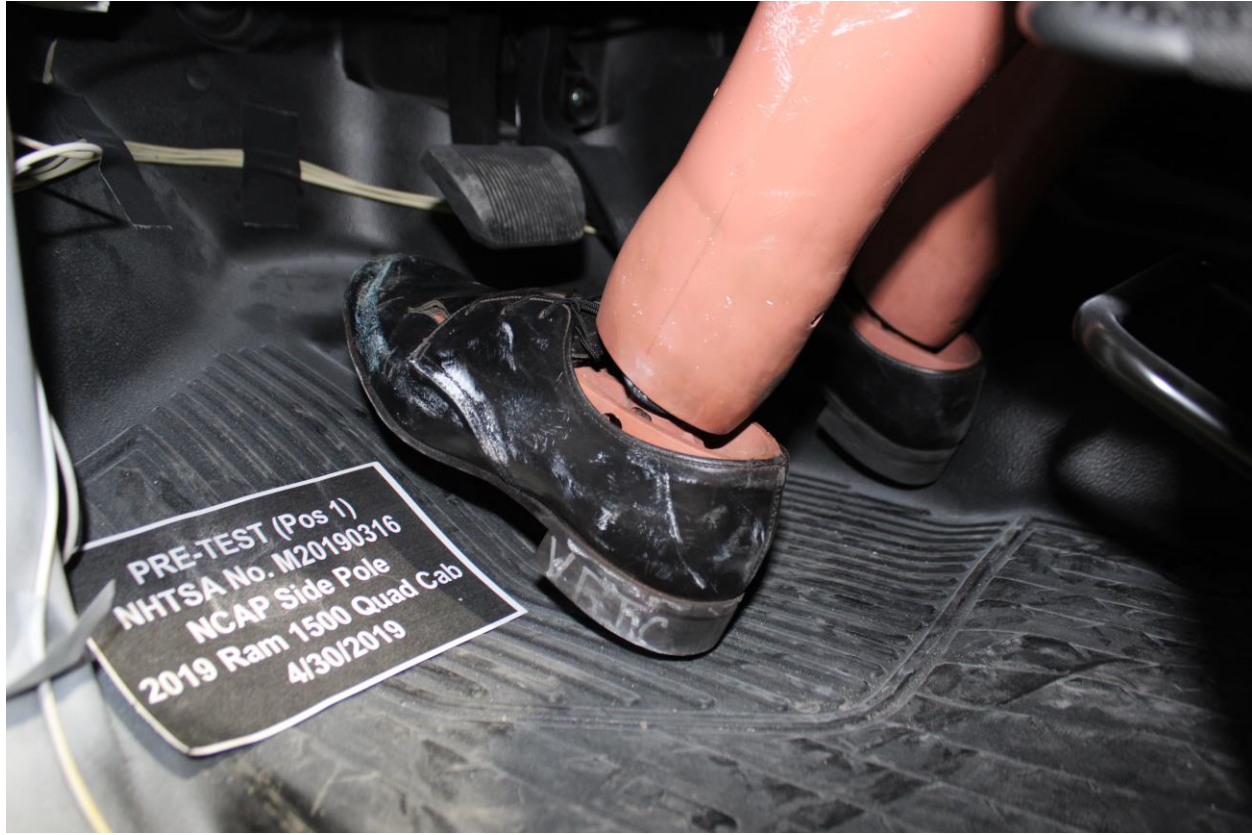
Figure A-32: Pre-Test Placement of Dummy's Feet
