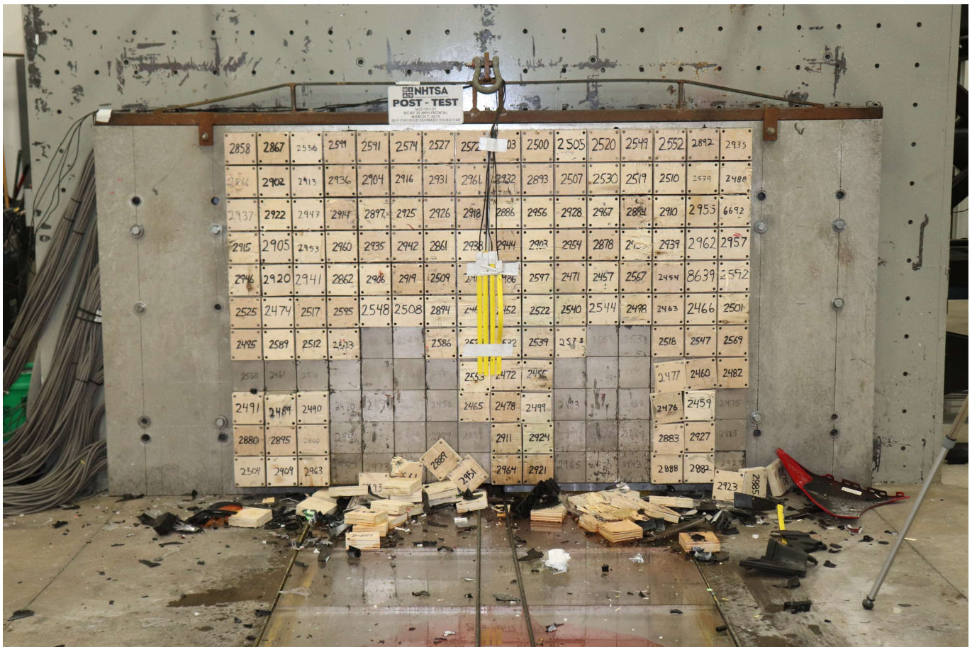
Photo No. 003 - Post-Test Load Cell Wall
