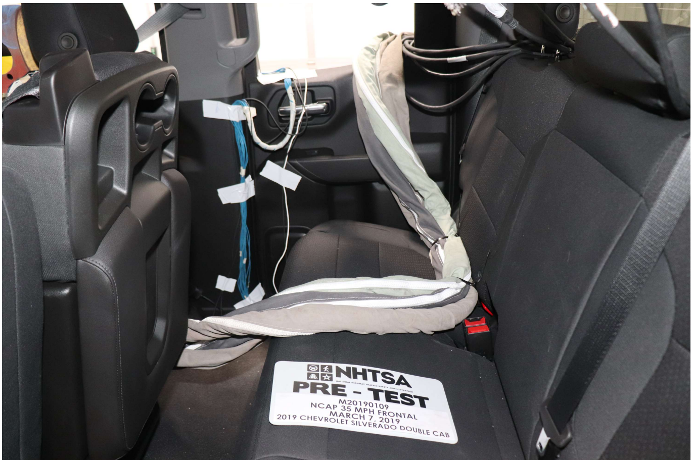
Photo No. 028 - Pre-Test Dummy Cable Routing
