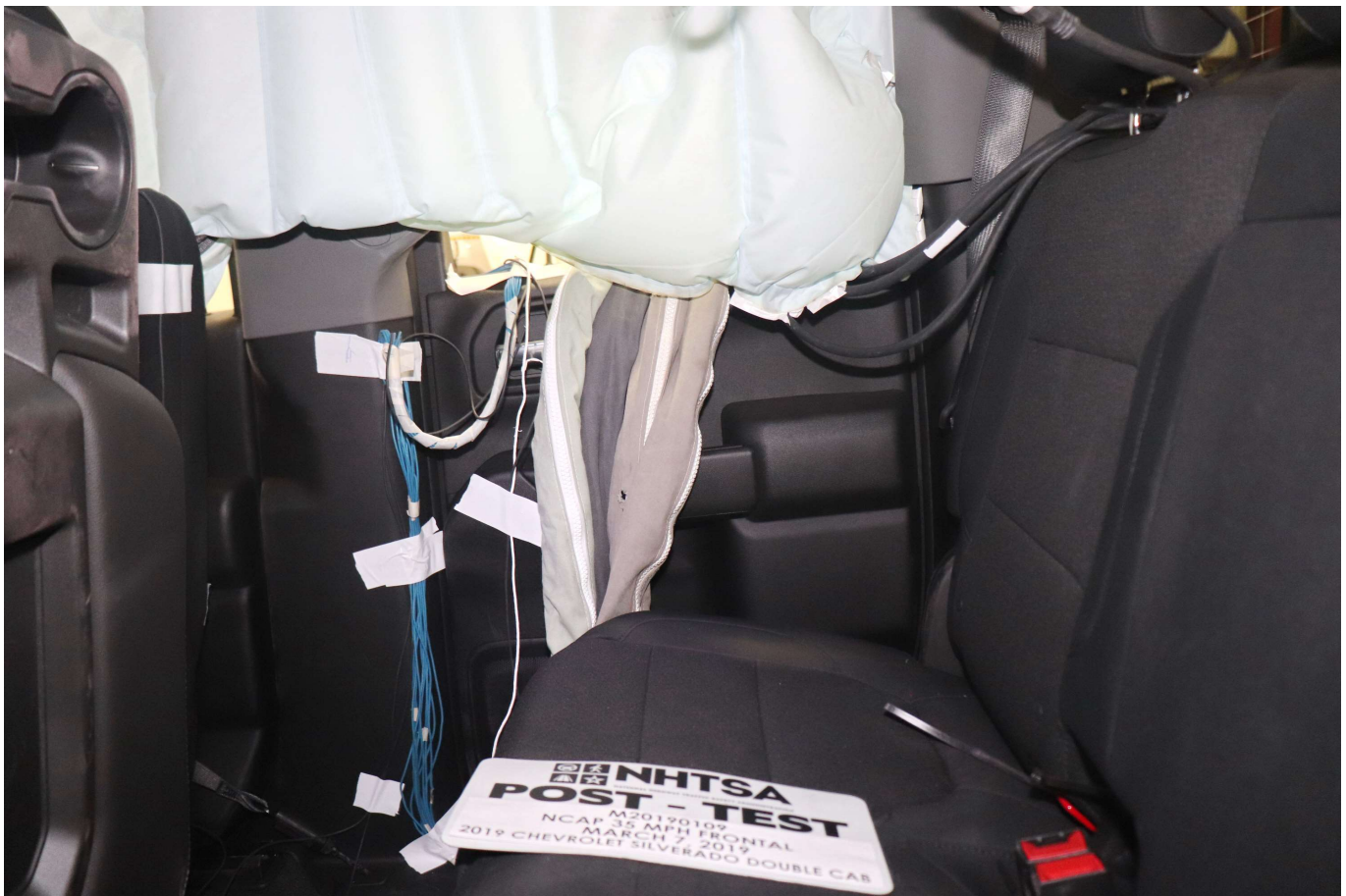
Photo No. 029 - Post-Test Dummy Cable Routing
