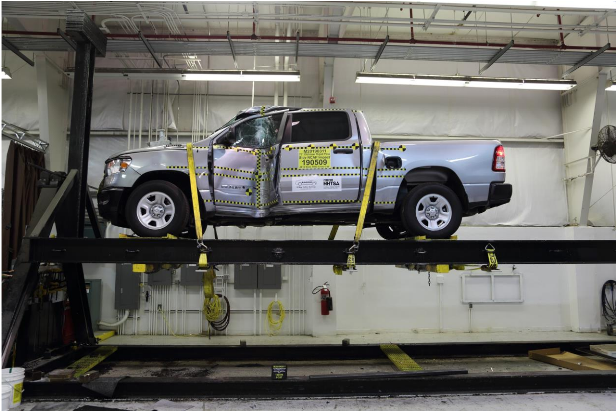
No. 067 FMVSS No. 301 Static Rollover 360 Degrees
