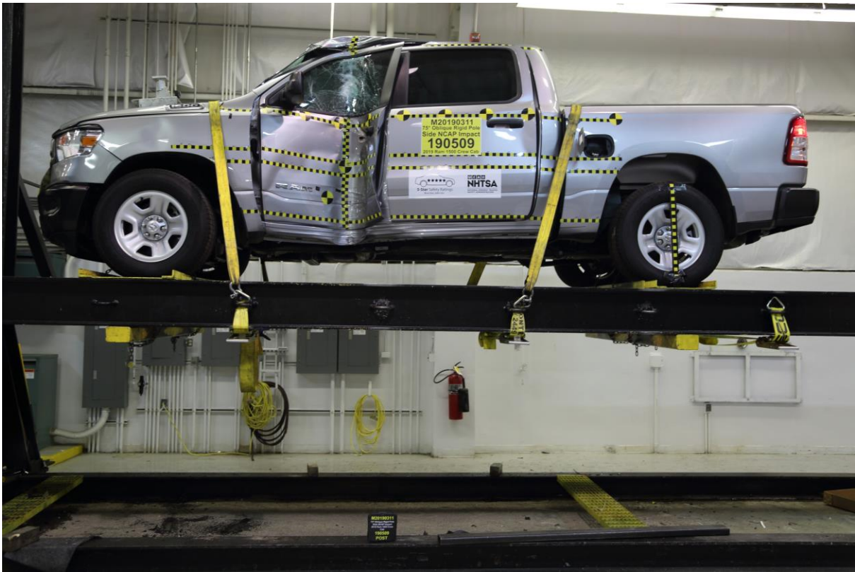
No. 063 FMVSS No. 301 Static Rollover 0 Degrees
