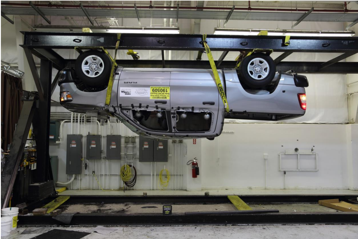
No. 065 FMVSS No. 301 Static Rollover 180 Degrees
