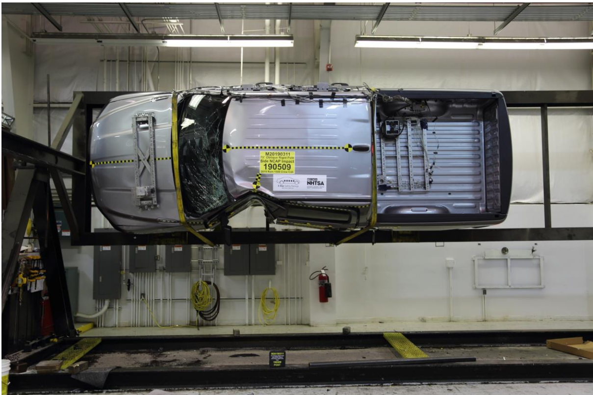
No. 064 FMVSS No. 301 Static Rollover 90 Degrees
