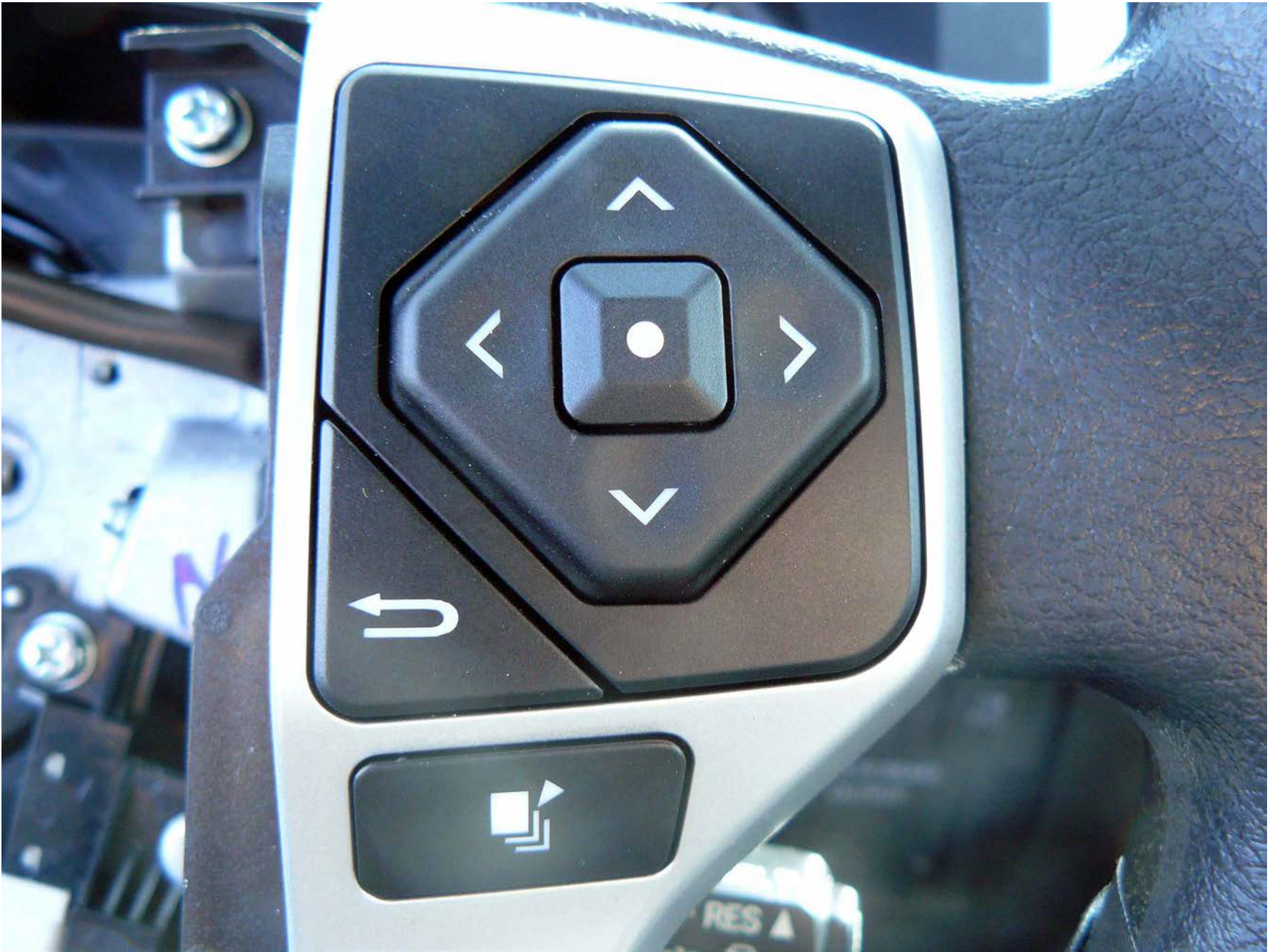
Figure A16. Steering Wheel Mounted Controls for AEB/FCW System Settings
