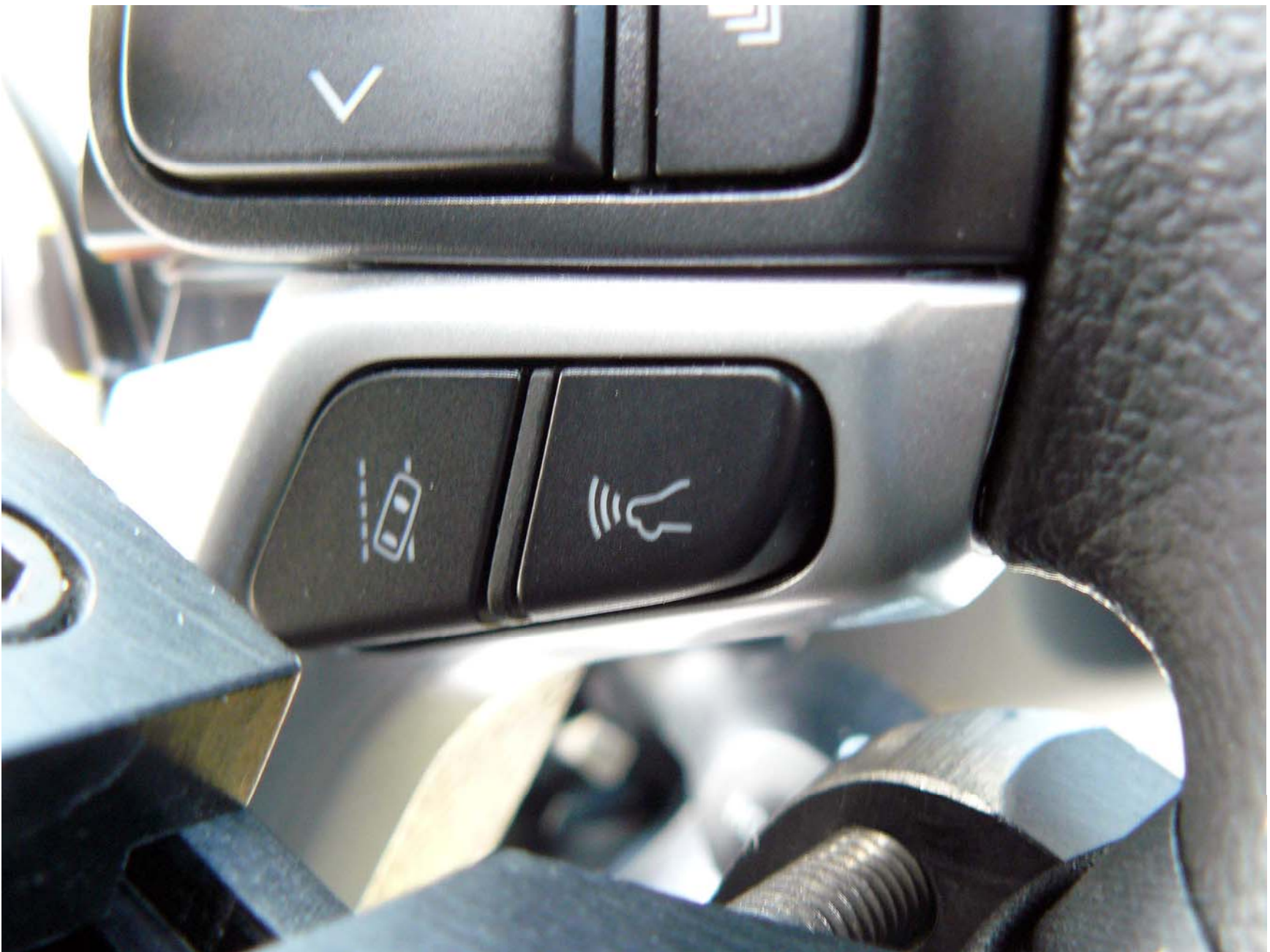
Figure A19. Steering Wheel Mounted Control Buttons for Setting Range
