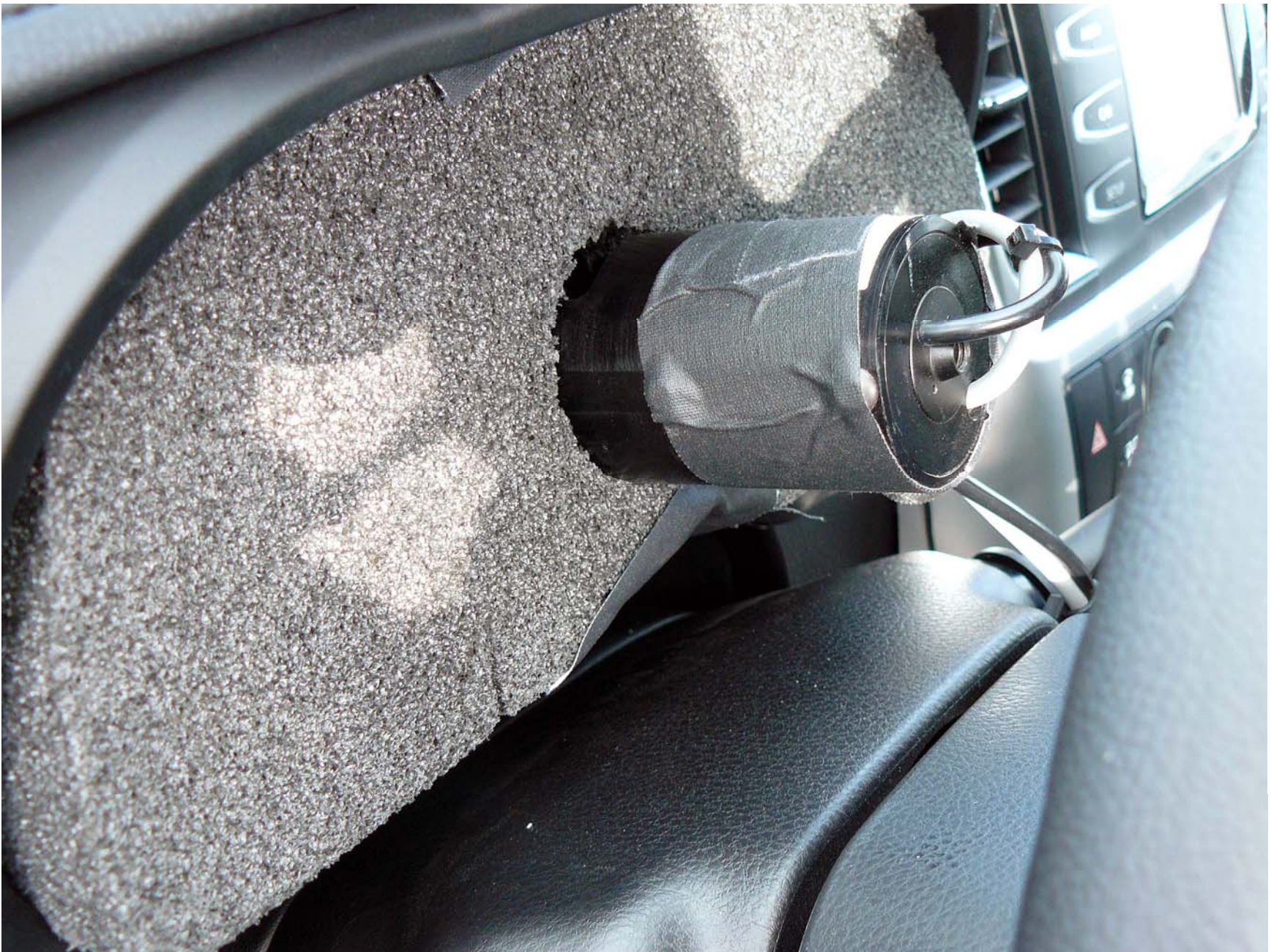
Figure A12. Sensor for Detecting Visual Alerts
