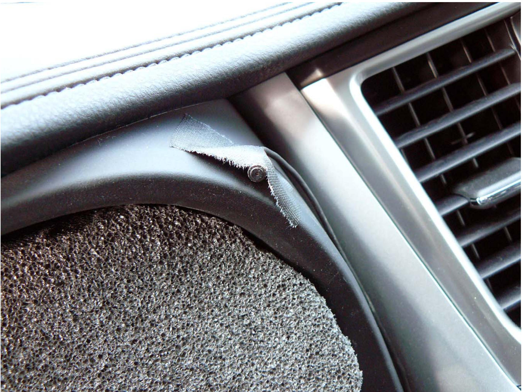
Figure A11. Sensor for Detecting Auditory Alerts
