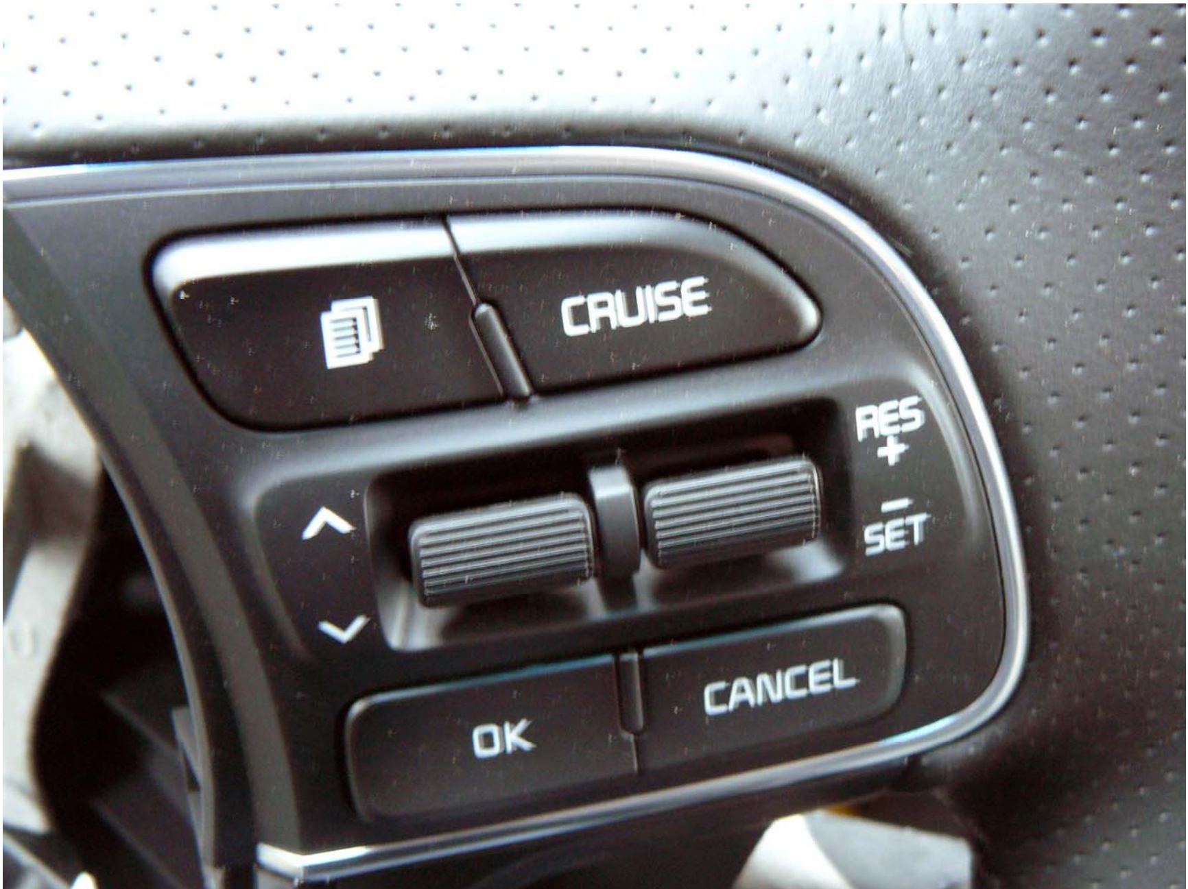
Figure A16. Steering Wheel Mounted Control Buttons for Changing Parameters
