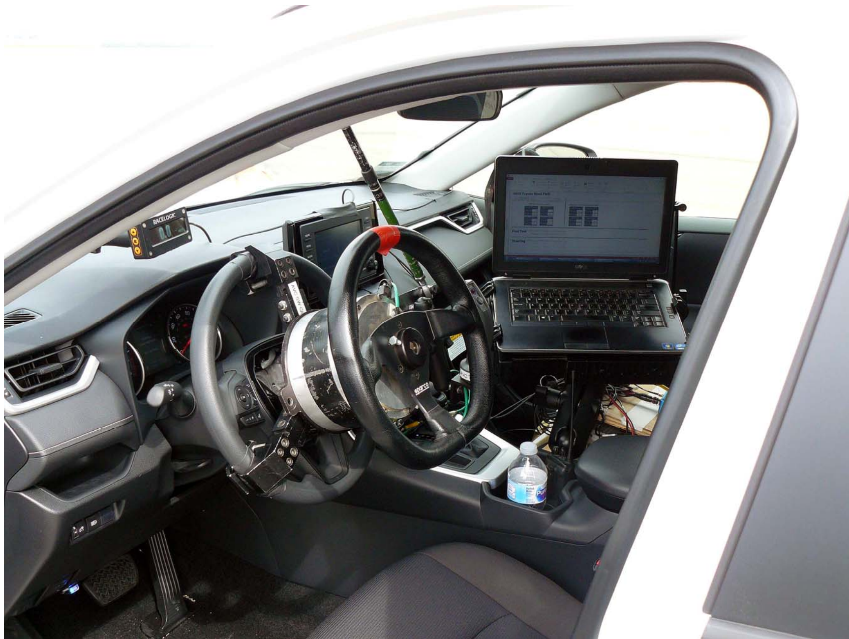
Figure A9. Steering Controller and Computer
