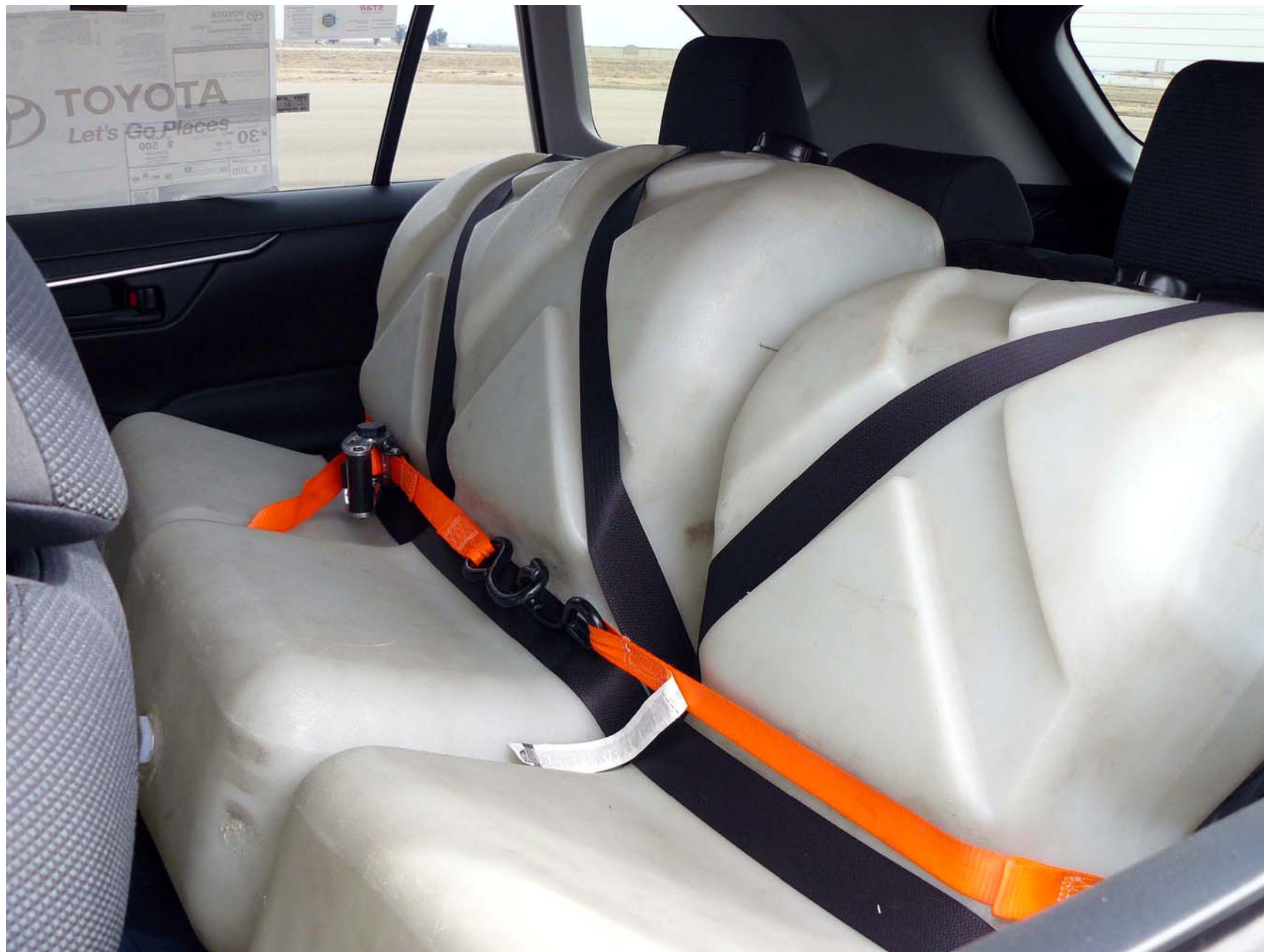
Figure A10. Ballast Condition
