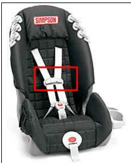
Retainer clip with 5-point harness
