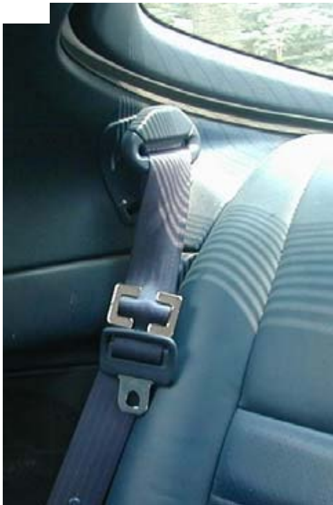
Locking clip incorrectly placed on belt webbing
