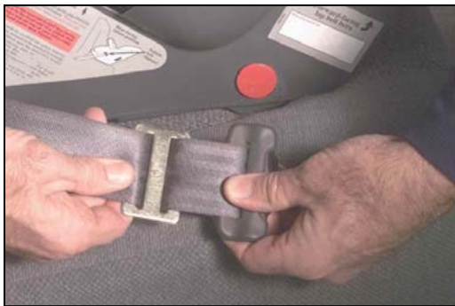
ng clip no more than 1 inch from latch plate
