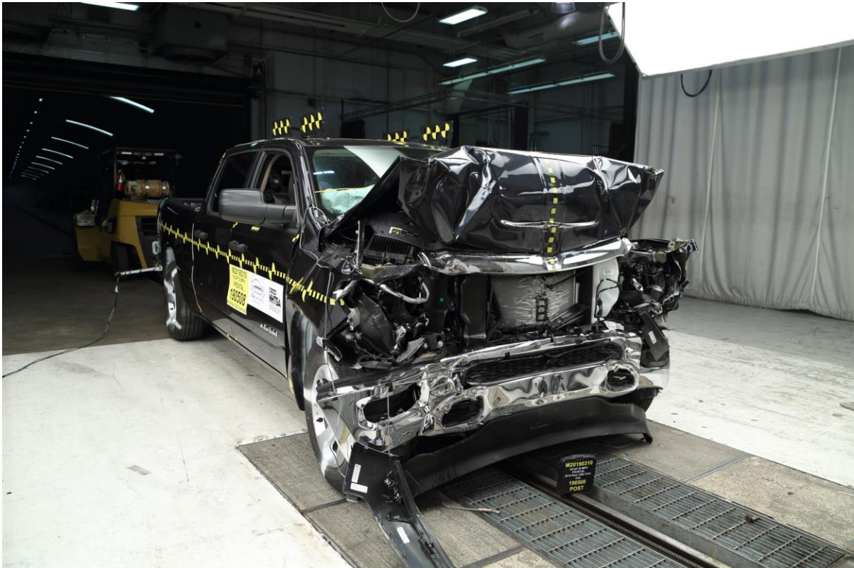
015 Post-Test Right Front 3-4 View
