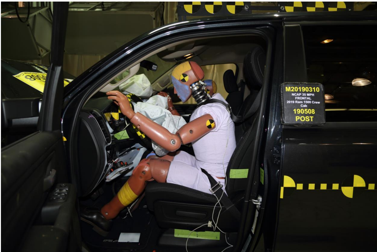
035 Post-Test Driver Dummy and Vehicle Interior View
