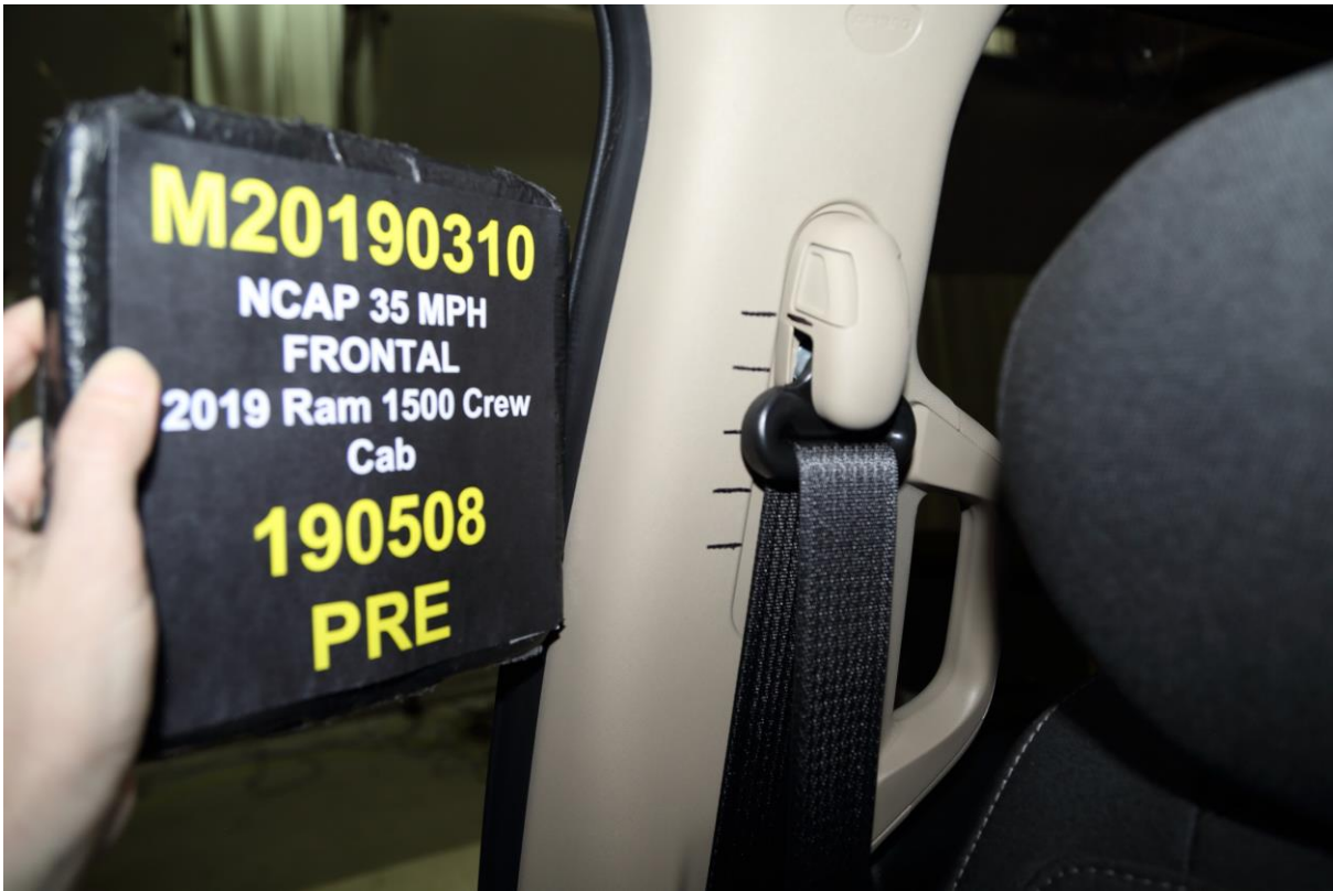
061 Pre-Test View of Belt Anchorage for Passenger Dummy
