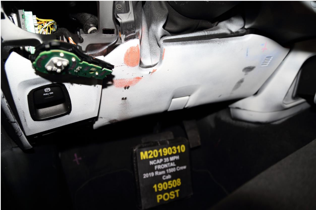
045 Post-Test Driver's Side Knee Bolster
