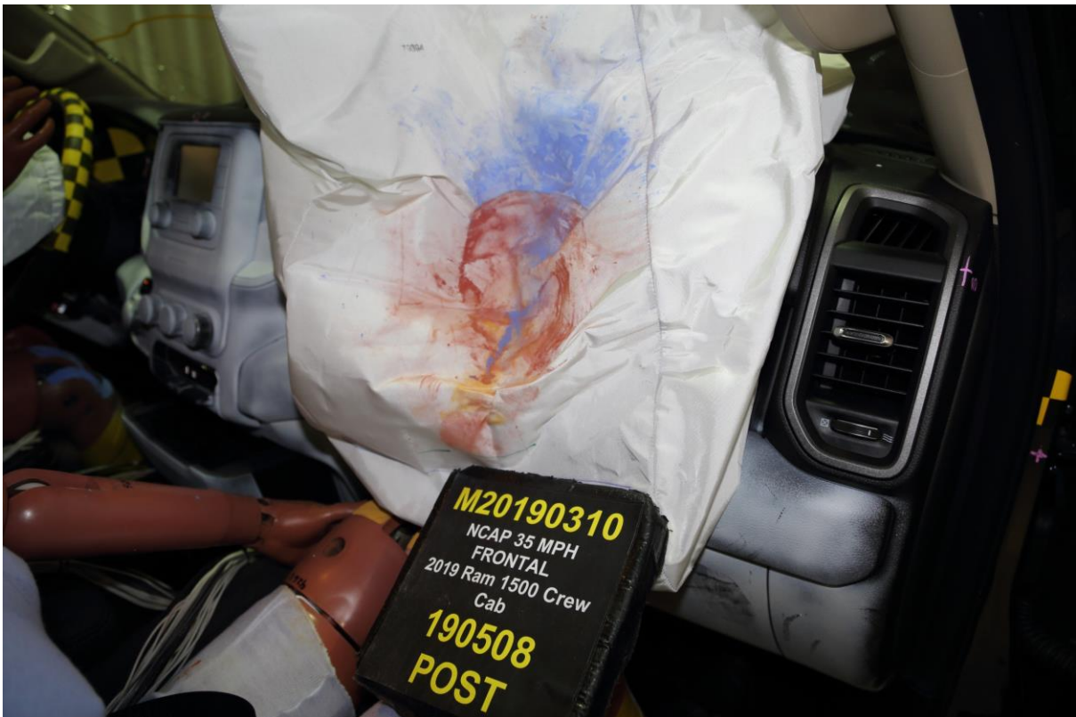
072 Post-Test Passenger Dummy Contact with Airbag
