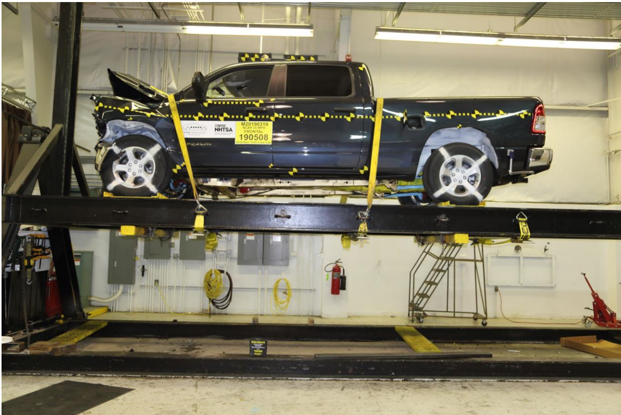
077 Vehicle at 0° on Static Rollover Device
