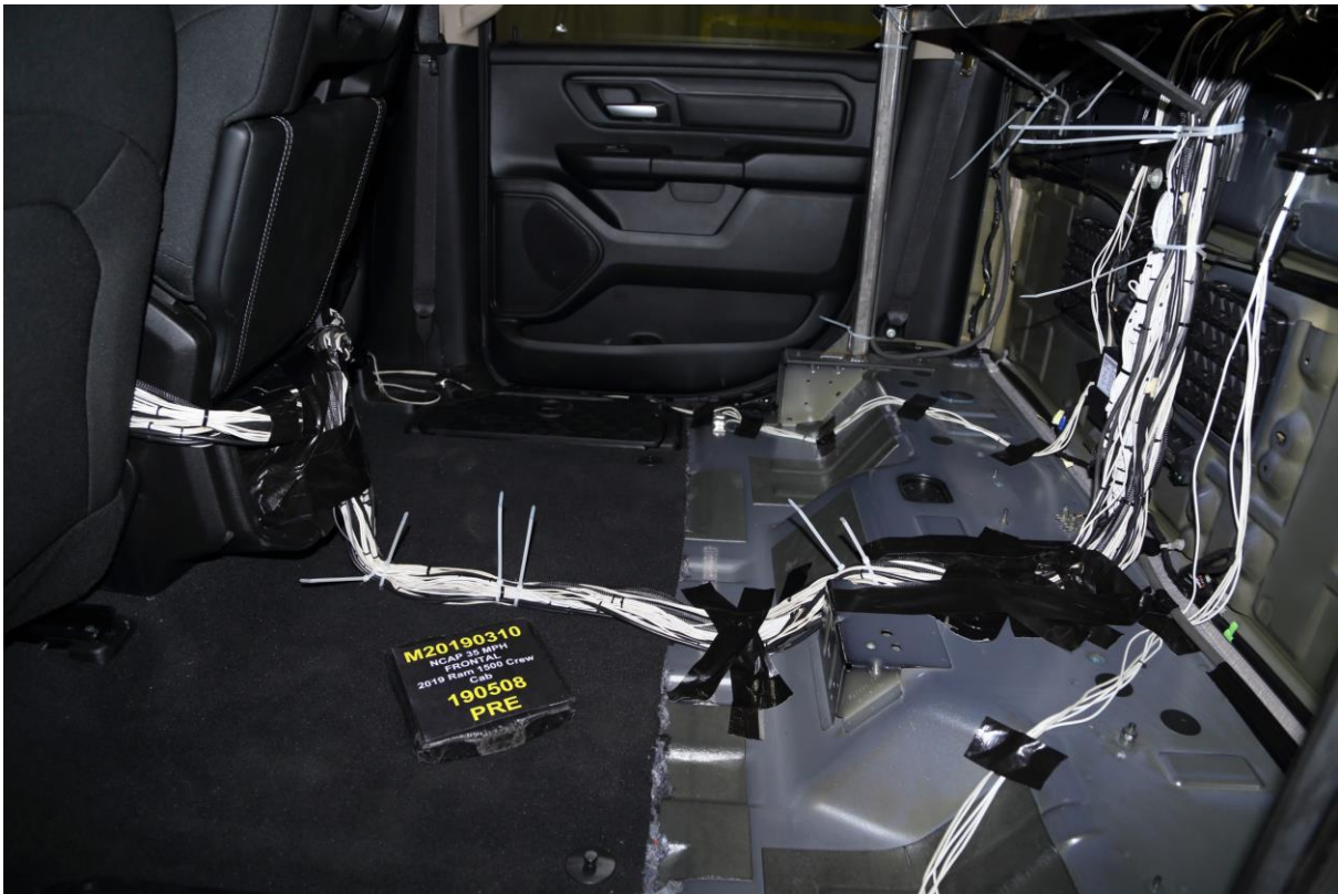
028 Pre-Test Dummy Cable Routing
