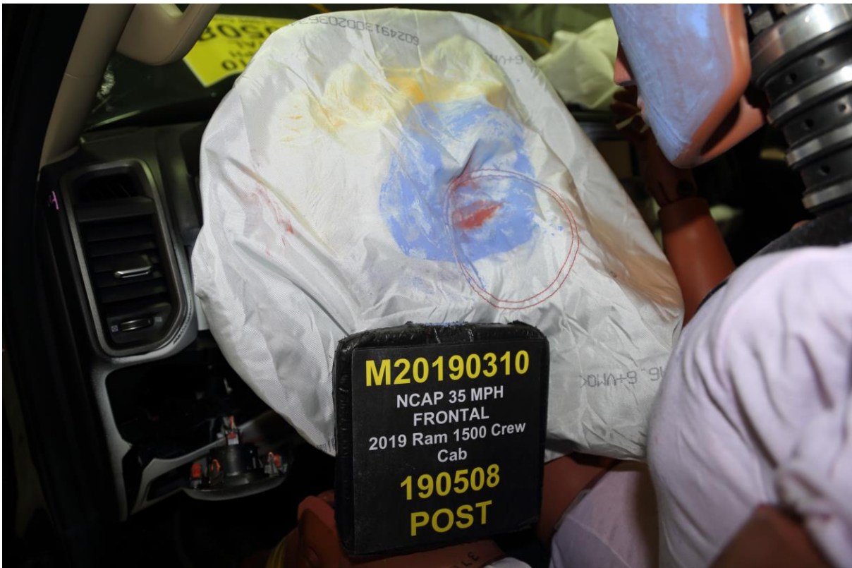
049 Post-Test Driver Dummy Contact with Airbag
