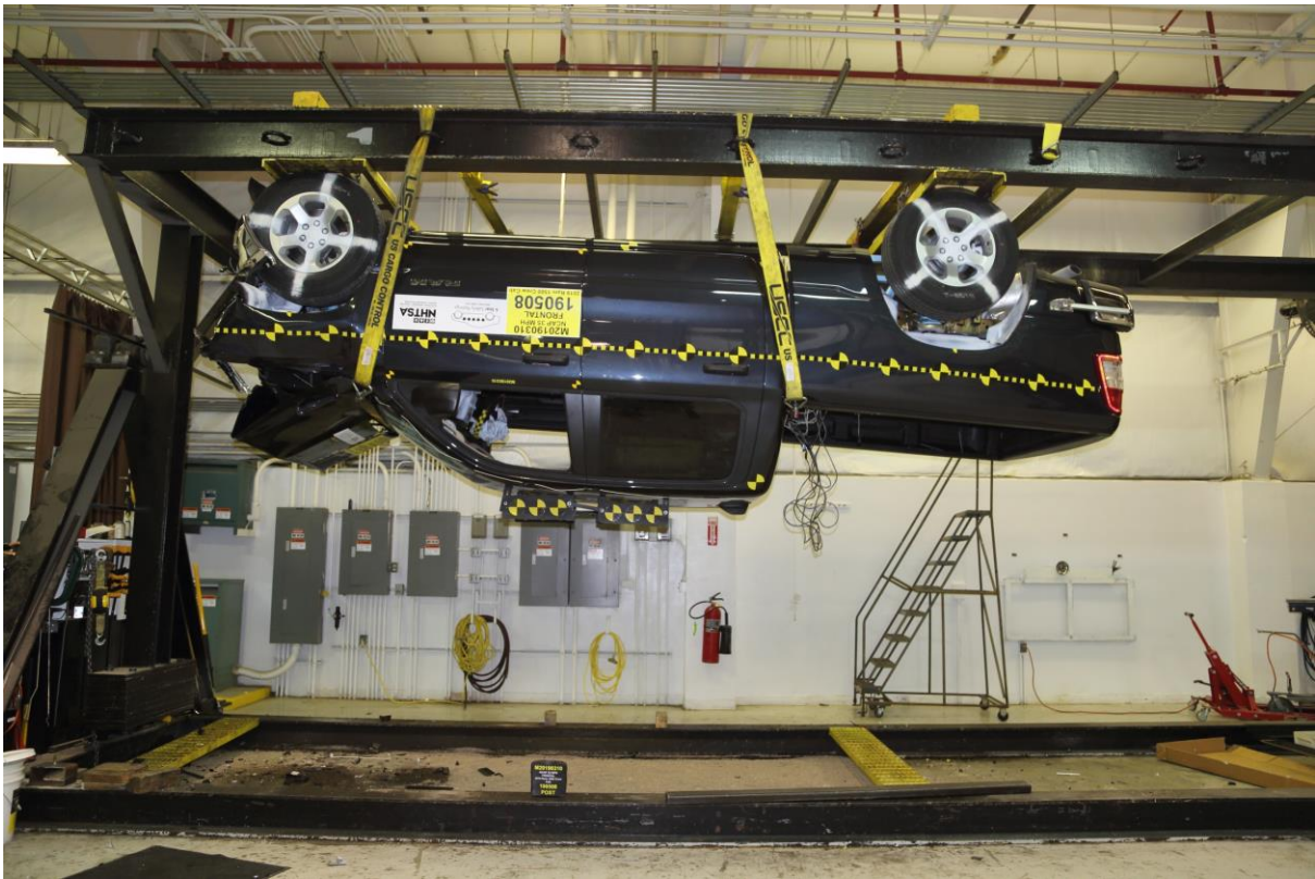
079 Vehicle at 180° on Static Rollover Device
