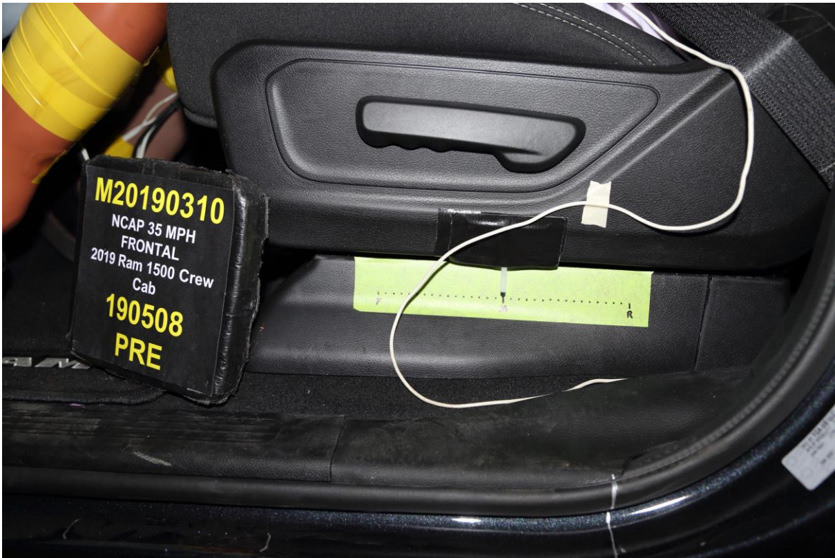
036 Pre-Test Driver's Seat Fore-Aft Markings
