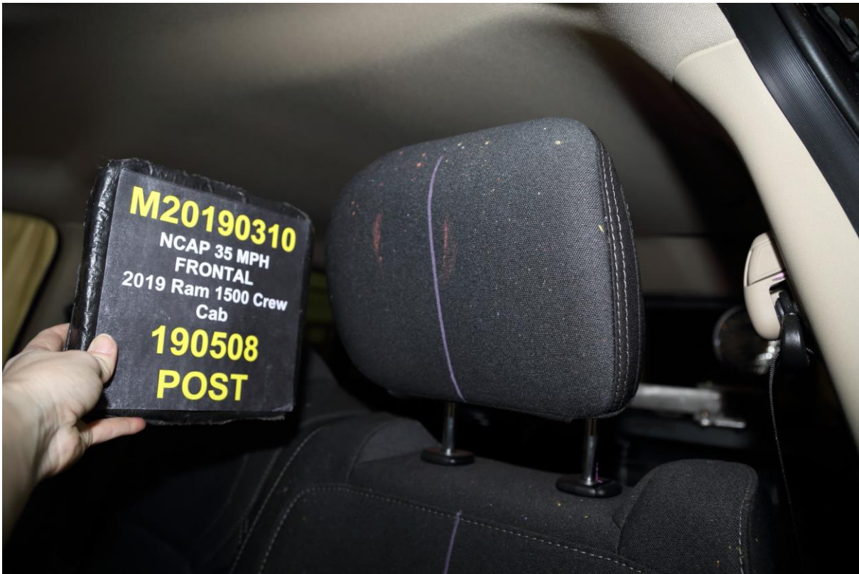
050 Post-Test Driver Dummy Contact with Headrest
