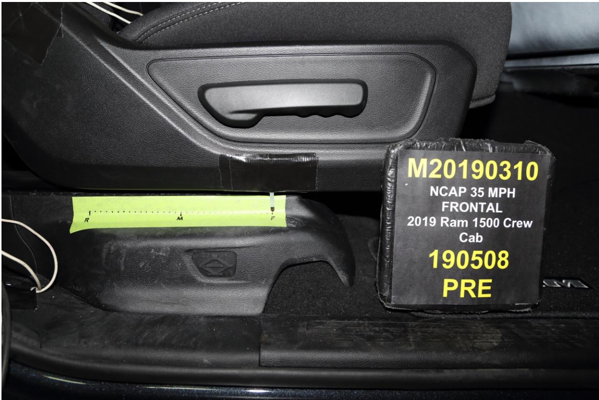
059 Pre-Test Passenger's Seat Fore-Aft Markings
