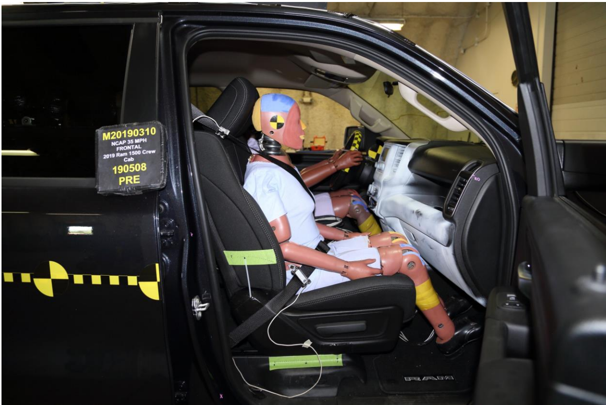
057 Pre-Test Passenger Dummy and Vehicle Interior View
