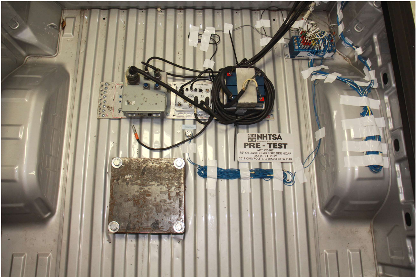
Photo No. 061 - Pre-Test Ballast View
