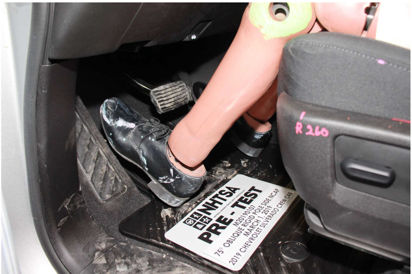
Photo No. 032 - Pre-Test Placement of Dummy Feet
