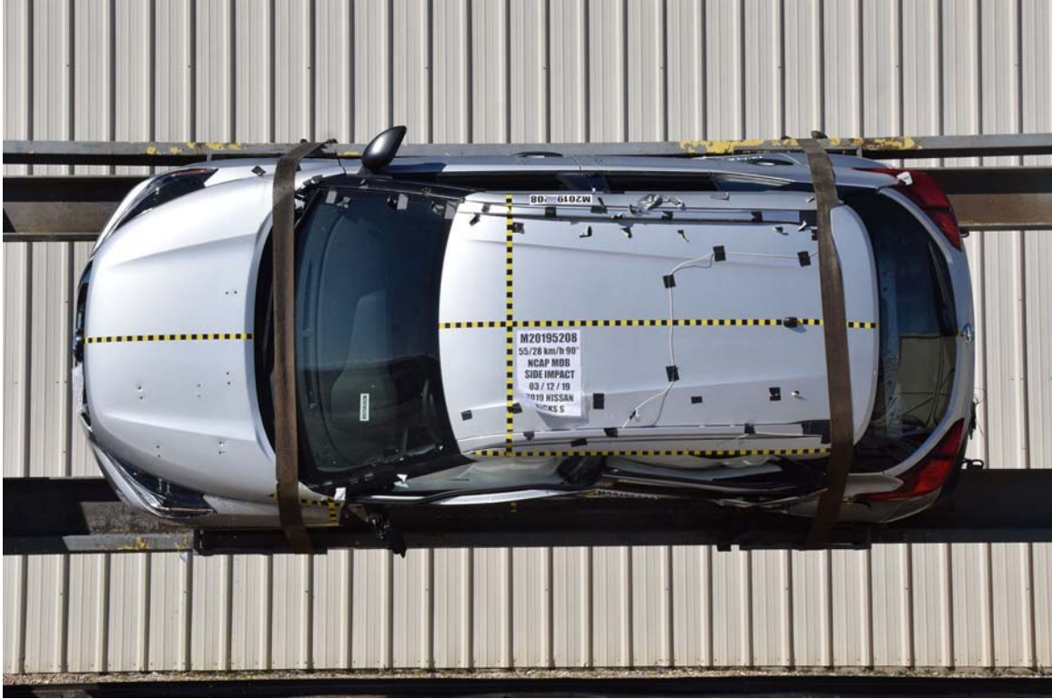
FIGURE 97. FMVSS No. 301 Static Rollover 90 Degrees
