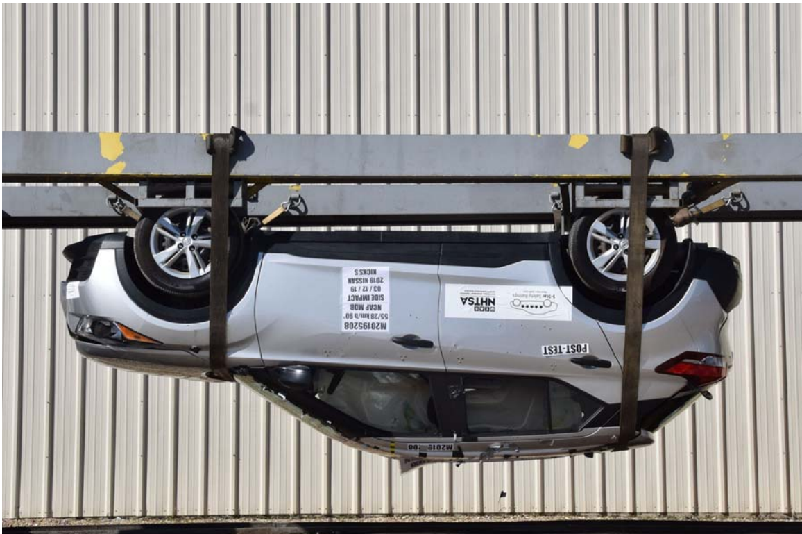
FIGURE 98. FMVSS No. 301 Static Rollover 180 Degrees
