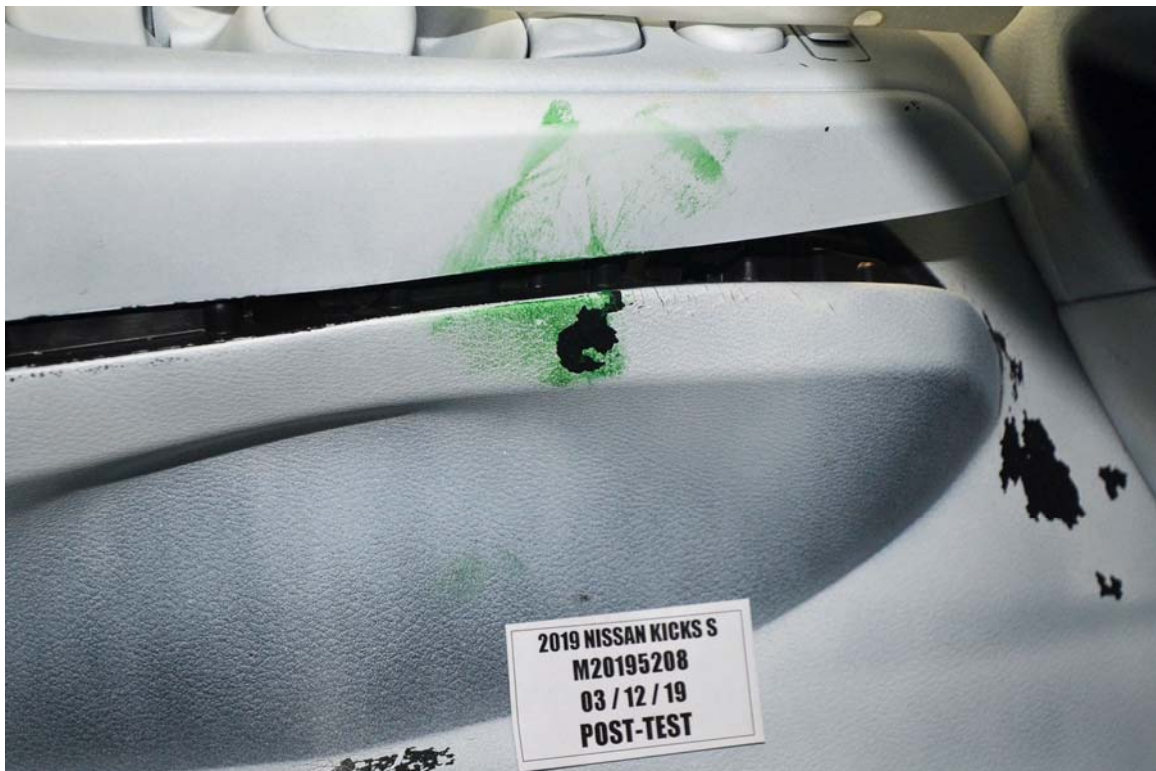
FIGURE 54. Post-Test Driver Dummy Close-Up Knee Contact View
