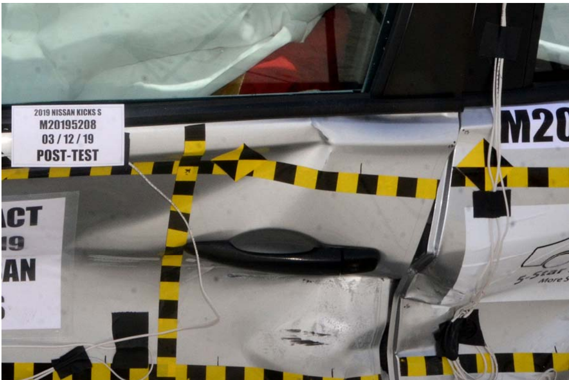
FIGURE 22. Post-Test Left Front Door Latch Close-Up
