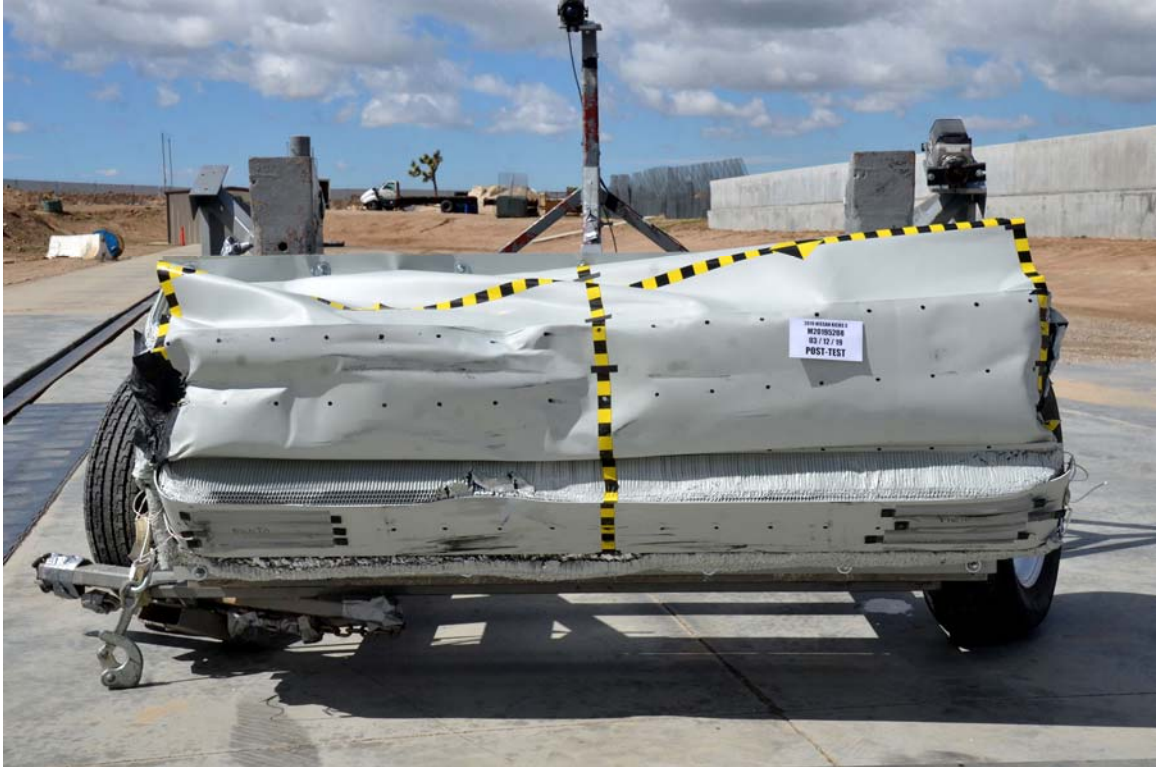
FIGURE 85. Post-Test Front View of MDB Impactor Face
