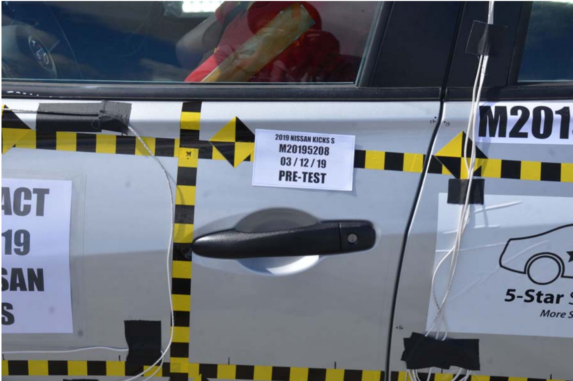
FIGURE 21. Pre-Test Left Front Door Latch Close-Up
