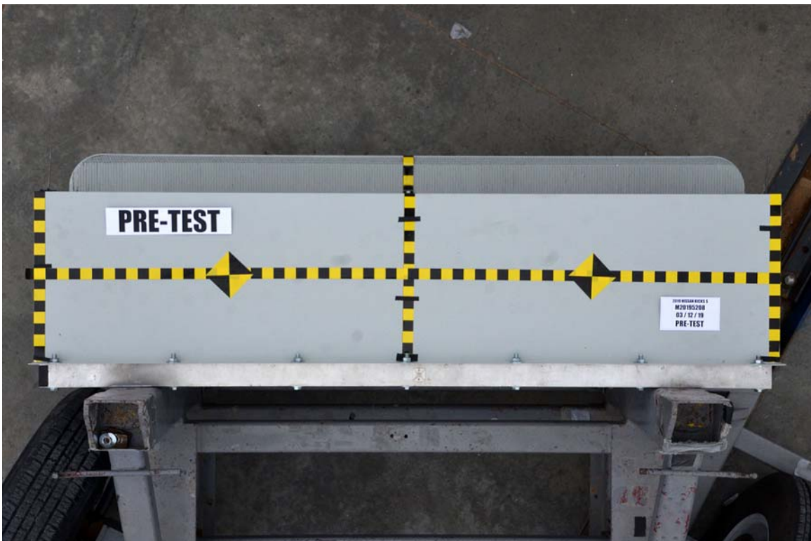
FIGURE 86. Pre-Test Top View of MDB Impactor Face
