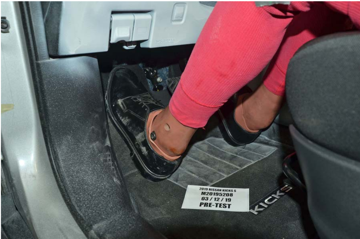
FIGURE 34. Pre-Test Placement of Driver Dummy's Feet
