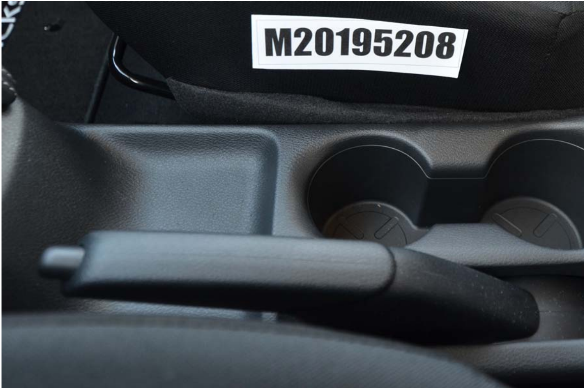
FIGURE 37. View of Disengaged Parking Brake
