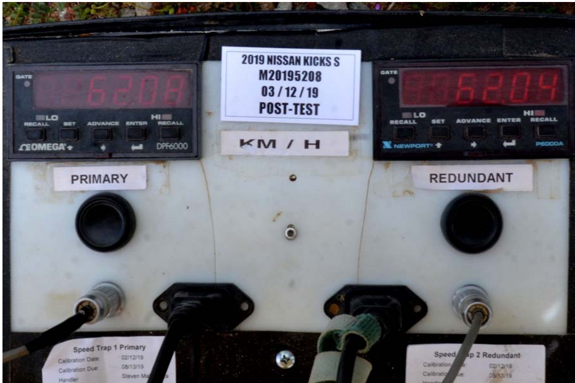
FIGURE 95. Post-Test Primary and Redundant Speed Trap Read-Out
