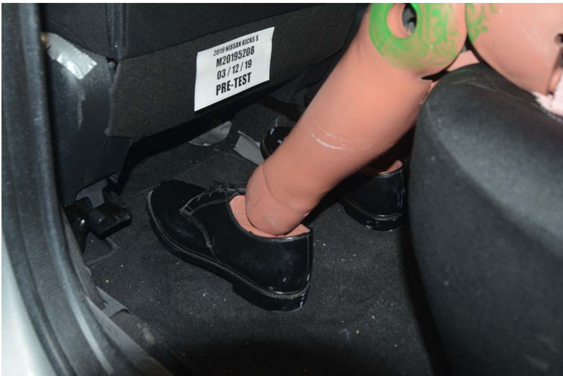
FIGURE 64. Pre-Test Placement of Rear Passenger Dummy's Feet
