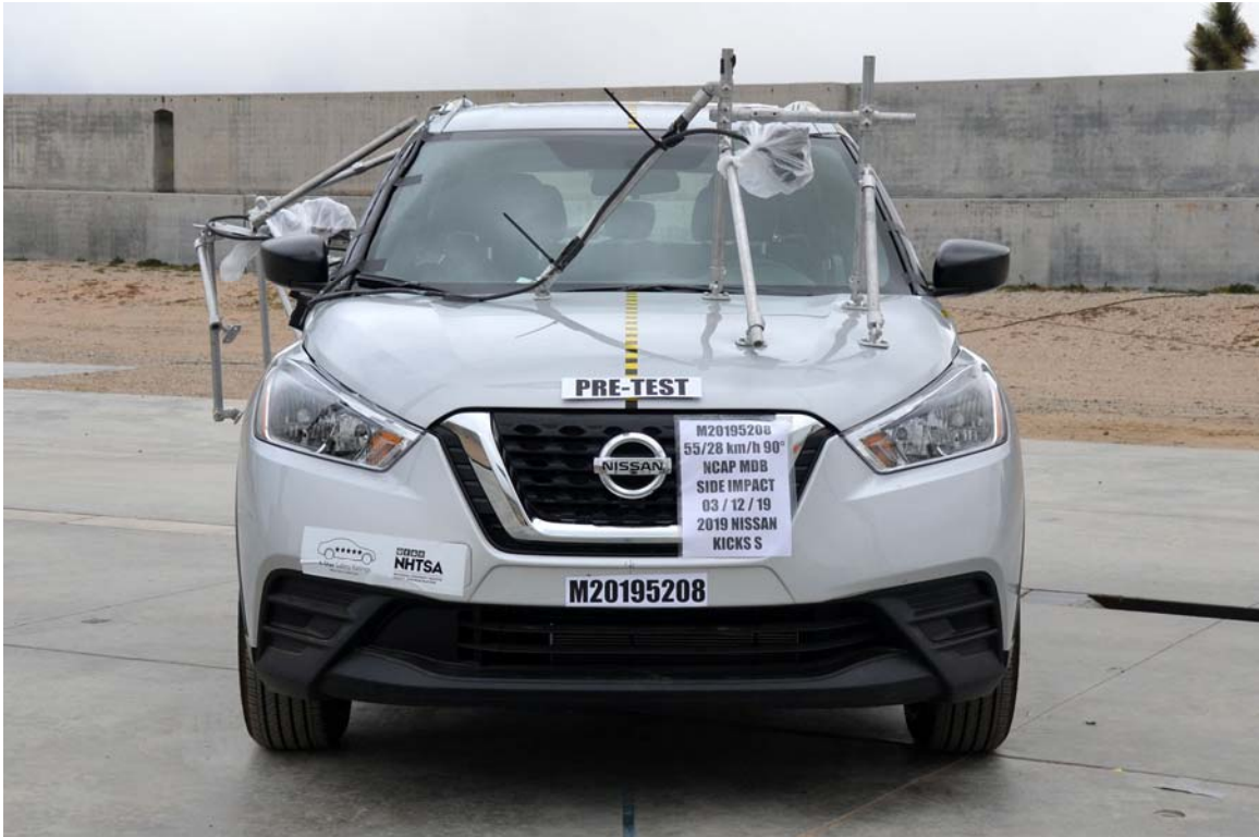
FIGURE 3. Pre-Test Frontal View of Test Vehicle
