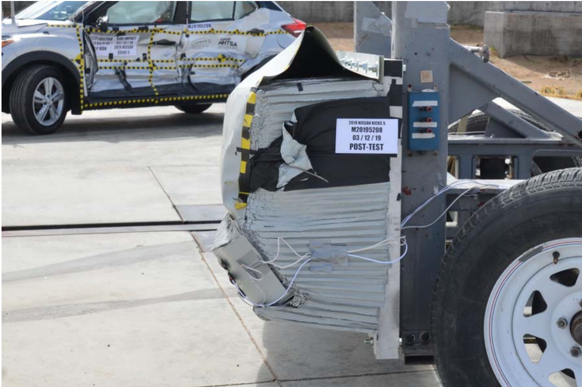
FIGURE 89. Post-Test Left Side View of MDB Impactor Face
