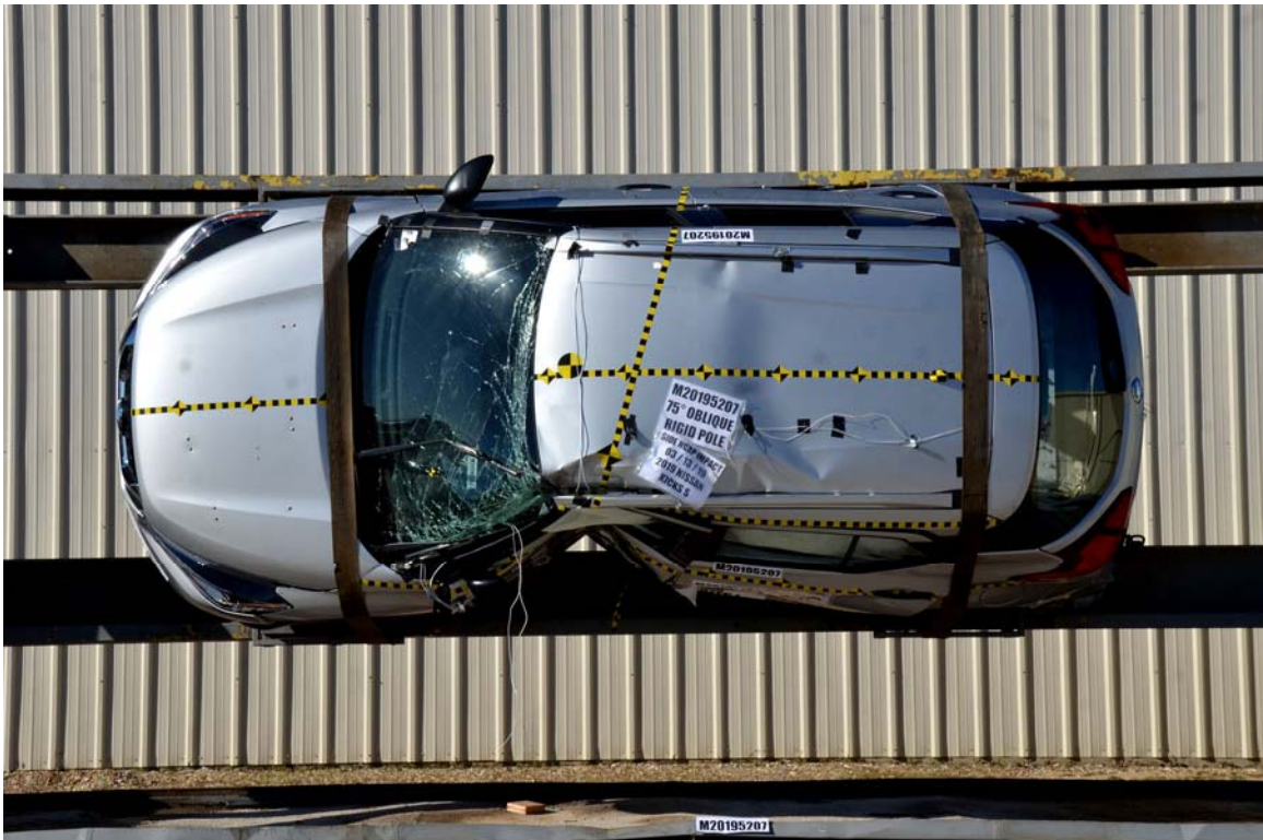
FIGURE 64. FMVSS No. 301 Static Rollover 90 Degrees
