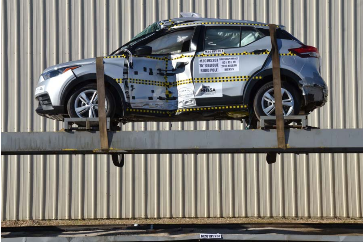
FIGURE 67. FMVSS No. 301 Static Rollover 360 Degrees
