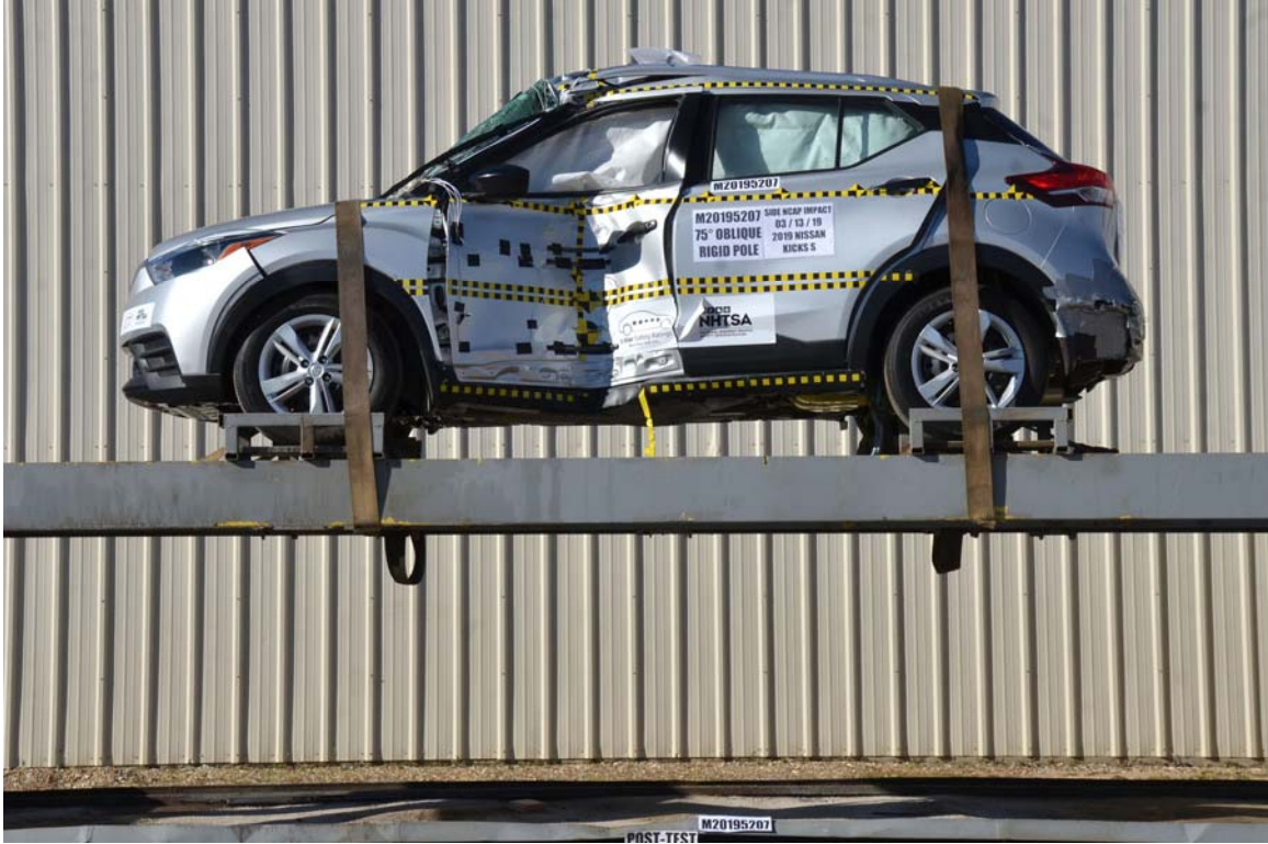
FIGURE 63. FMVSS No. 301 Static Rollover 0 Degrees
