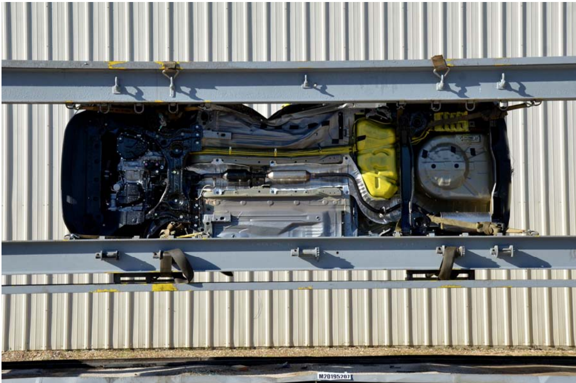
FIGURE 66. FMVSS No. 301 Static Rollover 270 Degrees
