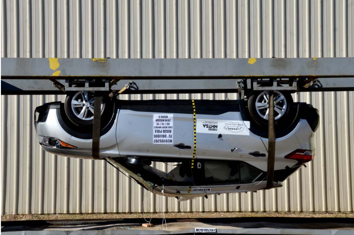
FIGURE 65. FMVSS No. 301 Static Rollover 180 Degrees
