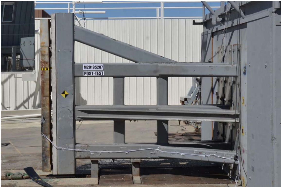
FIGURE 60. Post-Test Pole Barrier Side View
