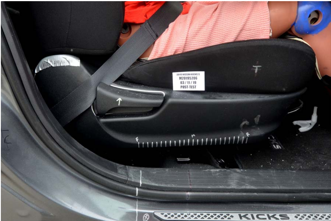
FIGURE 58. Post-Test Passenger's Seat Fore-Aft Markings
