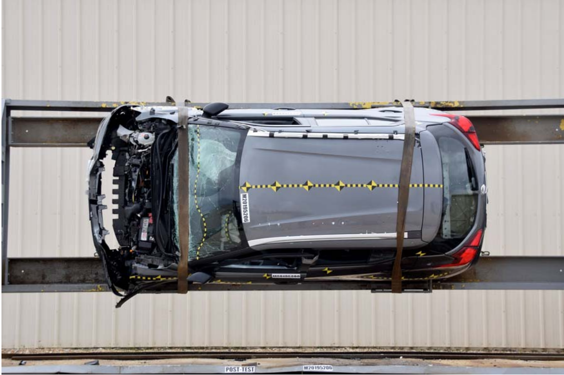
FIGURE 74. Vehicle at 90° on Static Rollover Device
