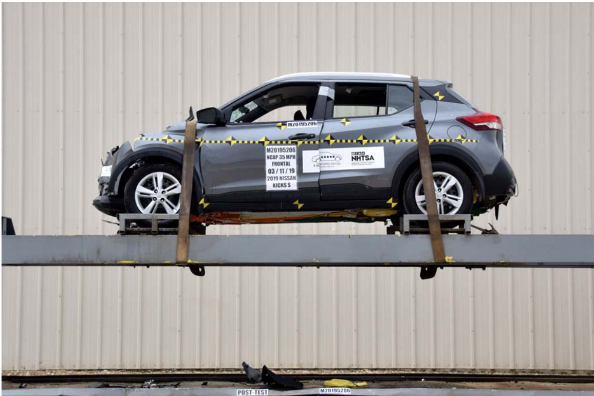
FIGURE 77. Vehicle at 360° on Static Rollover Device
