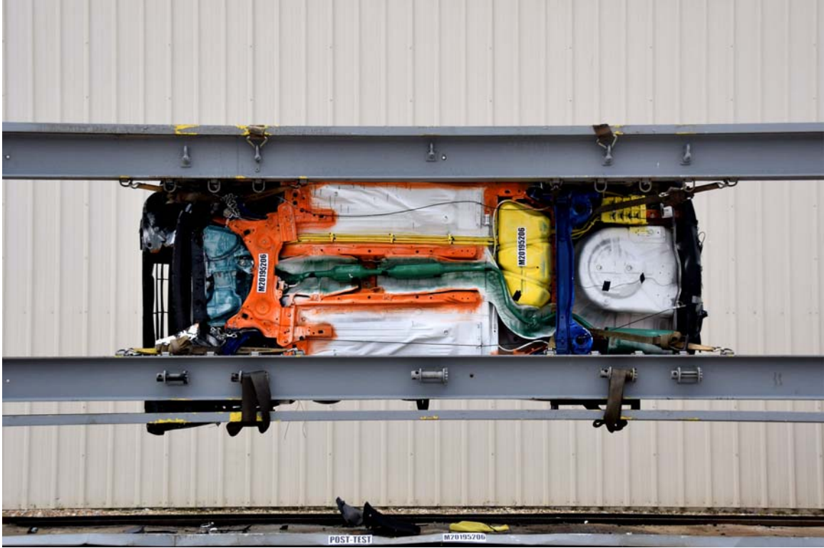
FIGURE 76. Vehicle at 270° on Static Rollover Device
