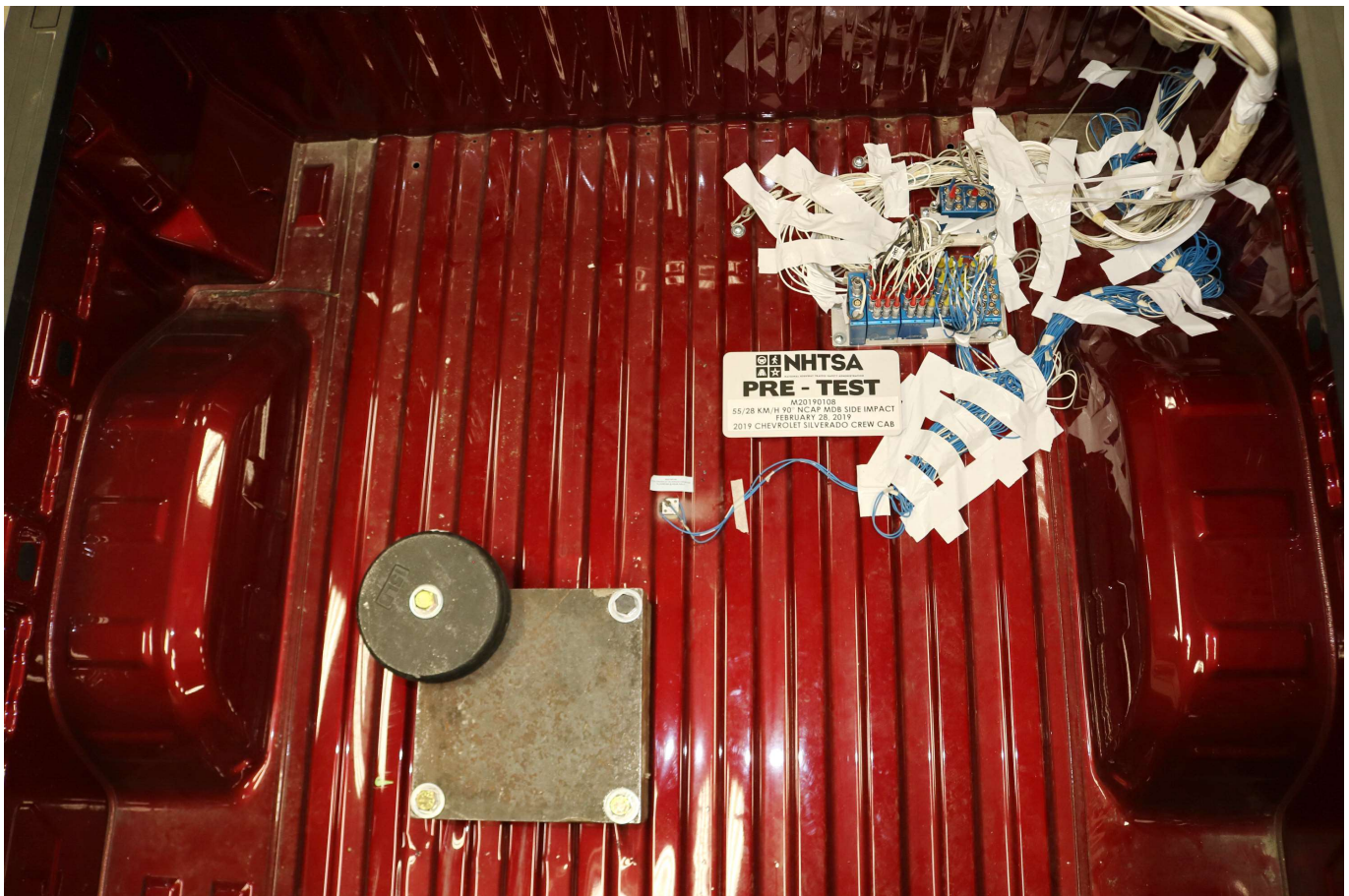
Photo No. 094 - Pre-Test Ballast View
