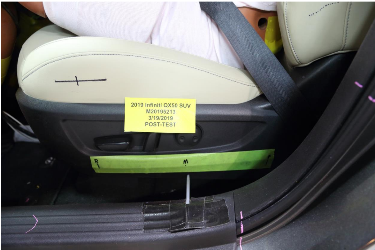
037 Post-Test Driver's Seat Fore-Aft Markings
