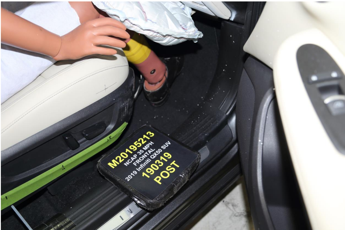
066 Post-Test Passenger Dummy Feet
