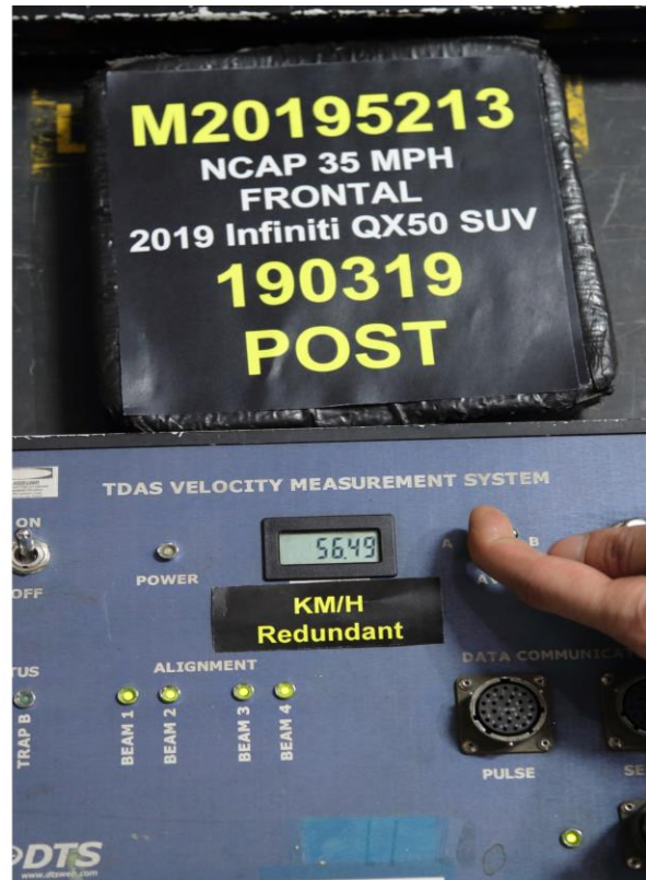
076 Post-Test Speed Trap Read out
