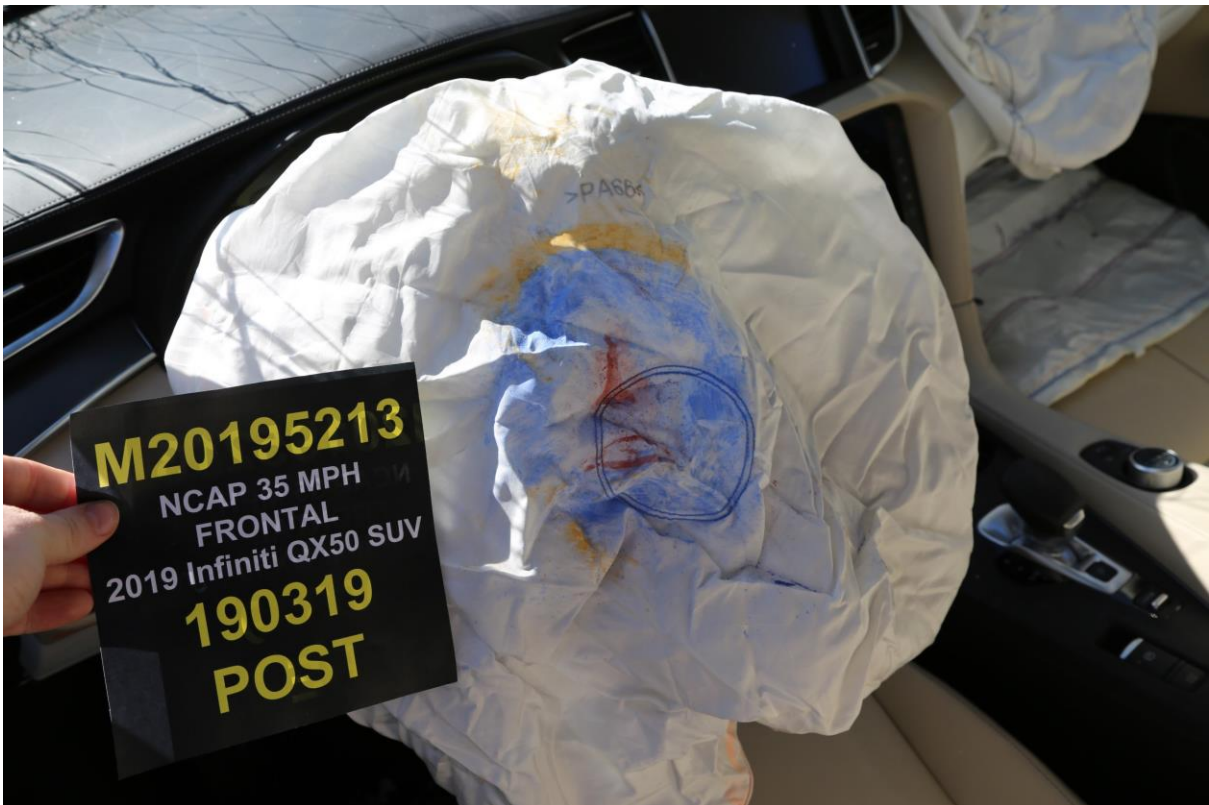
049 Post-Test Driver Dummy Contact with Airbag
