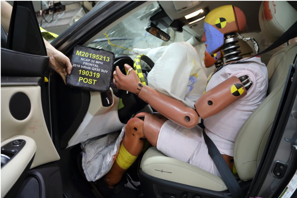
052 Post-Test View of the Steering Wheel
