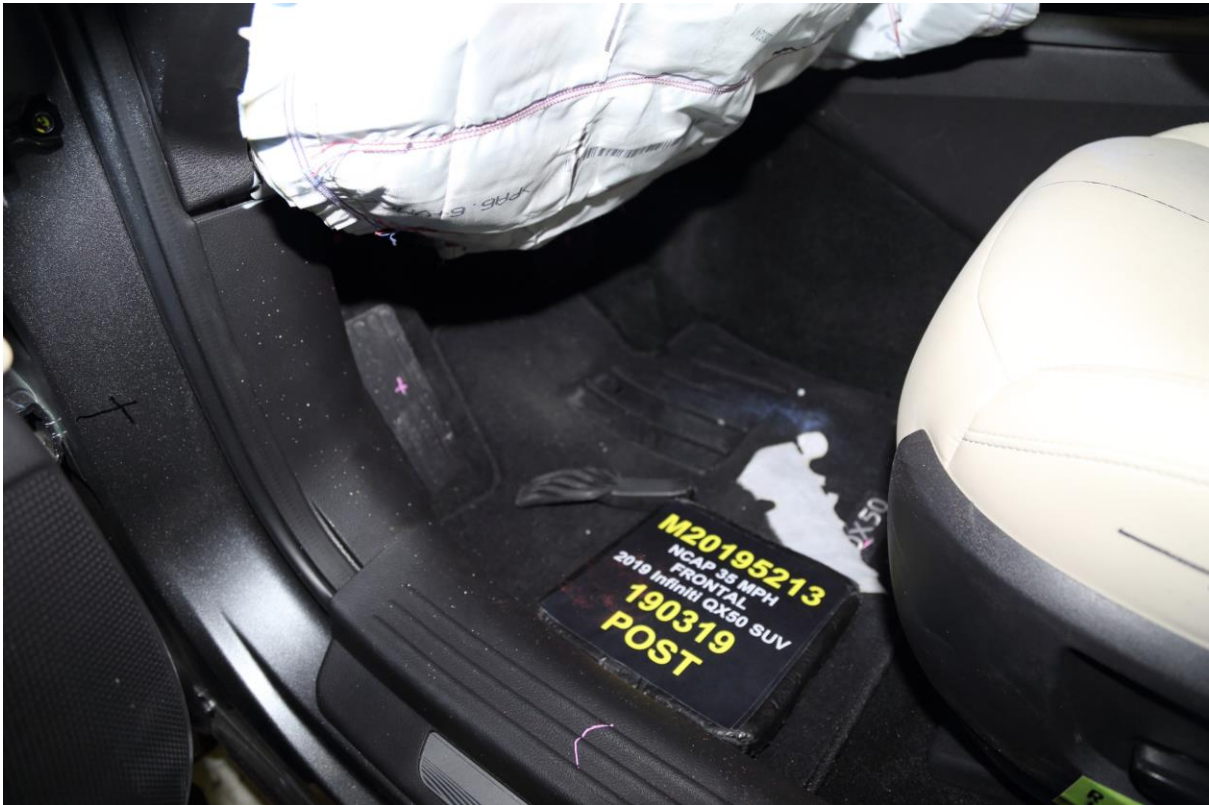
047 Post-Test Driver's Side Floorpan
