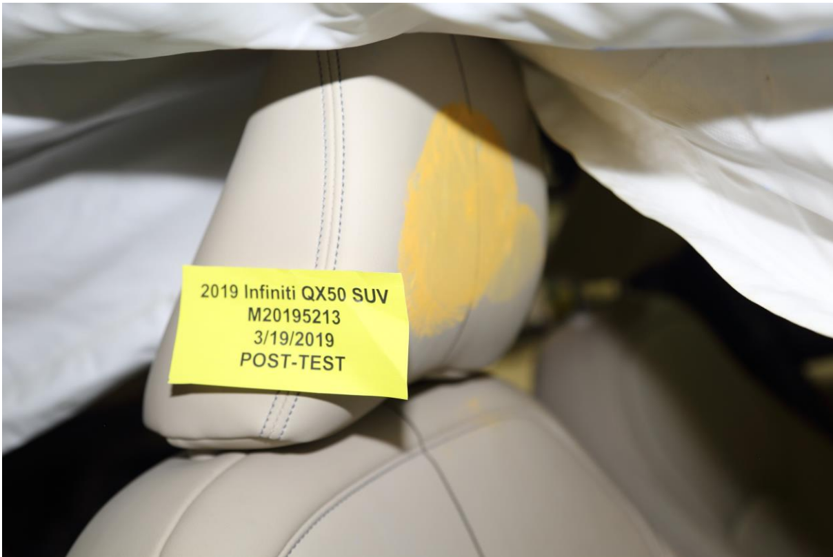
073 Post-Test Passenger Dummy Contact with Headrest
