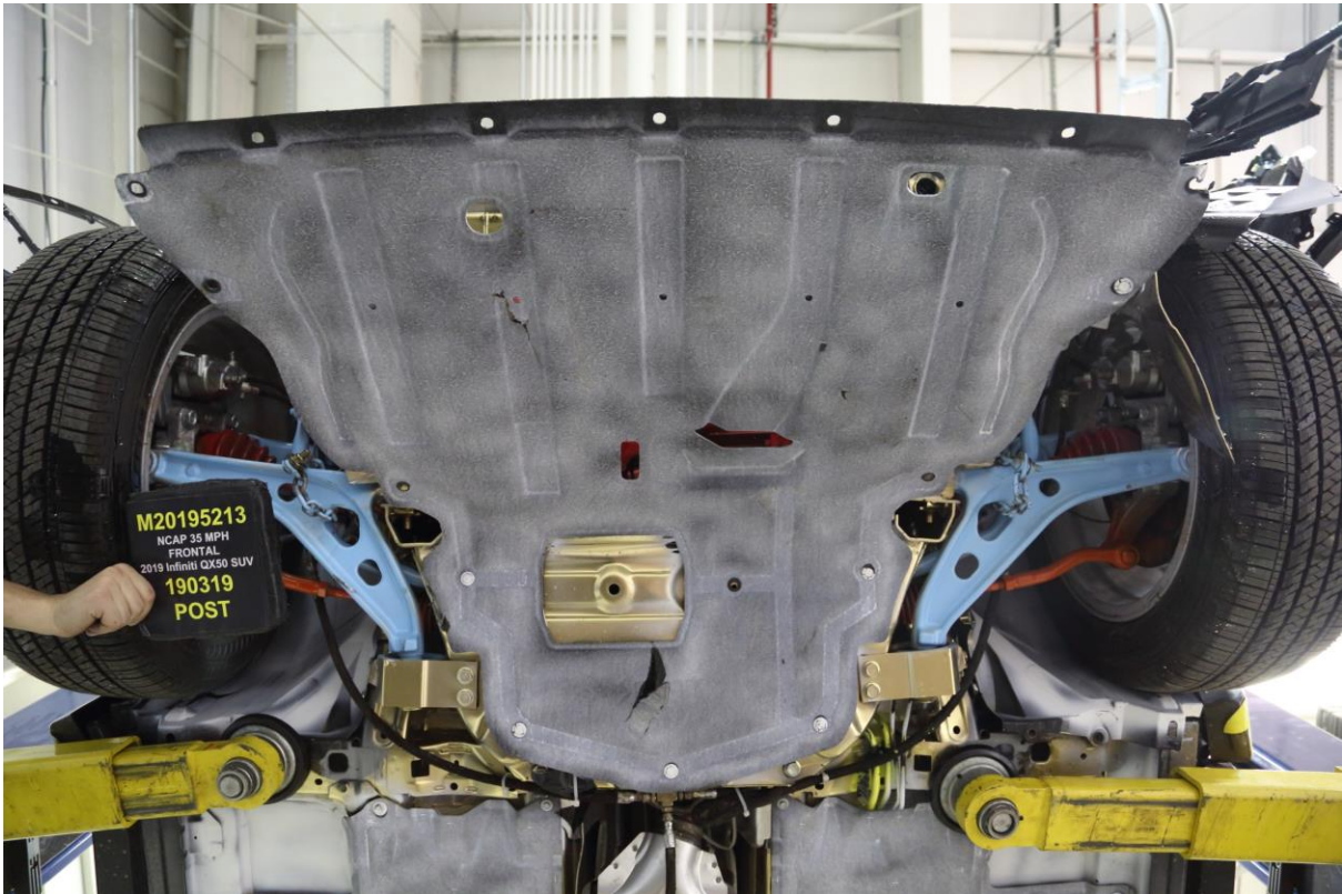
025 Post-Test Front Underbody View
