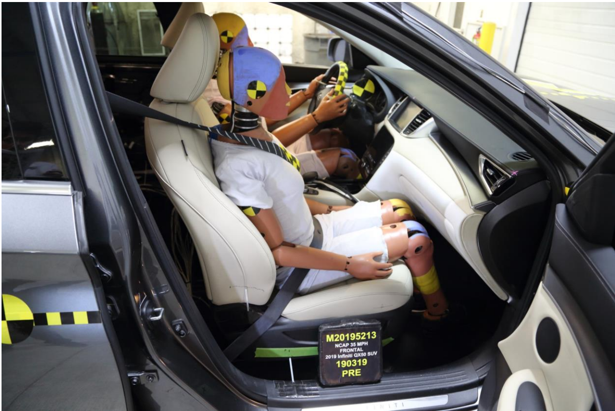
057 Pre-Test Passenger Dummy and Vehicle Interior View
