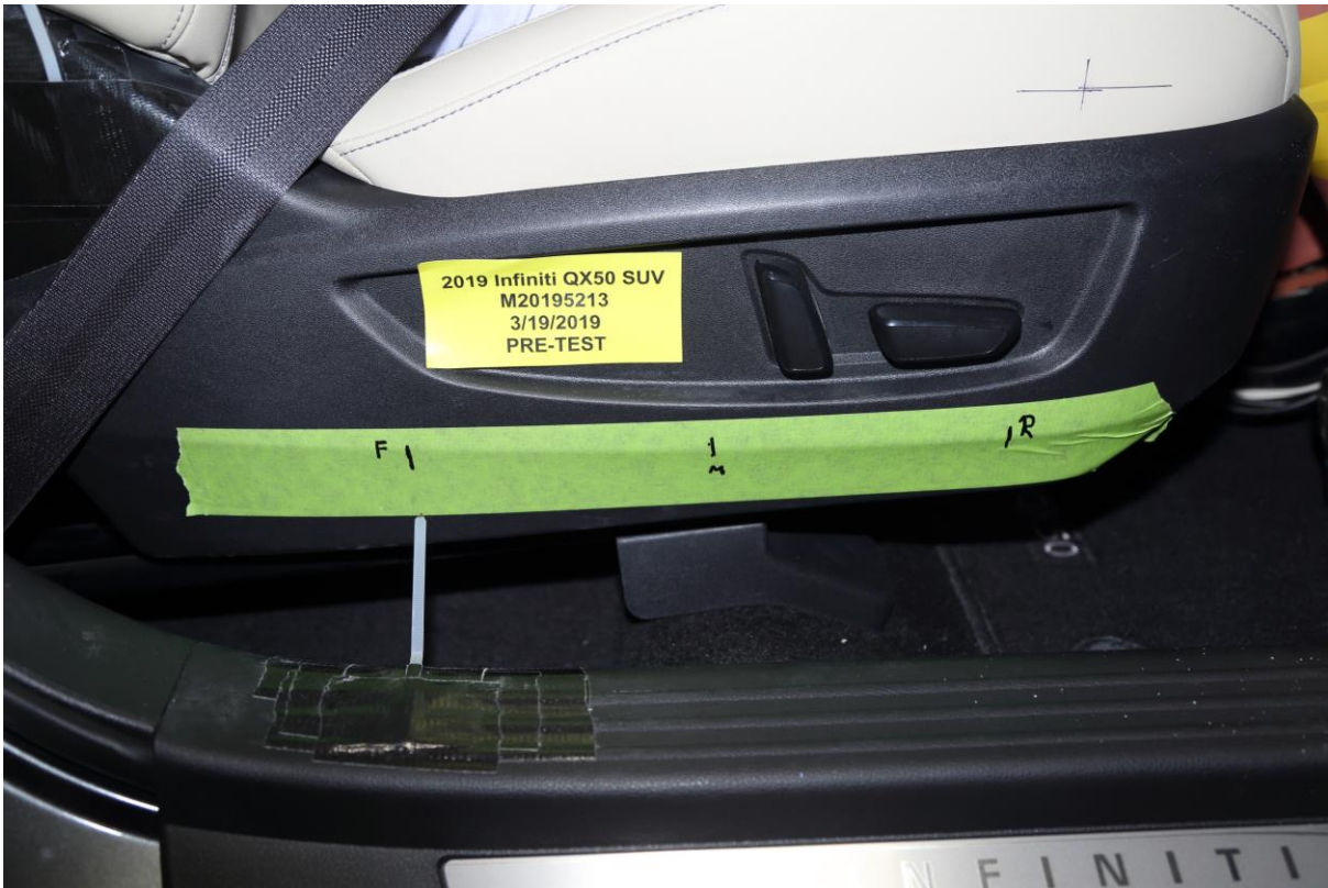
059 Pre-Test Passenger's Seat Fore-Aft Markings
