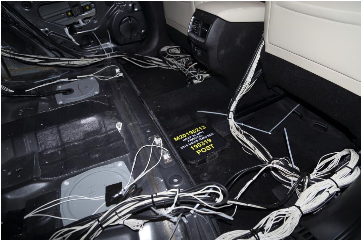
029 Post-Test Dummy Cable Routing
