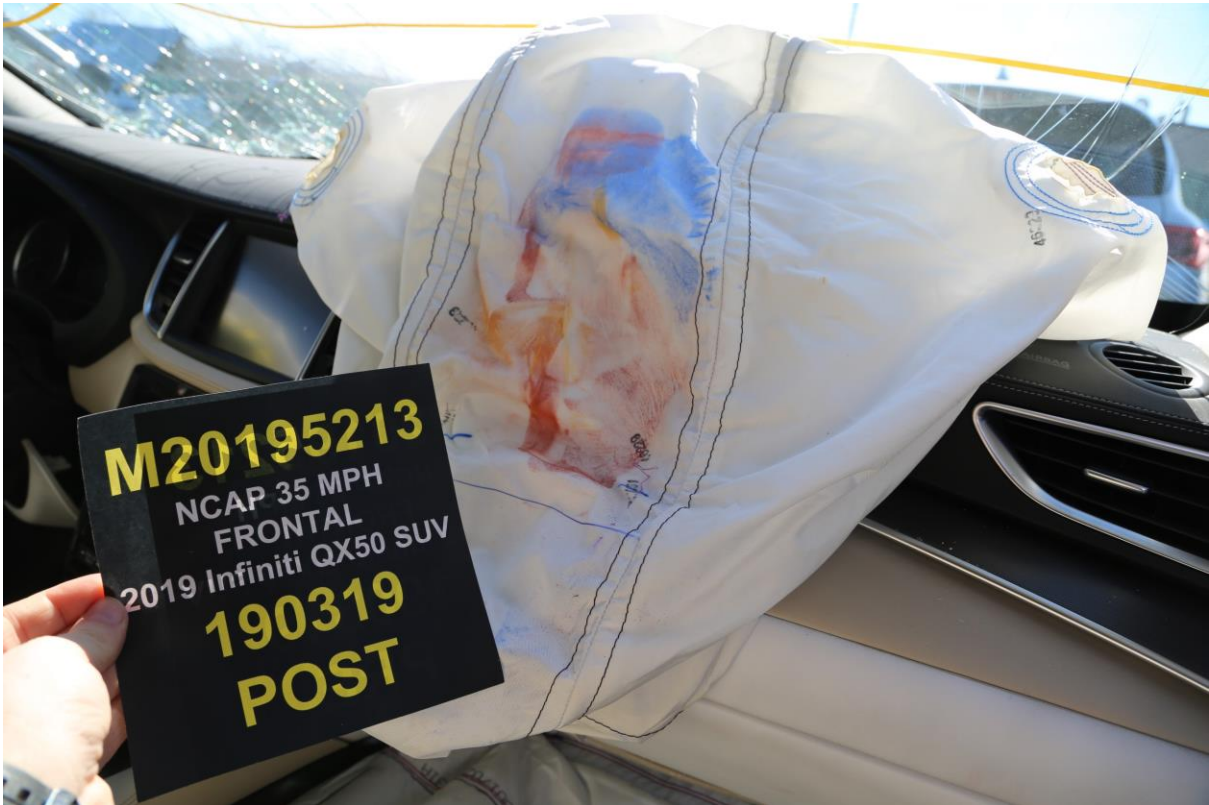
072 Post-Test Passenger Dummy Contact with Airbag
