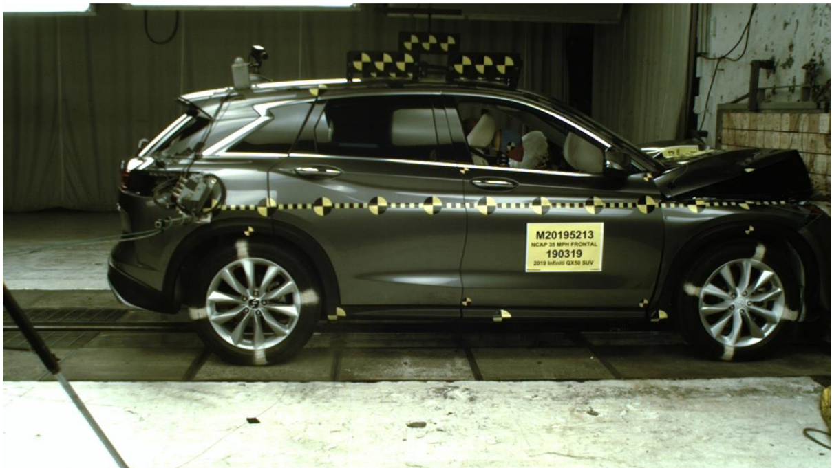
082 2019 Infiniti QX50 SUV Frontal Impact Event
