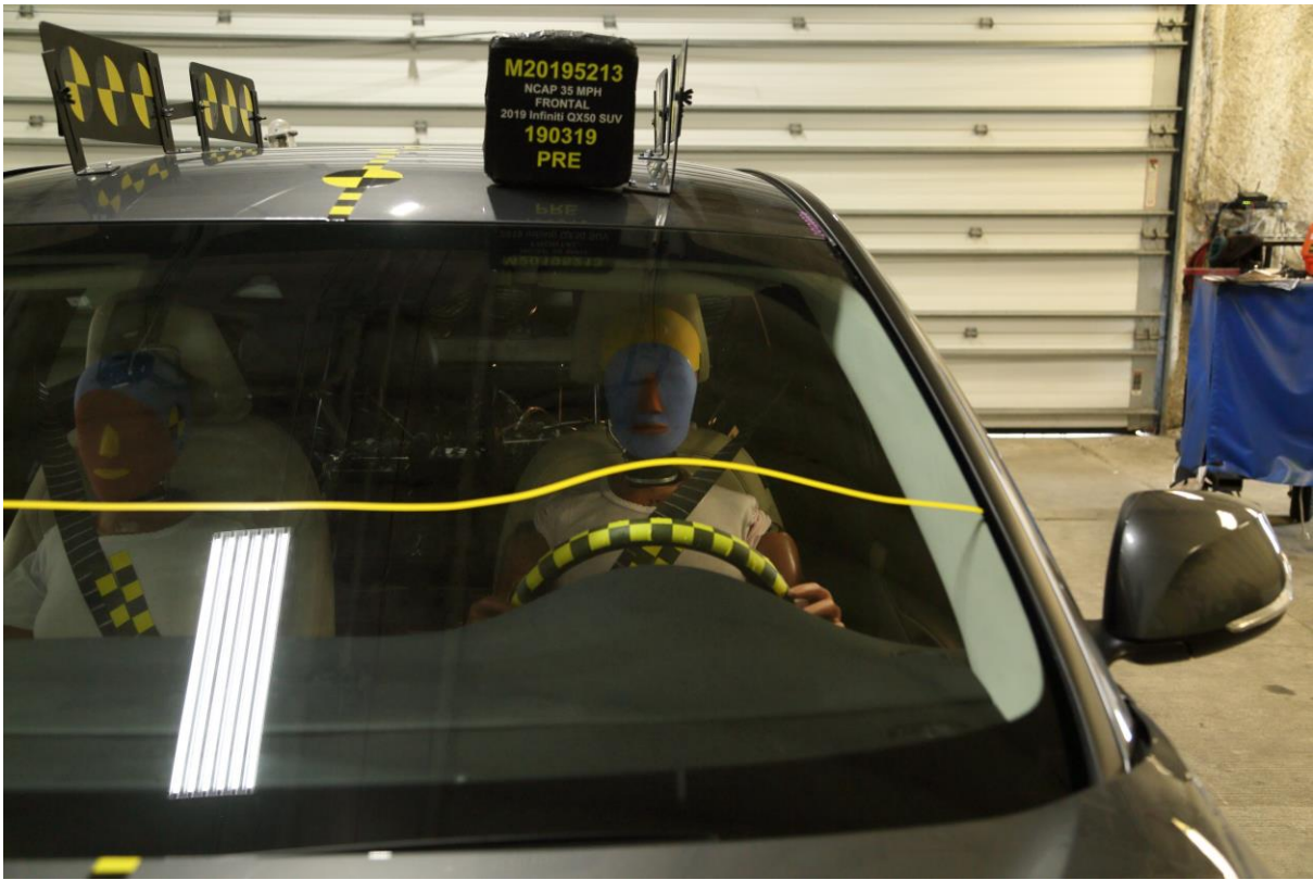
030 Pre-Test Driver Dummy Front View
