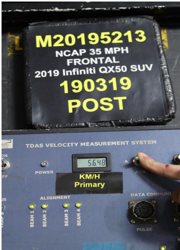
076 Post-Test Speed Trap Read out
