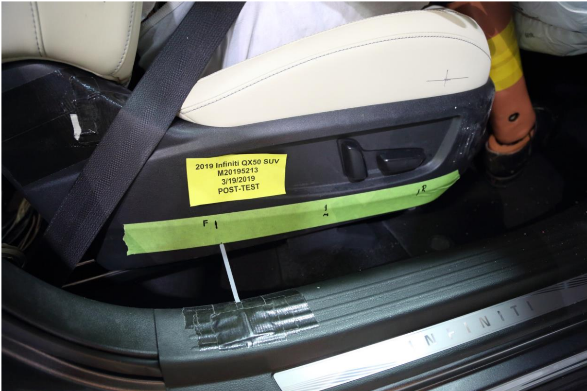
060 Post-Test Passenger's Seat Fore-Aft Markings
