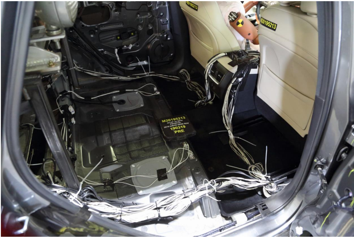
028 Pre-Test Dummy Cable Routing
