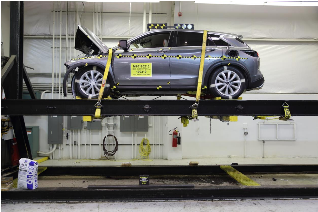
077 Vehicle at 0° on Static Rollover Device
