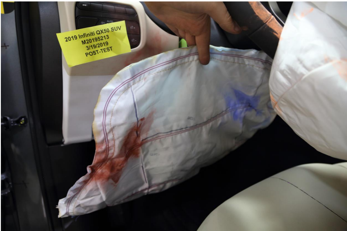
045 Post-Test Driver's Side Knee Bolster
