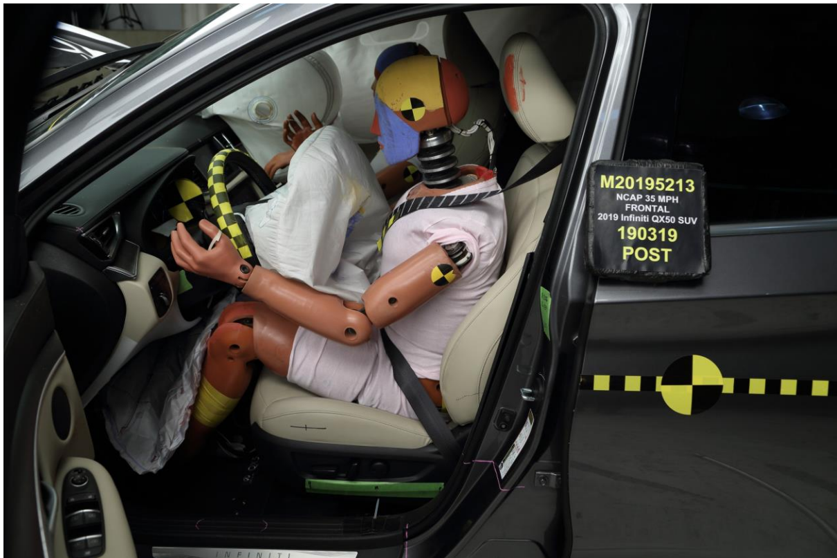
035 Post-Test Driver Dummy and Vehicle Interior View
