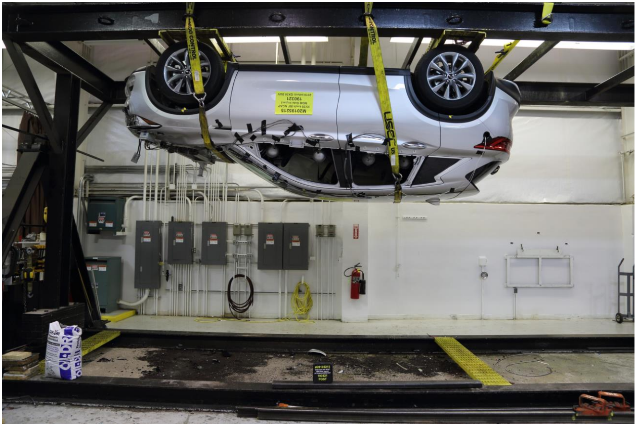
098 FMVSS No. 301 Static Rollover 180 Degrees
