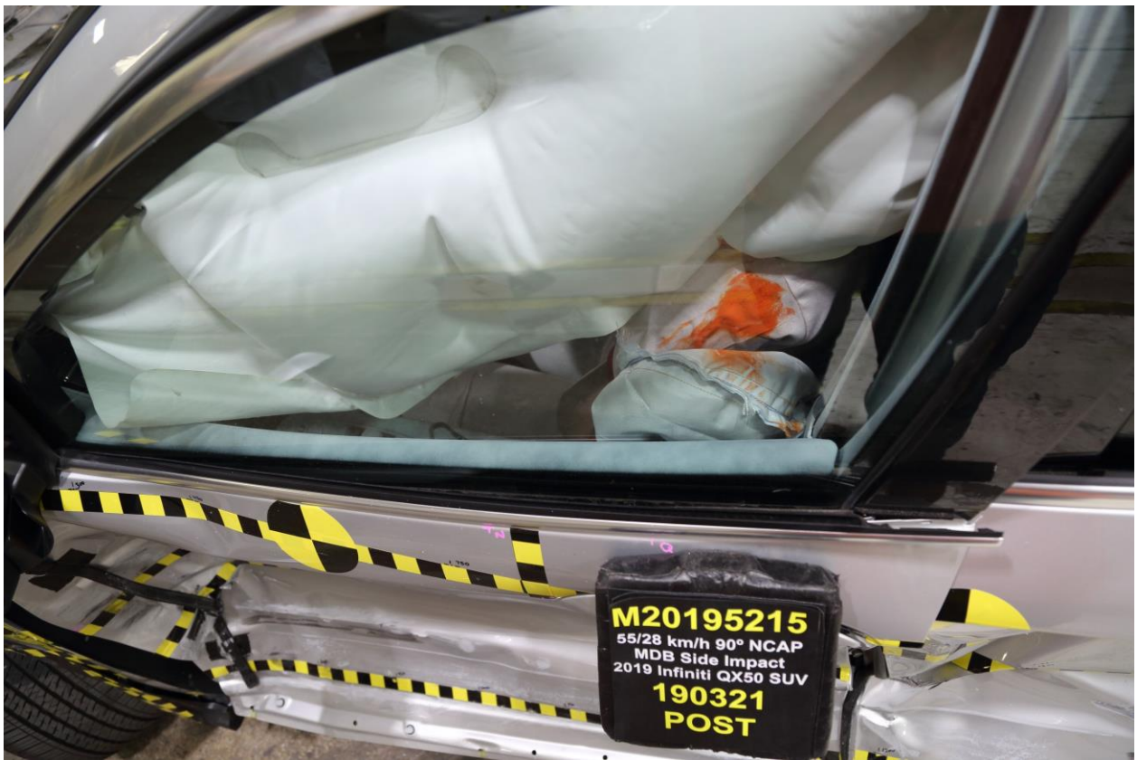
043 Post-Test Driver Dummy and Door Clearance View
