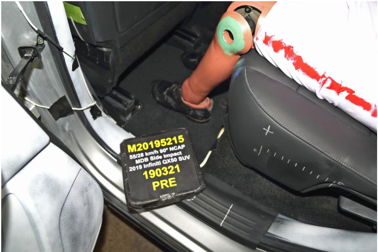
064 Pre-Test Placement of Rear Passenger Dummy's Feet
