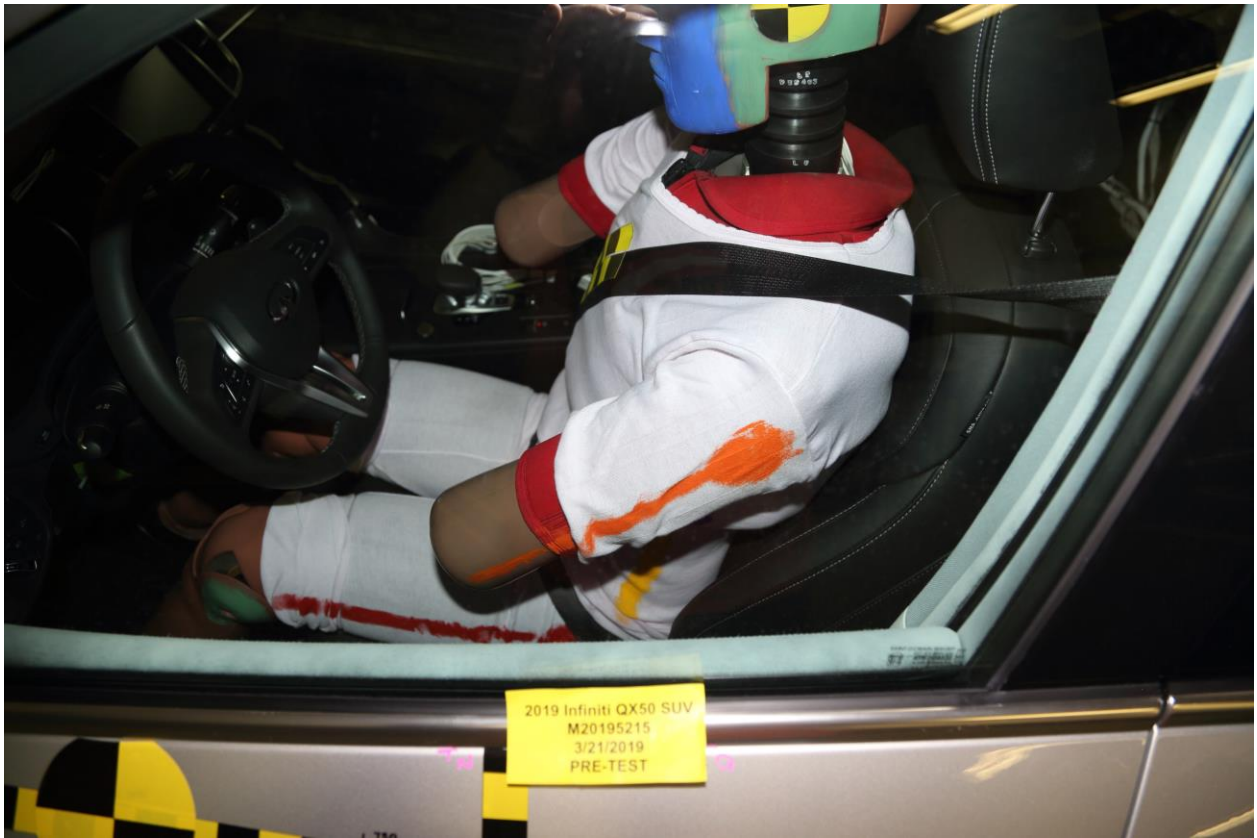
042 Pre-Test Driver Dummy and Door Clearance View
