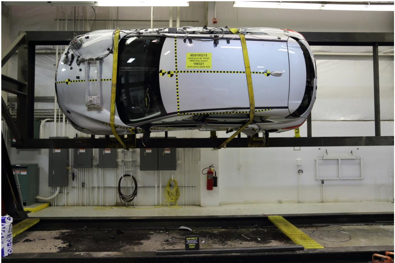
097 FMVSS No. 301 Static Rollover 90 Degrees
