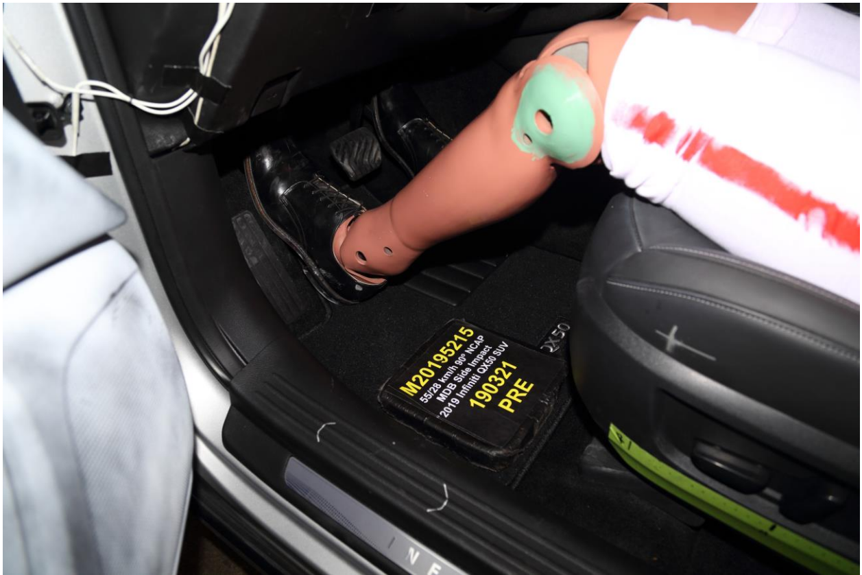
034 Pre-Test Placement of Driver's Dummy Feet
