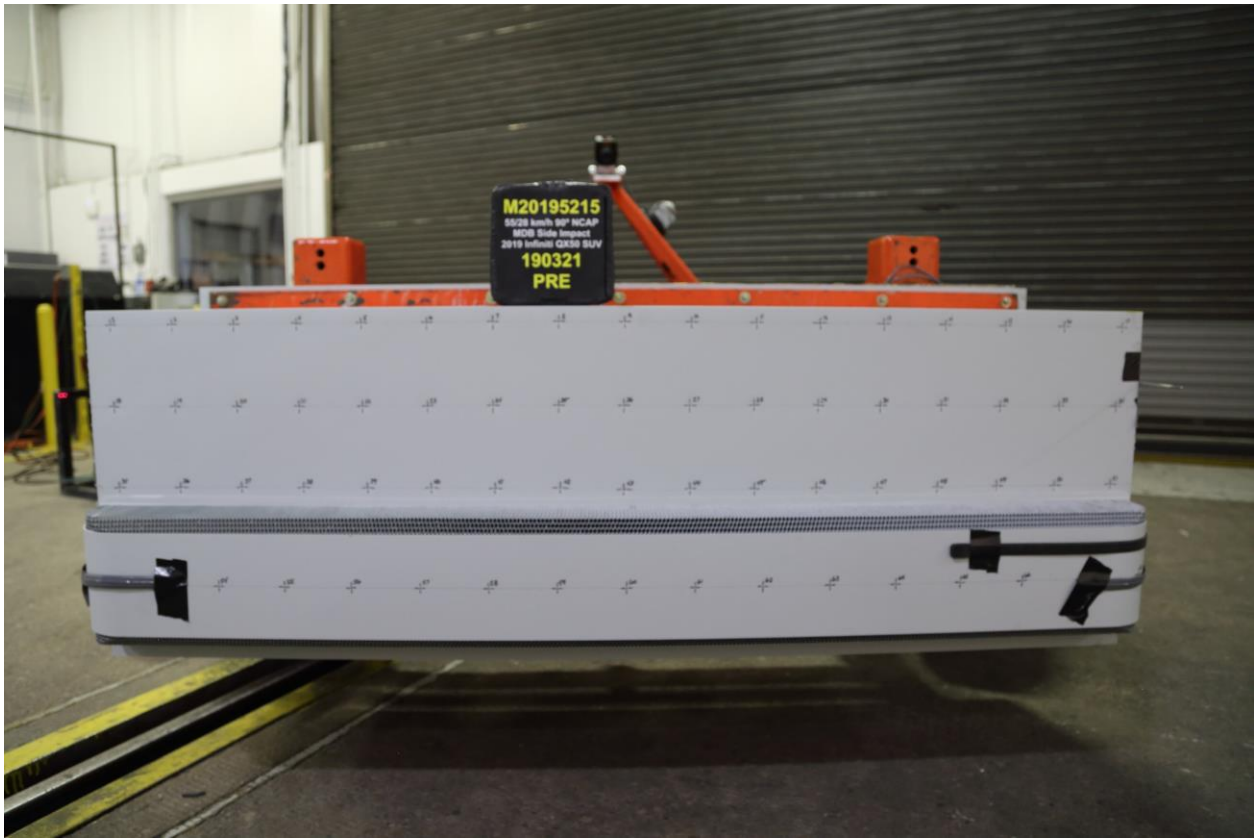
084 Pre-Test Front View of MDB Impactor Face
