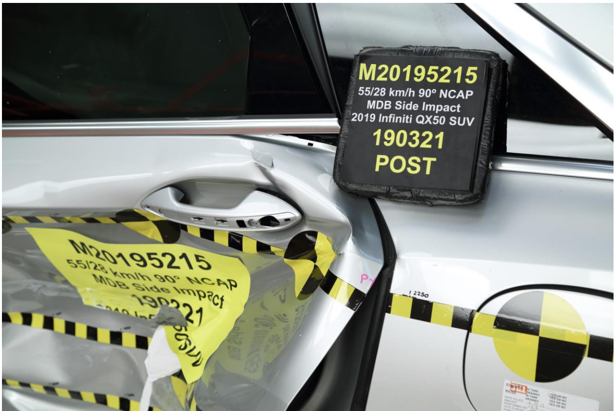
024 Post-Test Left Rear Door Latch Close-Up
