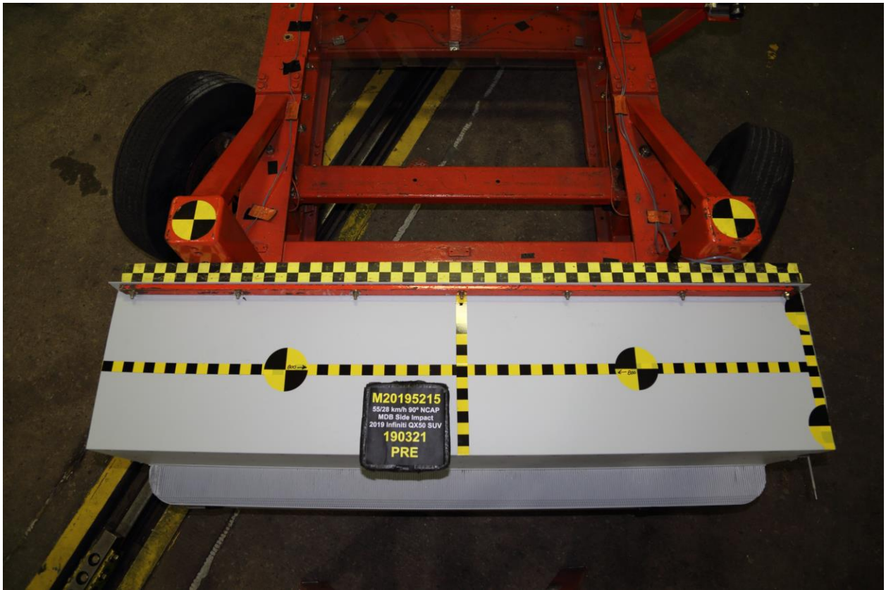
086 Pre-Test Top View of MDB Impactor Face
