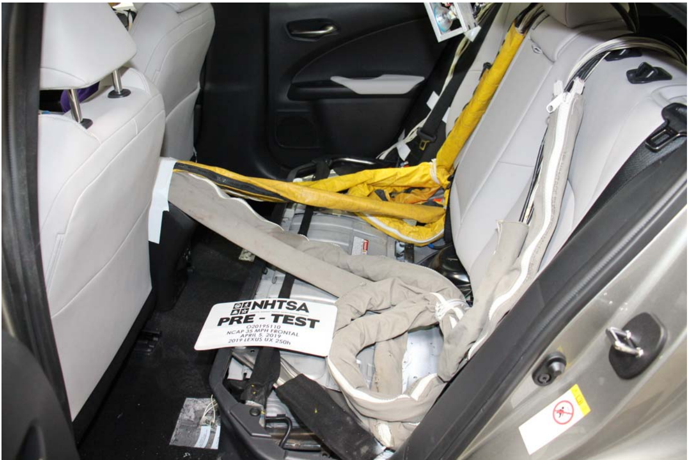
Photo No. 028 - Pre-Test Dummy Cable Routing
