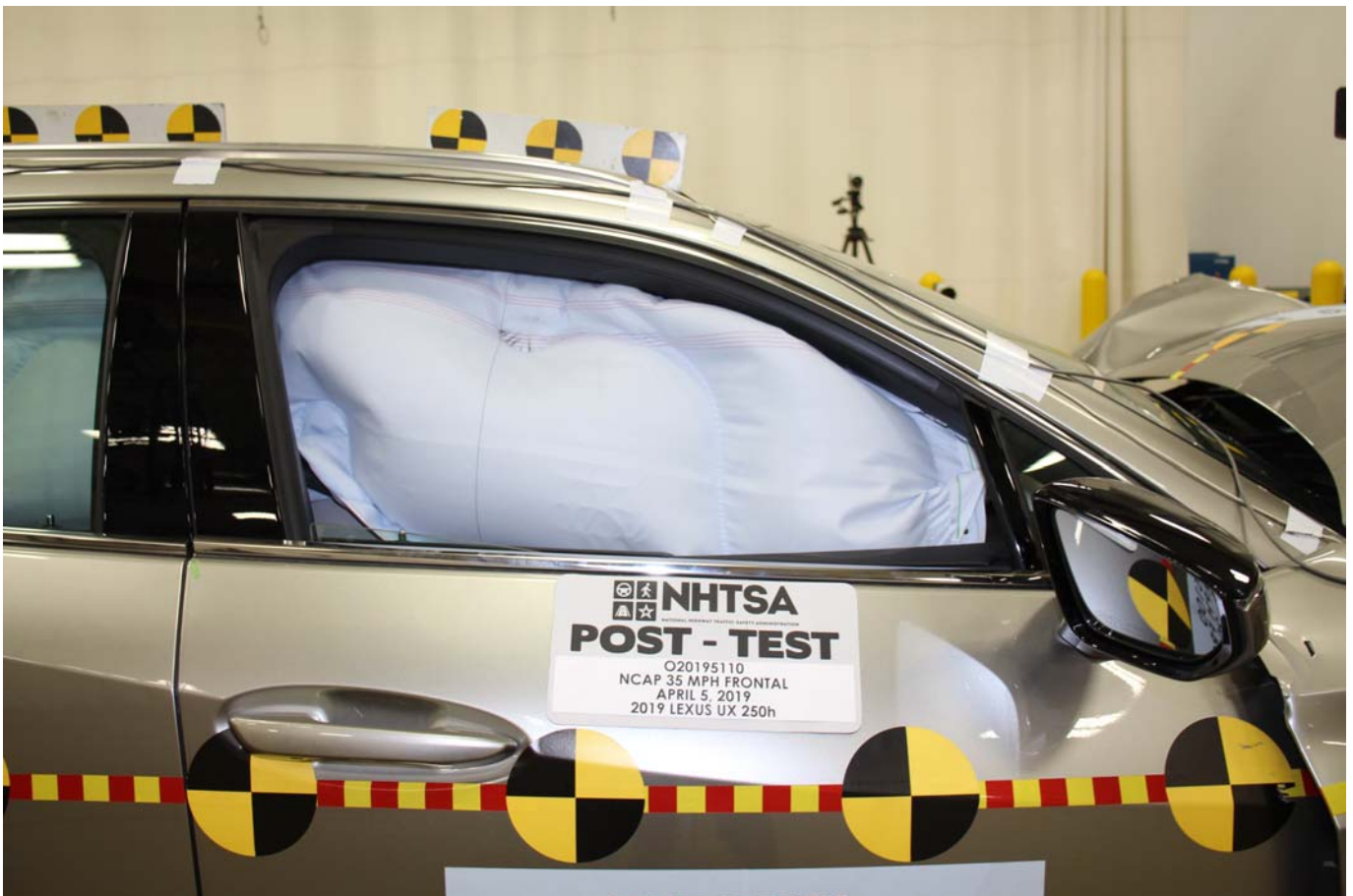
Photo No. 054 - Post-Test Passenger Dummy Window View
