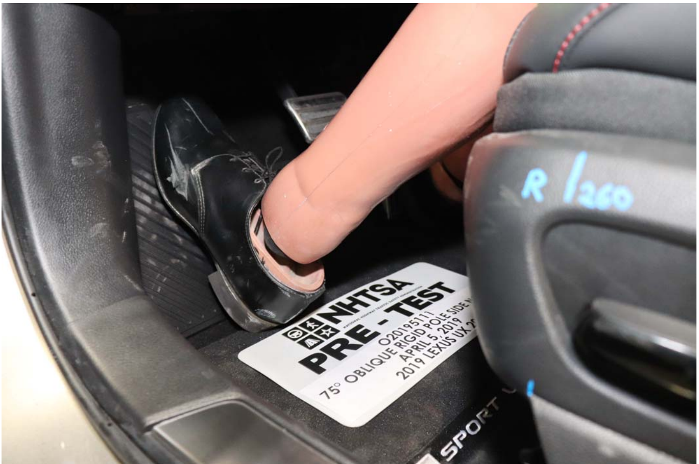
Photo No. 032 - Pre-Test Placement of Dummy Feet
