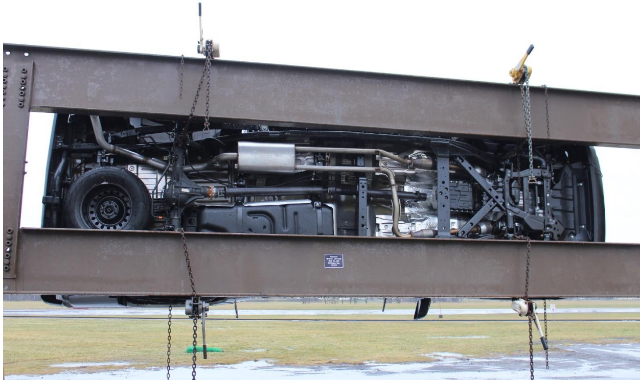
Figure A-97: FMVSS No. 301 Static Rollover 90 Degrees
