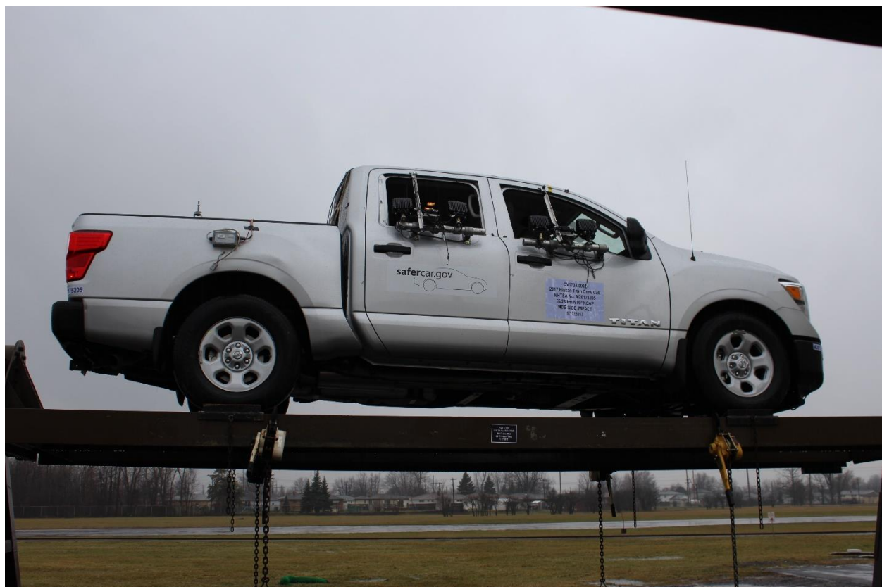
Figure A-96: FMVSS No. 301 Static Rollover 0 Degrees
