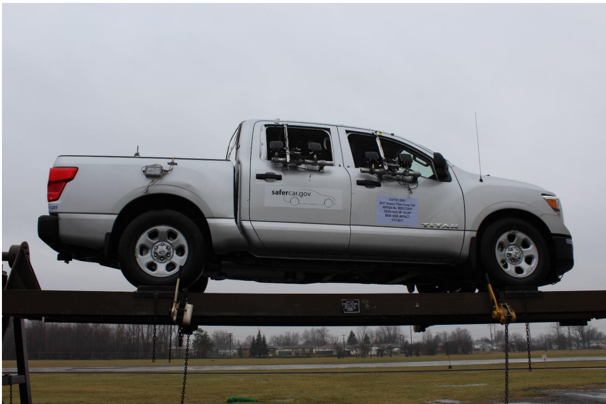
Figure A-100: FMVSS No. 301 Static Rollover 360 Degrees
