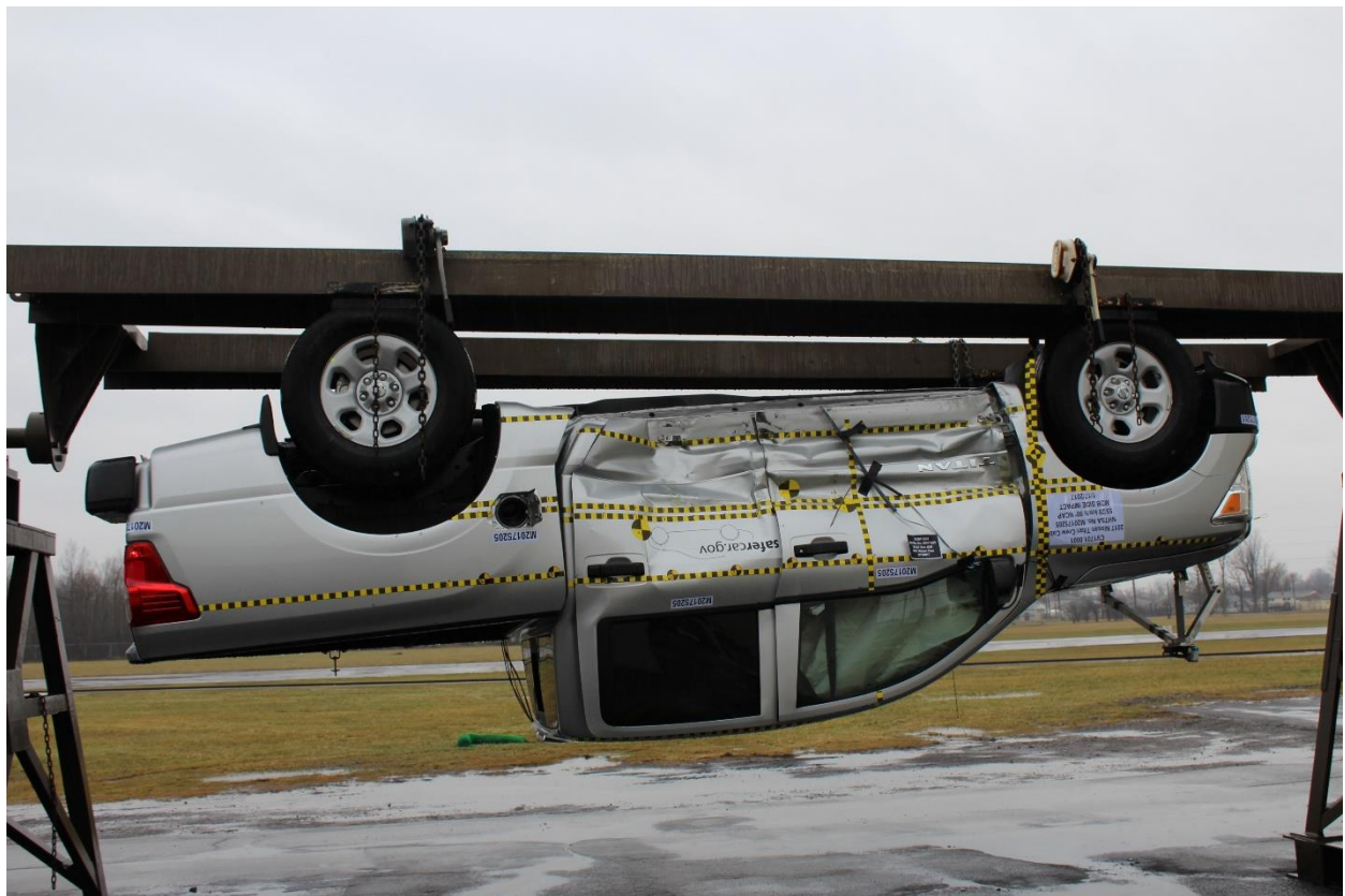
Figure A-98: FMVSS No. 301 Static Rollover 180 Degrees
