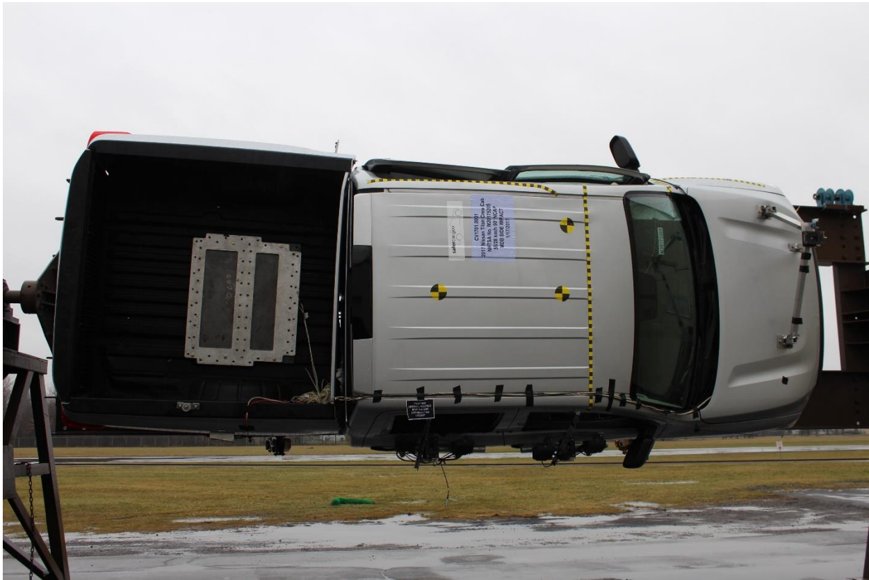
Figure A-99: FMVSS No. 301 Static Rollover 270 Degrees
