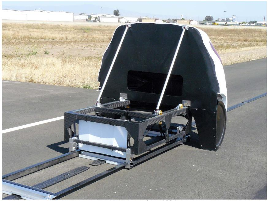
Figure A7. Load Frame/Slider of SSV
