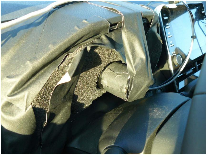
Figure A12. Sensor for Detecting Visual Alerts
