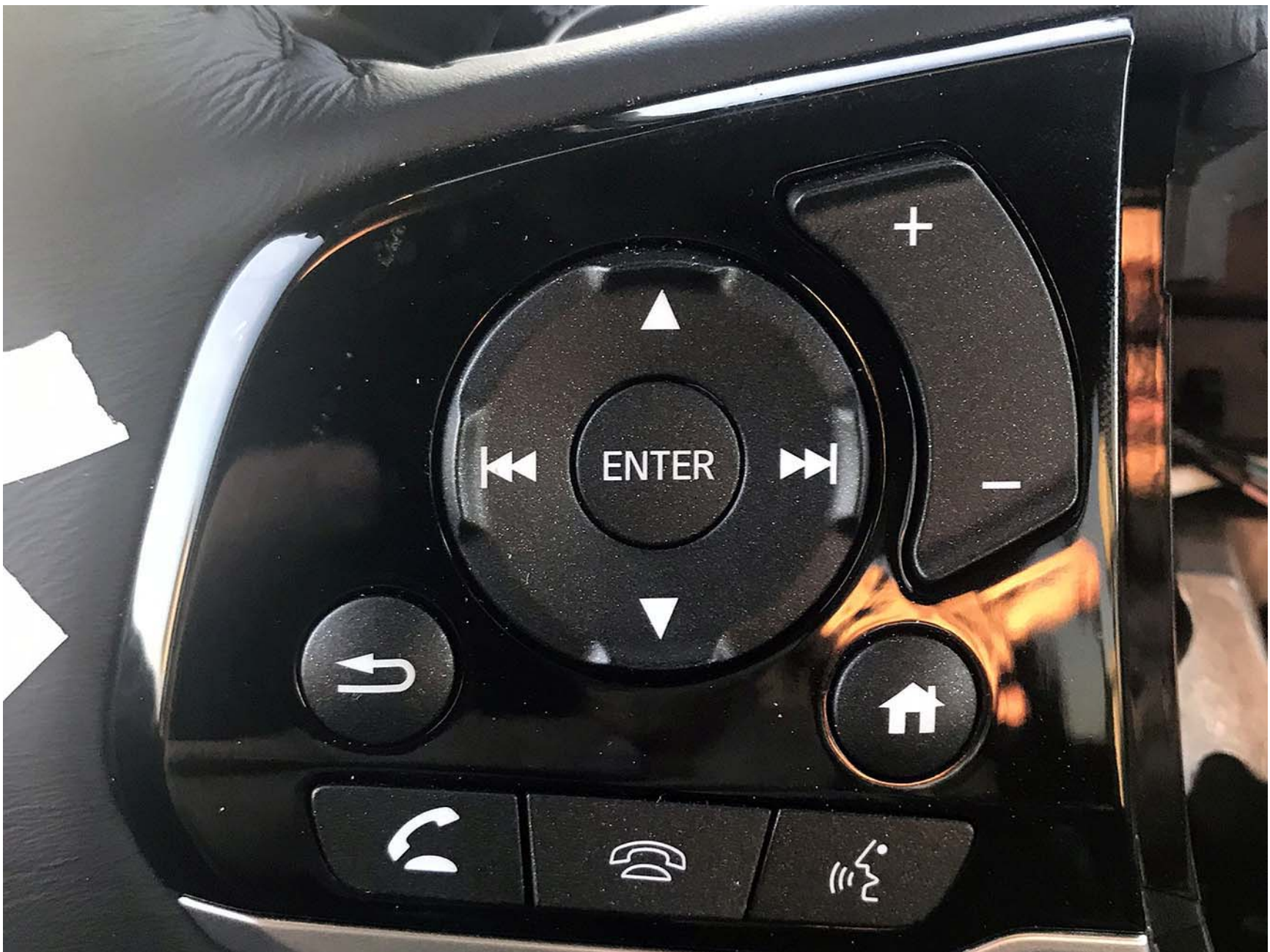
Figure A17. Steering Wheel Mounted Control Buttons for Changing Parameters
