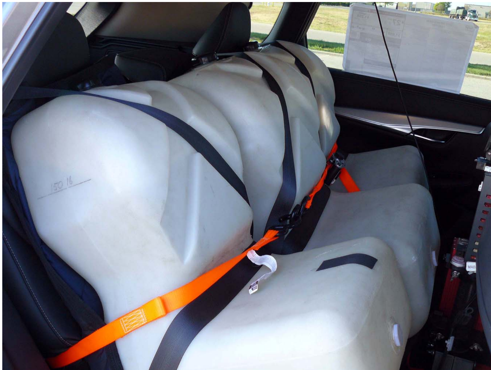
Figure A10. Ballast Condition
