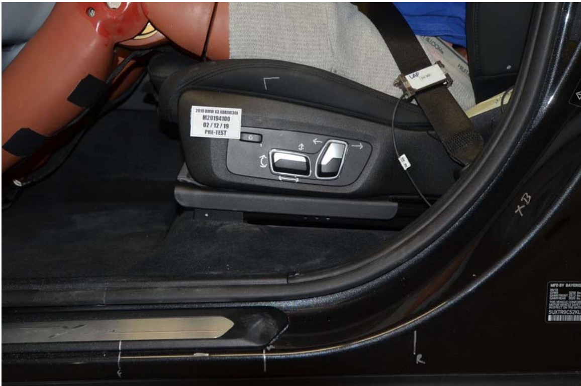
FIGURE 36. Pre-Test Driver's Seat Fore-Aft Markings
