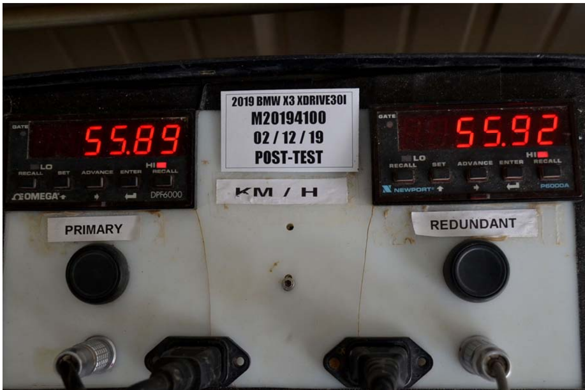
FIGURE 72. Post-Test Speed Trap Read-Out
