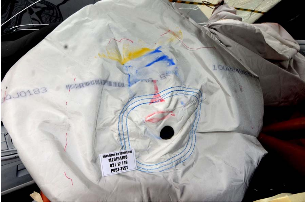
FIGURE 47. Post-Test Driver Dummy Contact with Airbag
