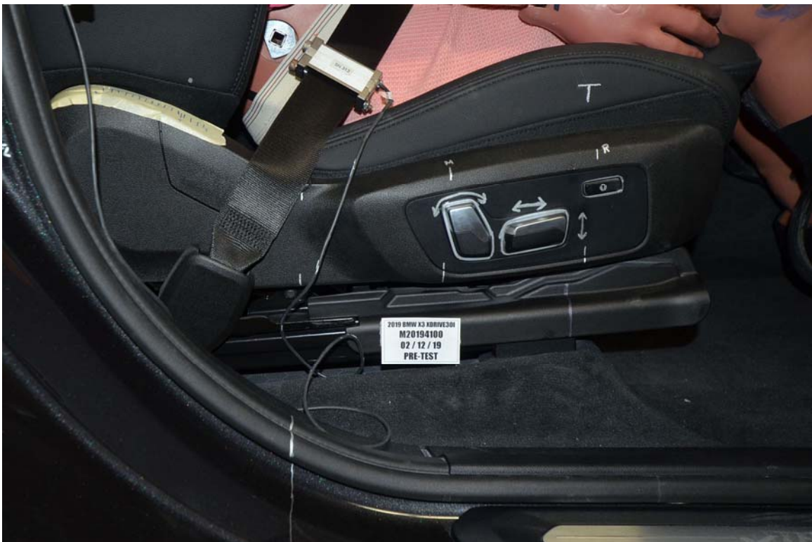
FIGURE 57. Pre-Test Passenger's Seat Fore-Aft Markings
