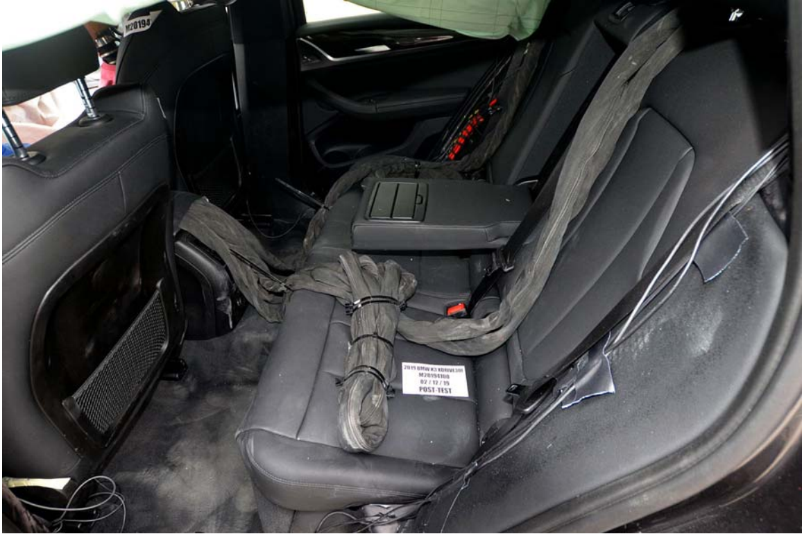
FIGURE 29. Post-Test Dummy Cable Routing
