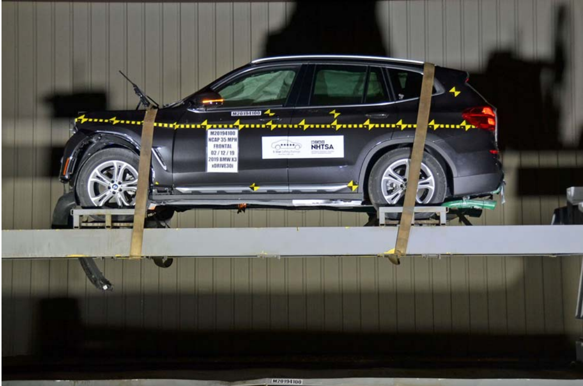
FIGURE 73. Vehicle at 0° on Static Rollover Device
