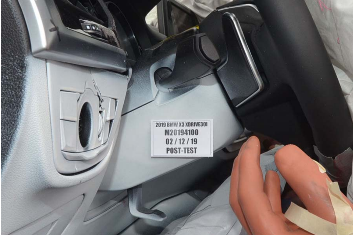
FIGURE 50. Post-Test View of the Steering Wheel
