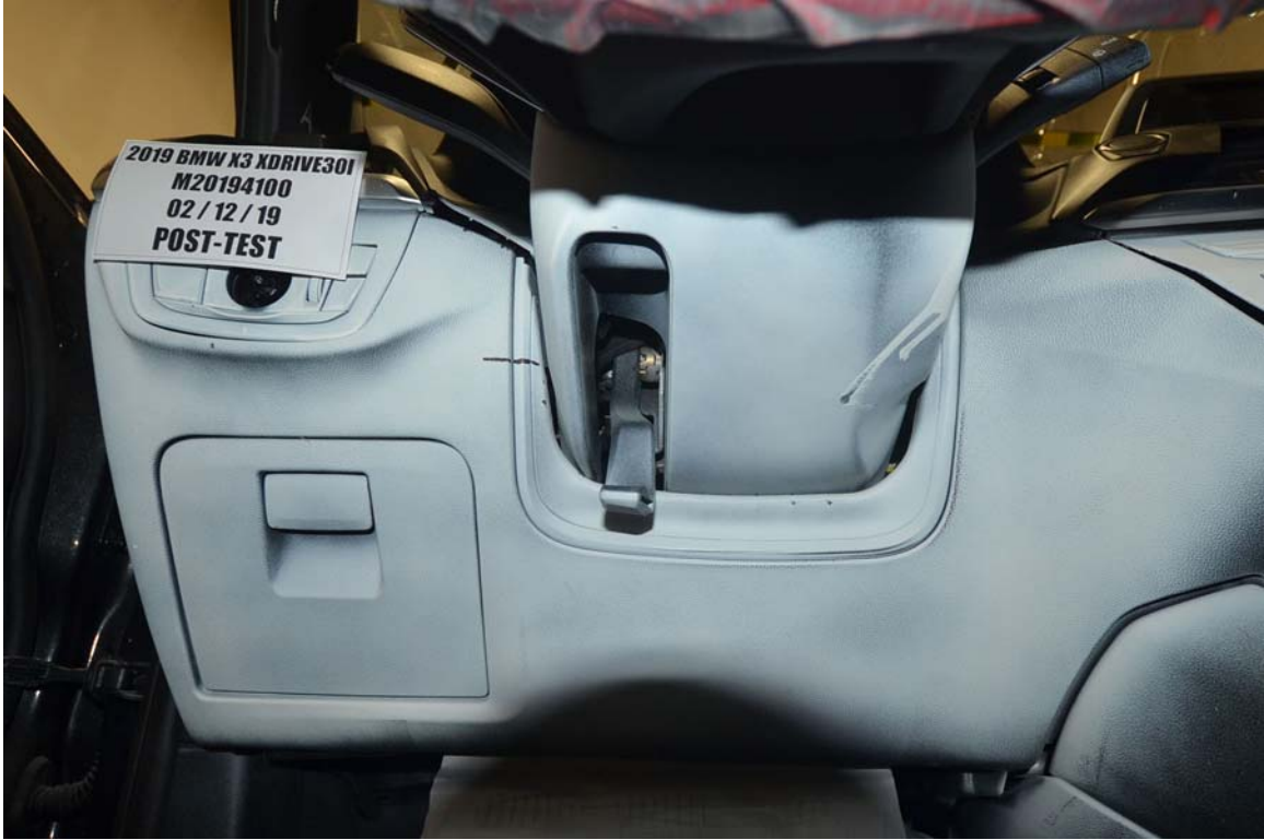
FIGURE 43. Post-Test Driver's Side Knee Bolster
