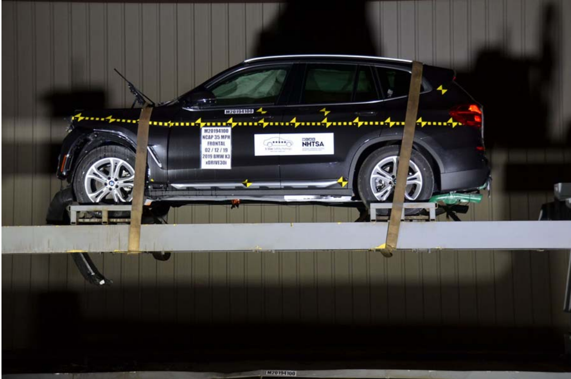
FIGURE 77. Vehicle at 360° on Static Rollover Device
