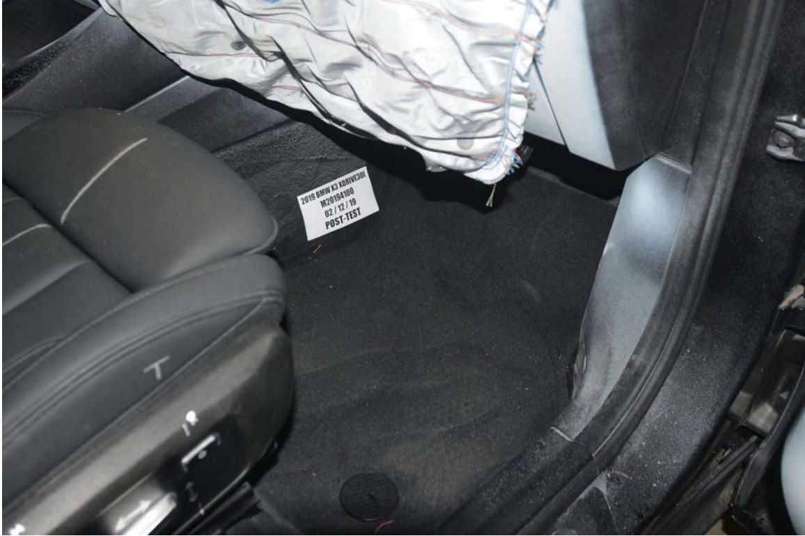
FIGURE 66. Post-Test Passenger's Side Floorpan
