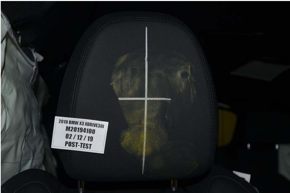
FIGURE 69. Post-Test Passenger Dummy Contact with Headrest
