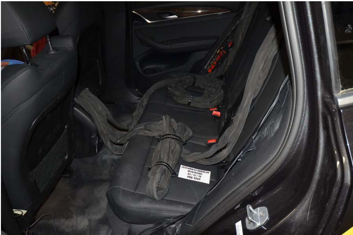
FIGURE 28. Pre-Test Dummy Cable Routing
