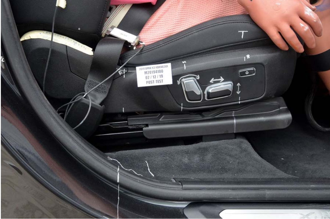
FIGURE 58. Post-Test Passenger's Seat Fore-Aft Markings
