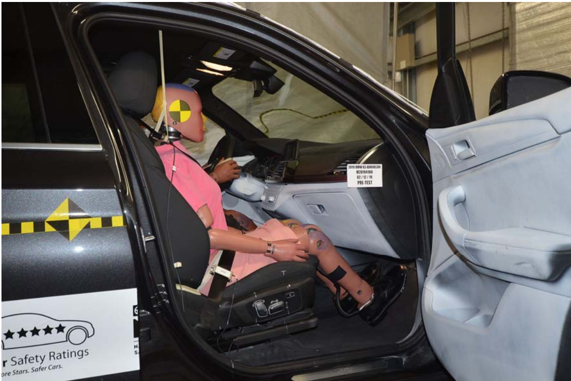
FIGURE 55. Pre-Test Passenger Dummy and Vehicle Interior View
