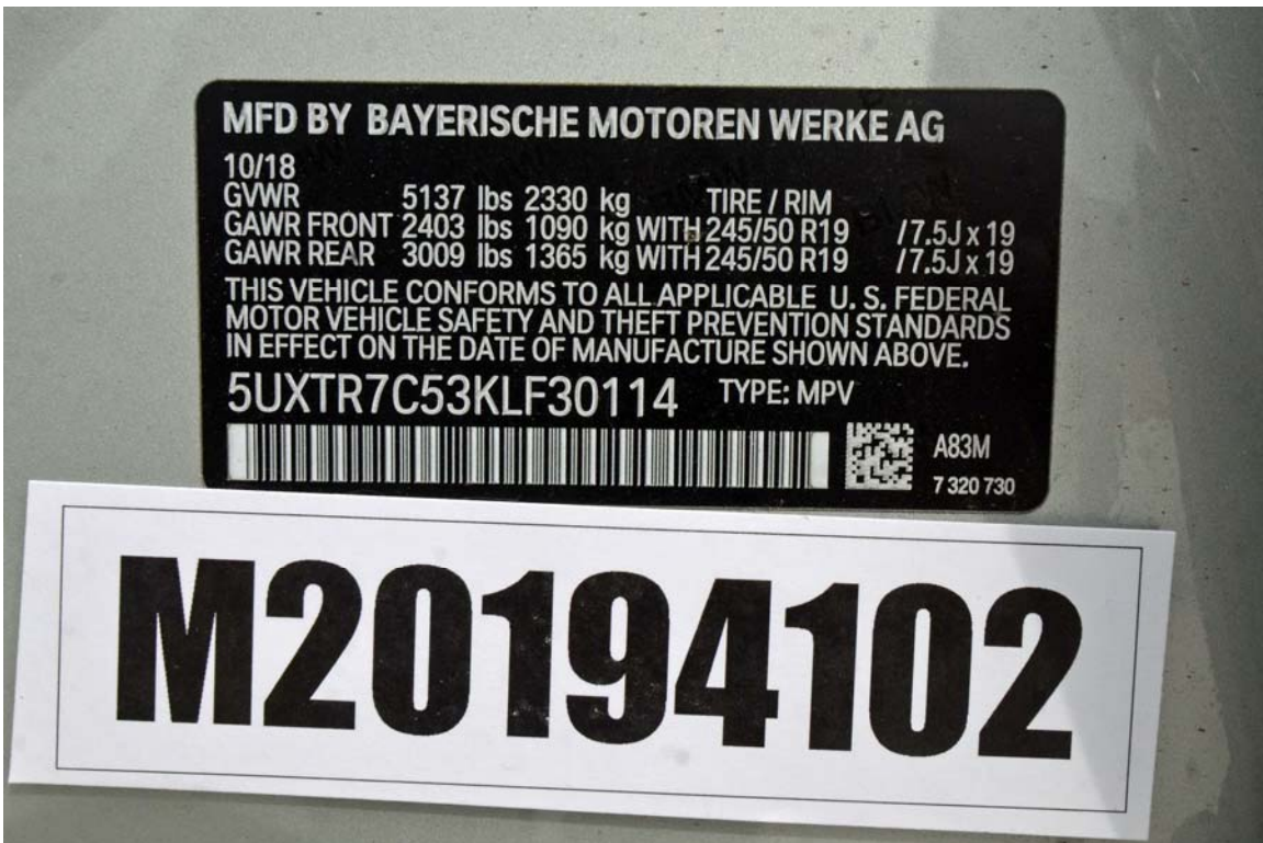
FIGURE 92. Close-Up View of Vehicle's Certification Label
