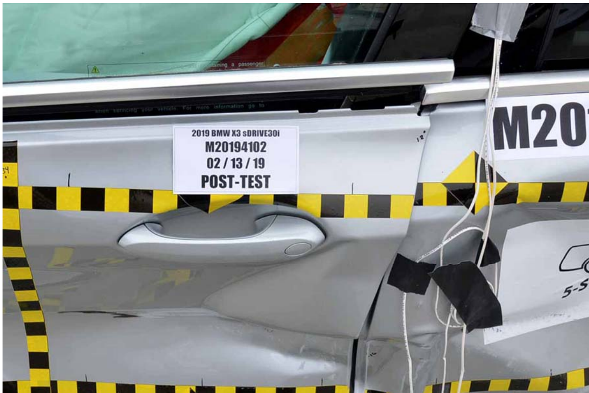
FIGURE 22. Post-Test Left Front Door Latch Close-Up
