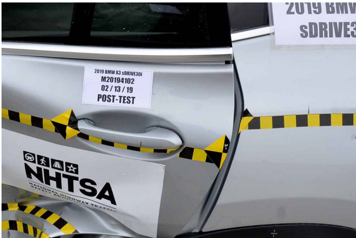
FIGURE 24. Post-Test Left Rear Door Latch Close-Up
