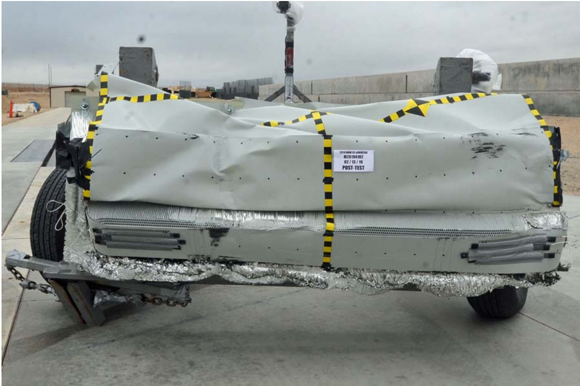
FIGURE 85. Post-Test Front View of MDB Impactor Face
