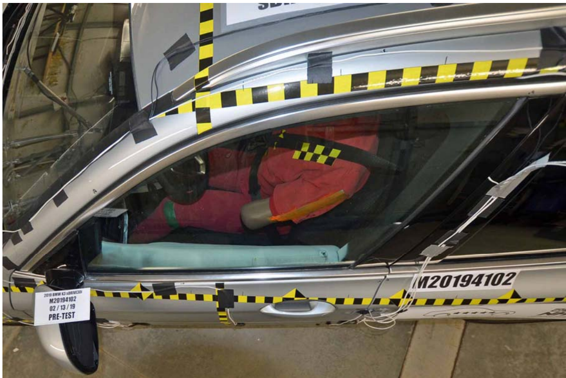
FIGURE 42. Pre-Test Driver Dummy and Door Clearance View
