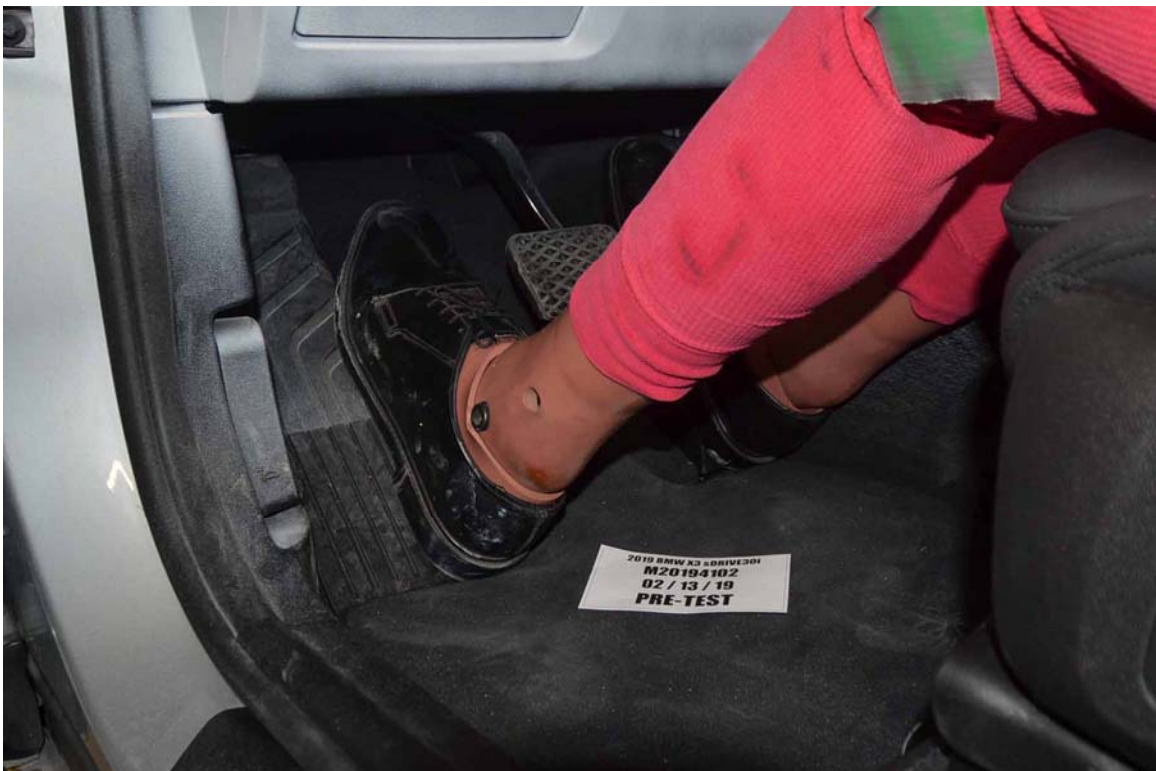
FIGURE 34. Pre-Test Placement of Driver Dummy's Feet
