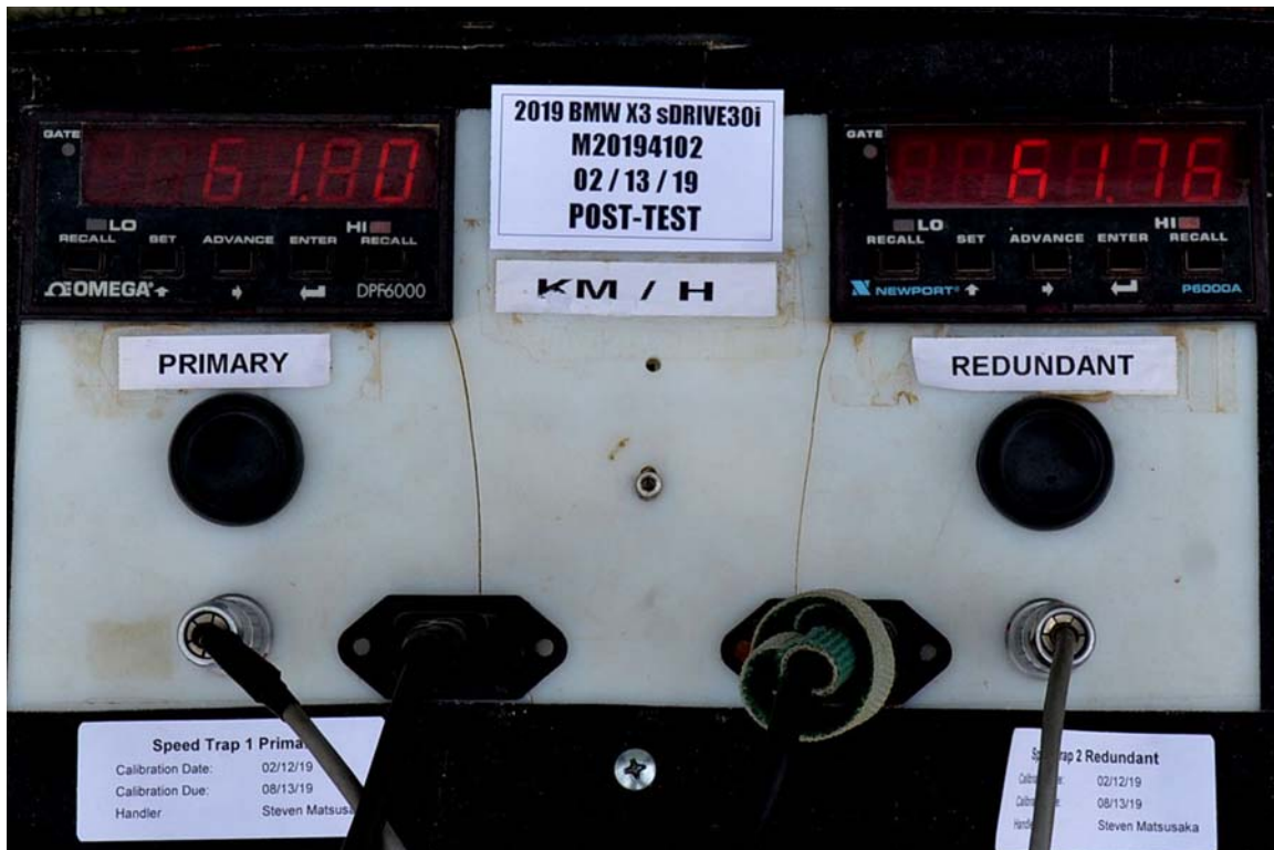
FIGURE 95. Post-Test Primary and Redundant Speed Trap Read-Out
