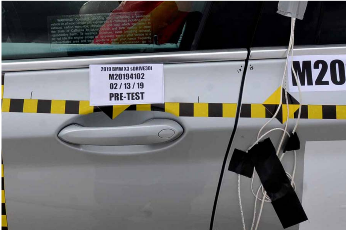
FIGURE 21. Pre-Test Left Front Door Latch Close-Up
