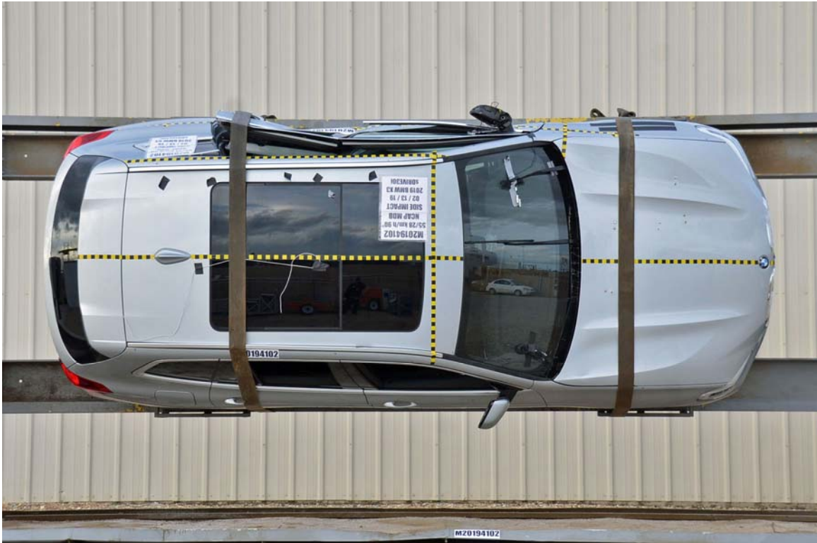
FIGURE 97. FMVSS No. 301 Static Rollover 90 Degrees
