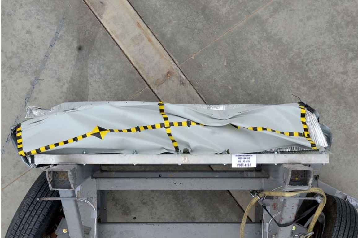
FIGURE 87. Post-Test Top View of MDB Impactor Face
