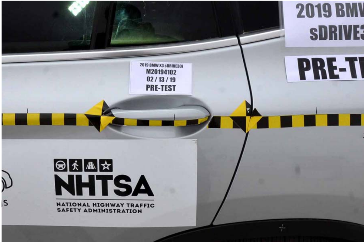
FIGURE 23. Pre-Test Left Rear Door Latch Close-Up
