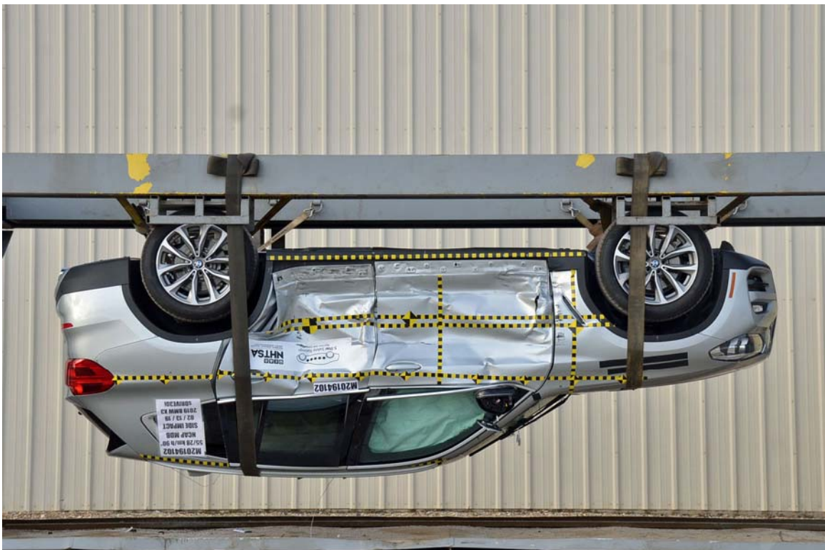
FIGURE 98. FMVSS No. 301 Static Rollover 180 Degrees
