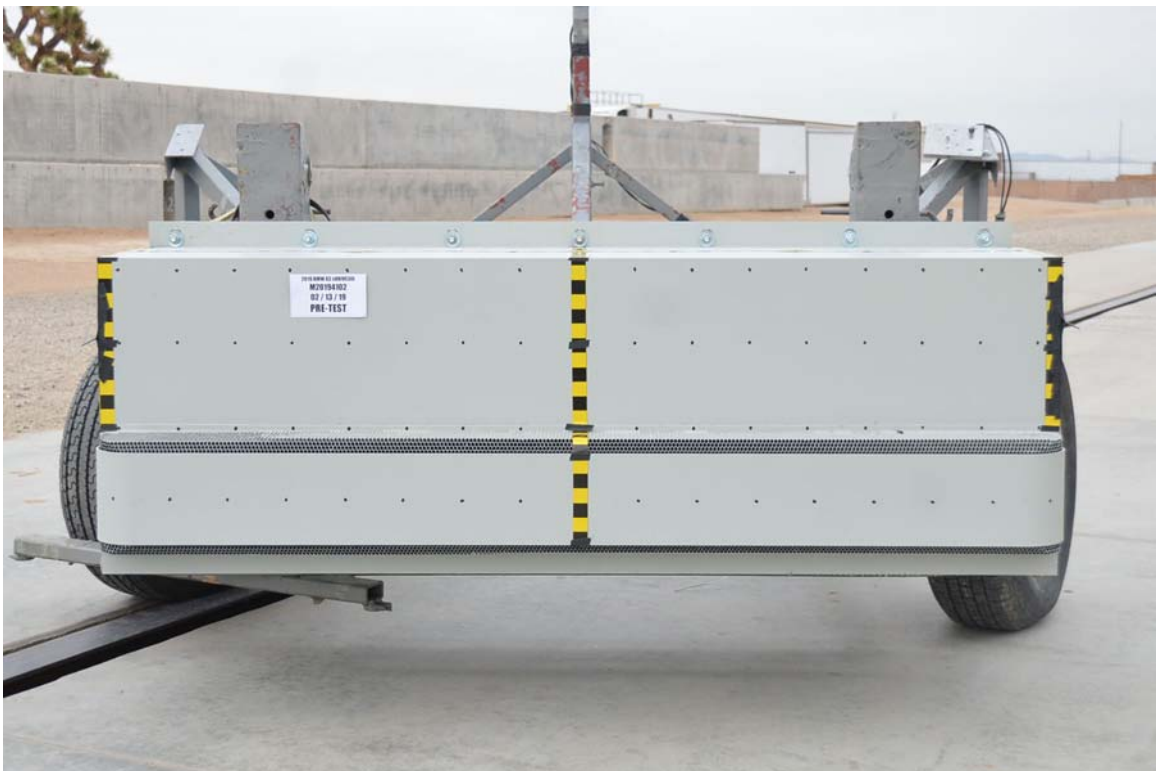
FIGURE 84. Pre-Test Front View of MDB Impactor Face
