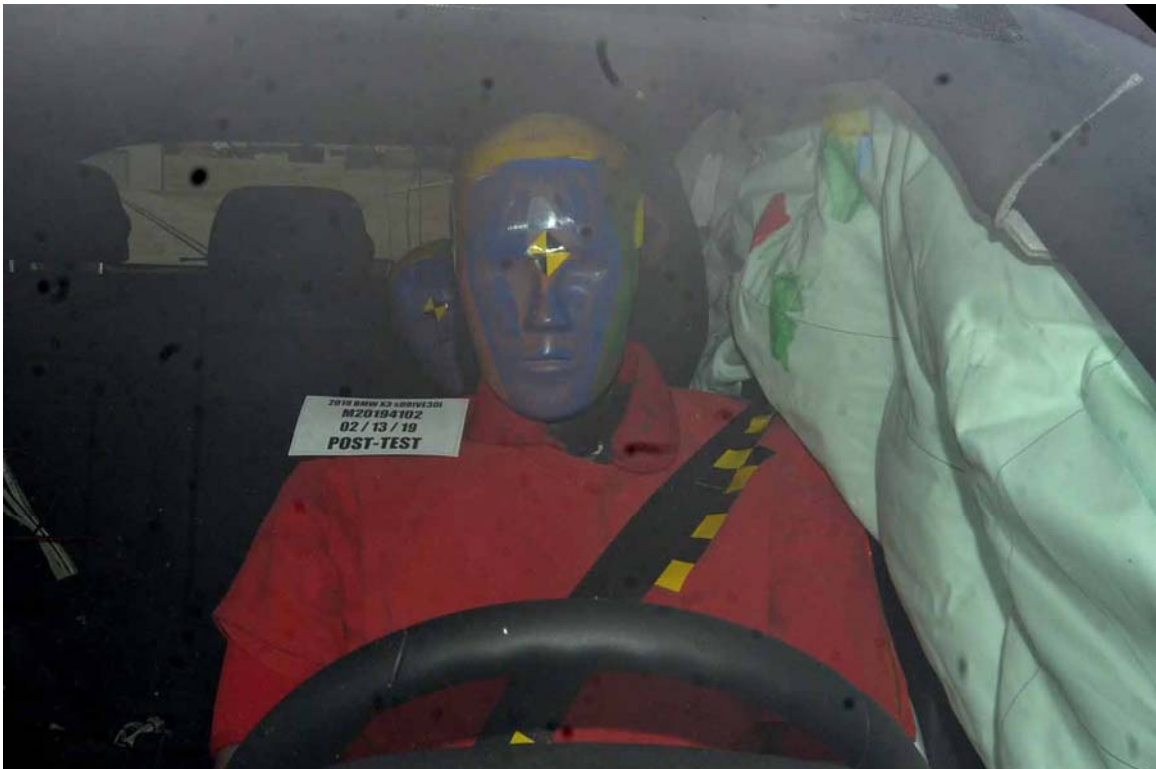
FIGURE 26. Post-Test Front Close-Up View of Driver Dummy
