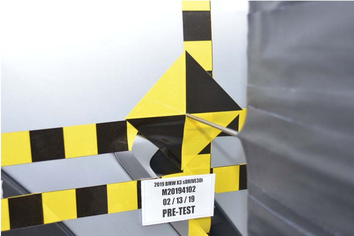
FIGURE 19. Pre-Test Close-Up View of Impact Point Target
