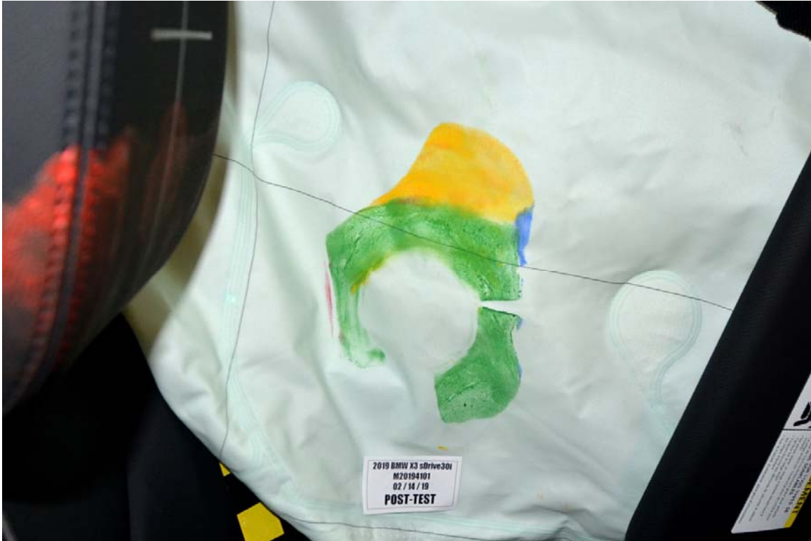
FIGURE 47. Post-Test Dummy Close-Up Head Contact With Side Airbag View
