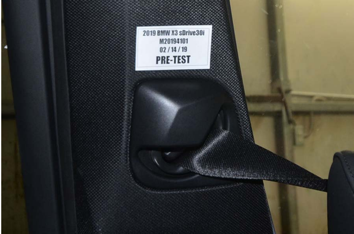
FIGURE 33. Pre-Test View of Belt Anchorage for Dummy
