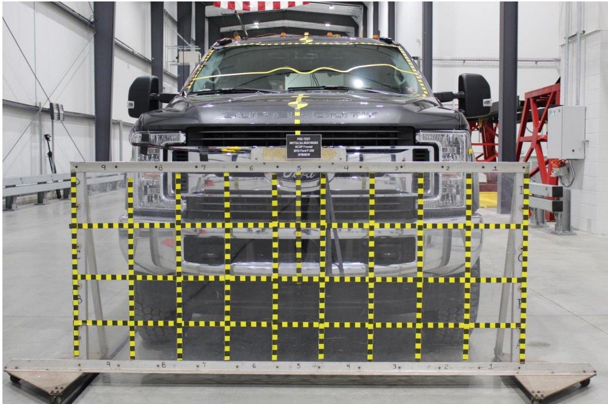
Figure A-1: Load Cell Location
