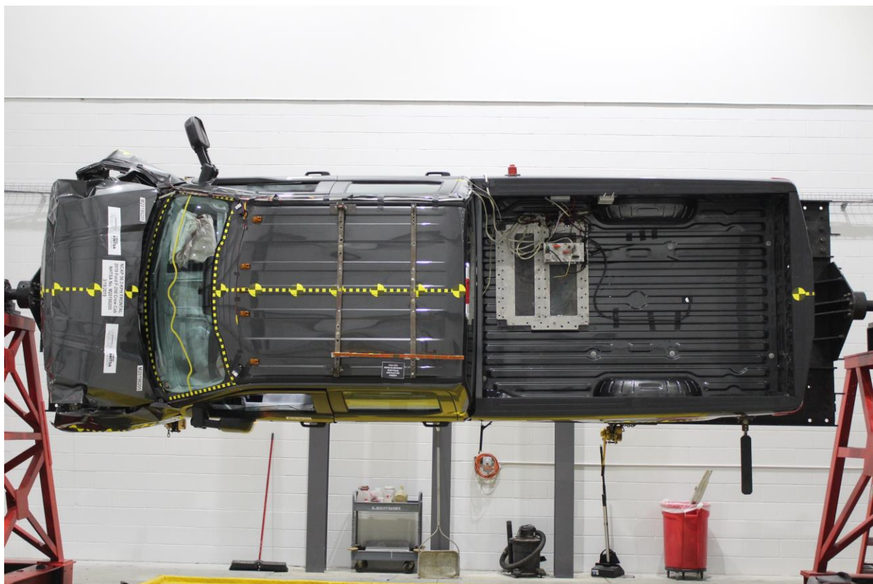
Figure A-74: Vehicle at 90° on Static Rollover Device
