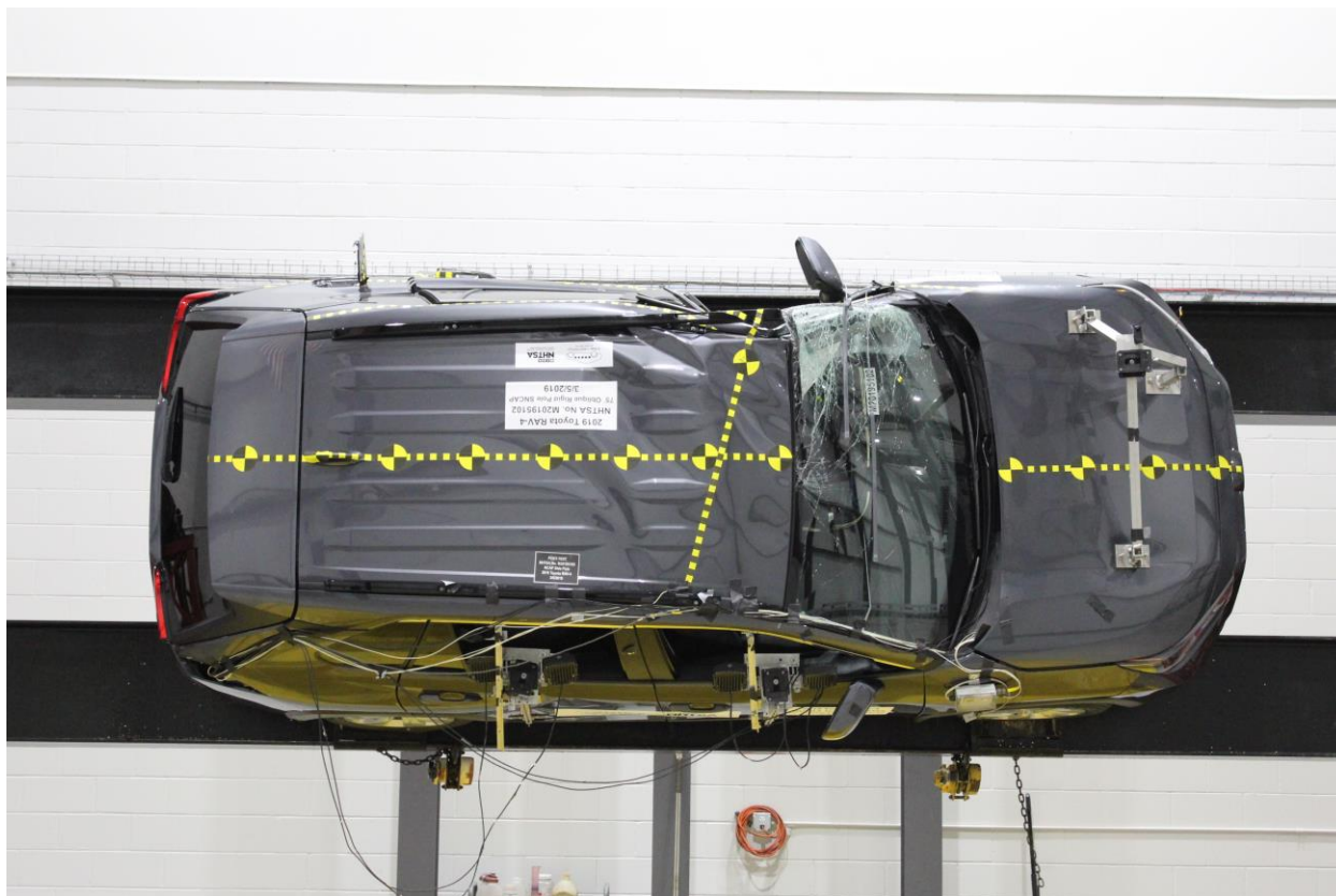
Figure A-66: FMVSS No. 301 Static Rollover 270 Degrees
