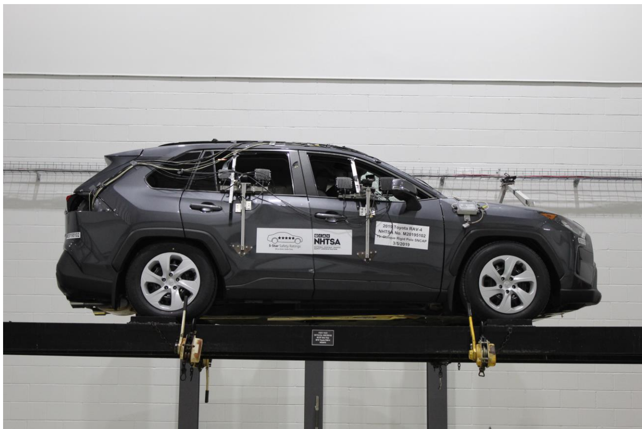
Figure A-63: FMVSS No. 301 Static Rollover 0 Degrees
