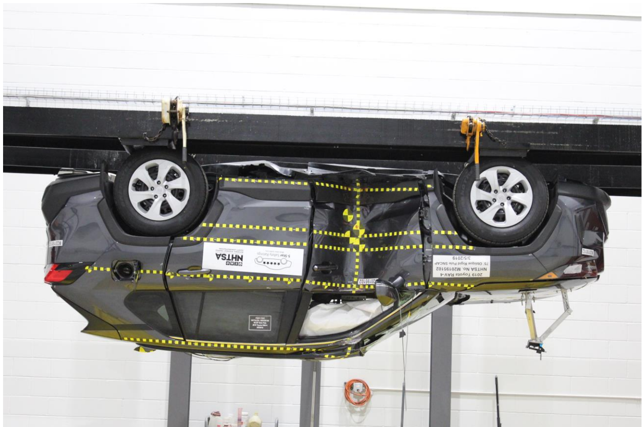
Figure A-65: FMVSS No. 301 Static Rollover 180 Degrees
