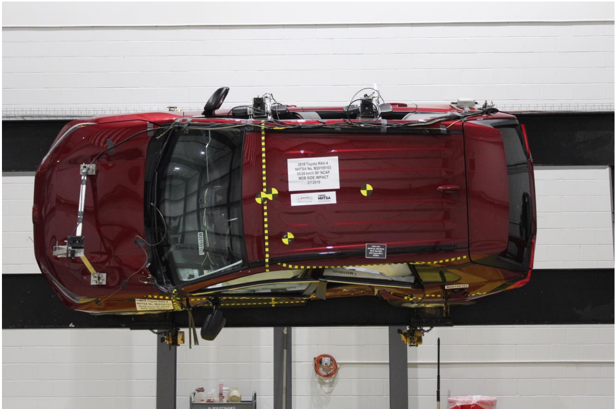
Figure A-97: FMVSS No. 301 Static Rollover 90 Degrees
