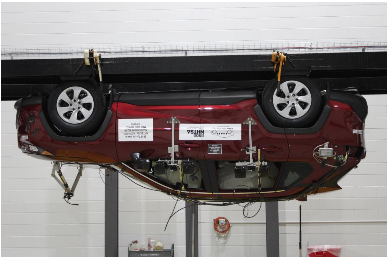
Figure A-98: FMVSS No. 301 Static Rollover 180 Degrees
