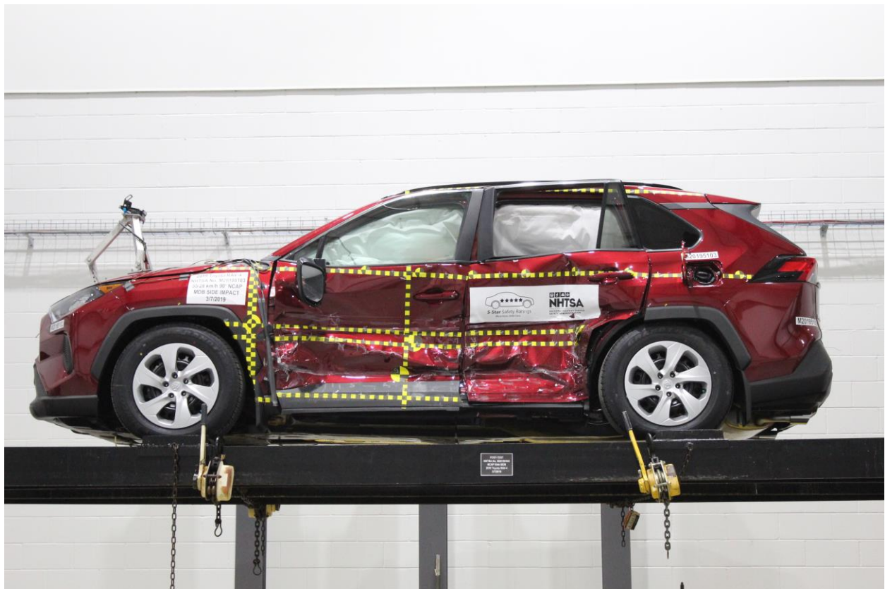
Figure A-100: FMVSS No. 301 Static Rollover 360 Degrees
