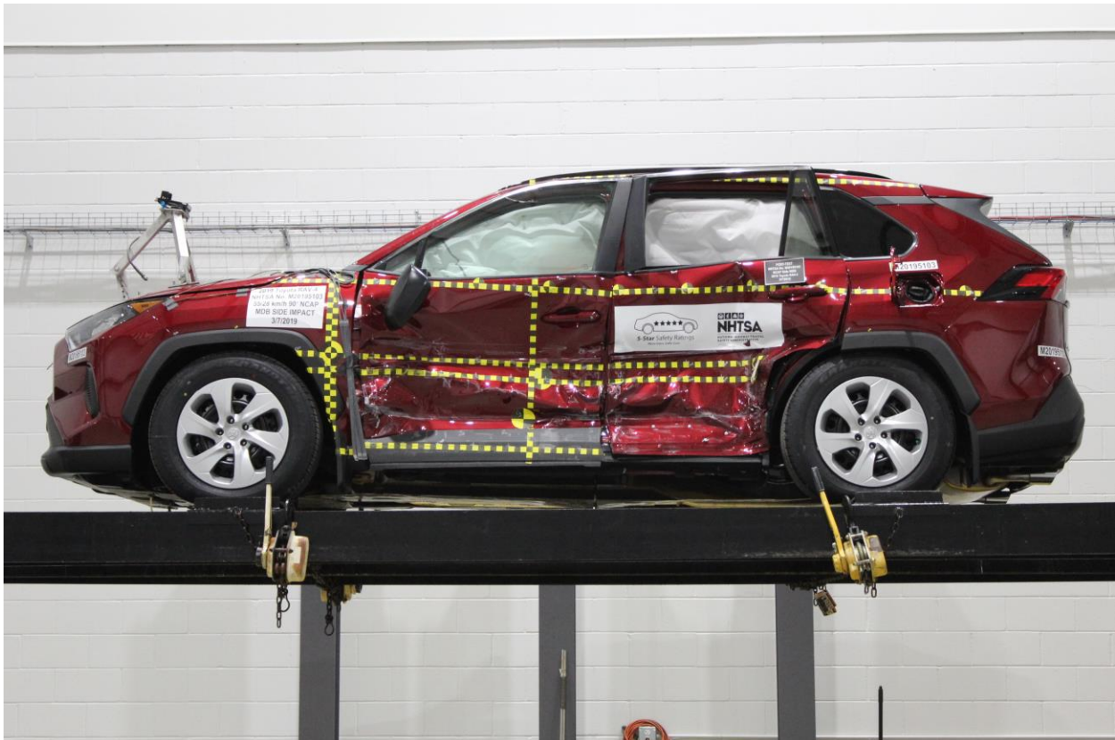
Figure A-96: FMVSS No. 301 Static Rollover 0 Degrees
