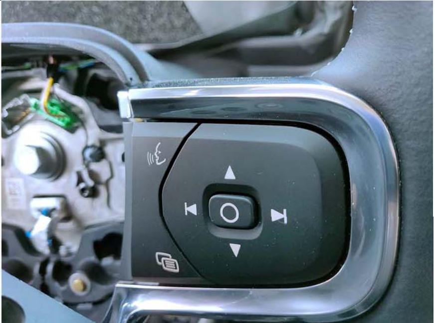
Figure A15. Steering Wheel Mounted Control Buttons for Changing Parameters
