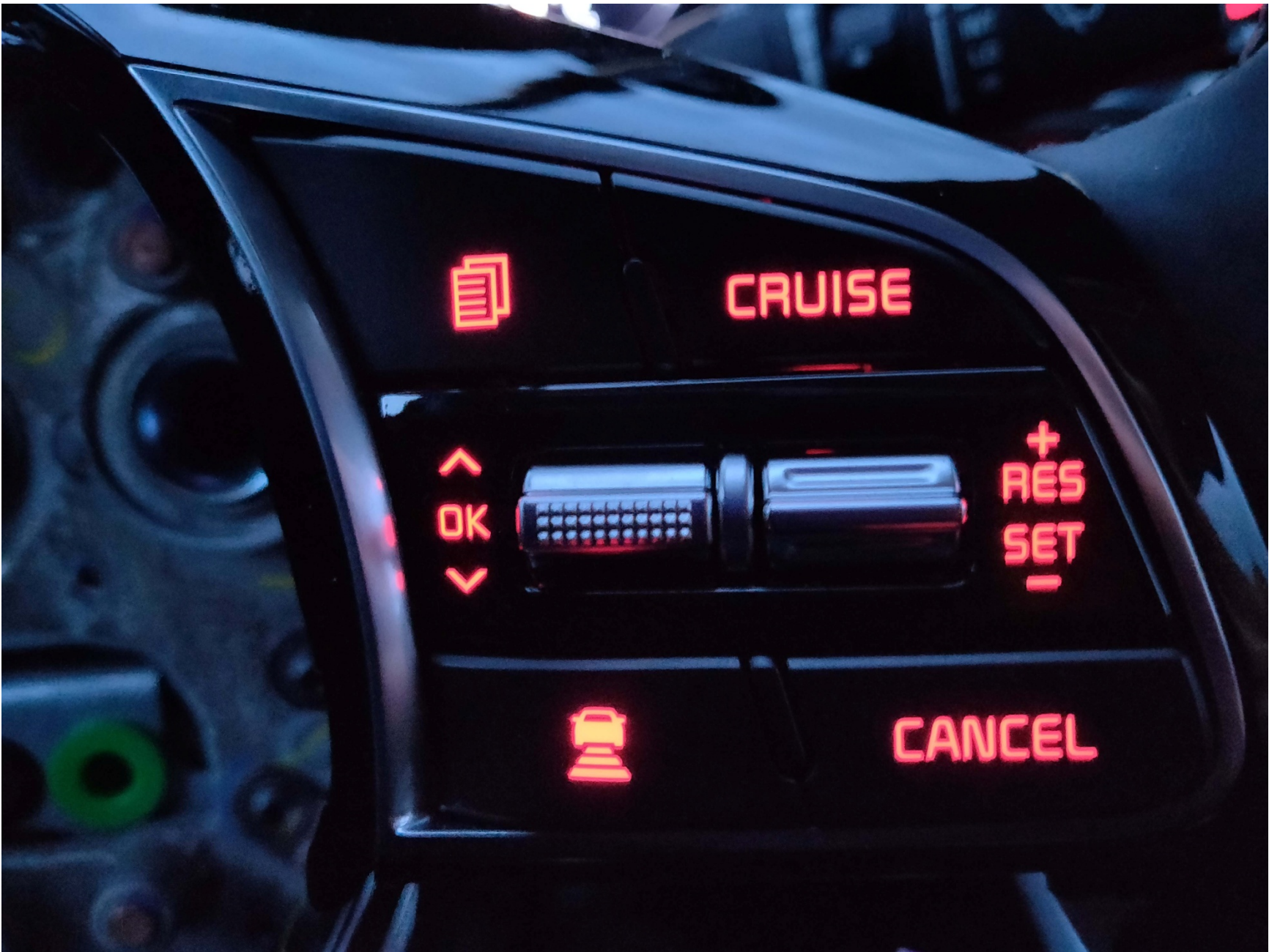
Figure A16. Steering Wheel Mounted Controls for Changing Parameters
