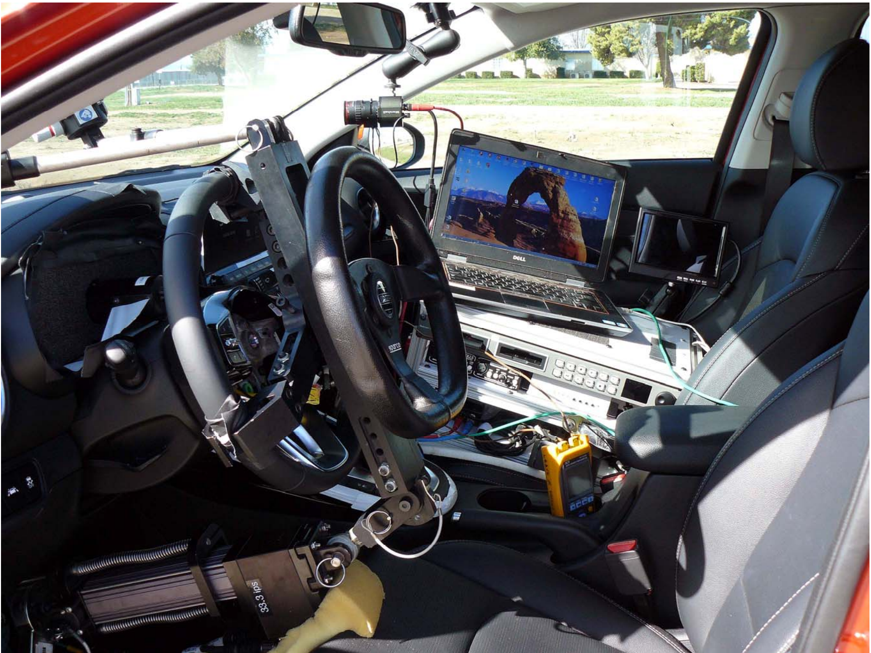
Figure A12. Computer Installed in Subject Vehicle
