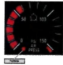
For Mack LR model vehicles, two pressure gauges, low air telltale, popup in the display, and an audible alarm are provided.
