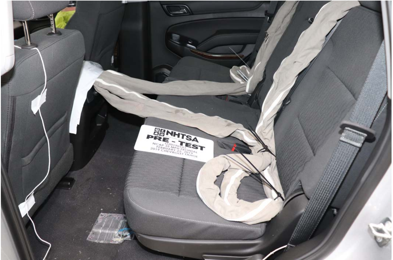
Photo No. 028 - Pre-Test Dummy Cable Routing
