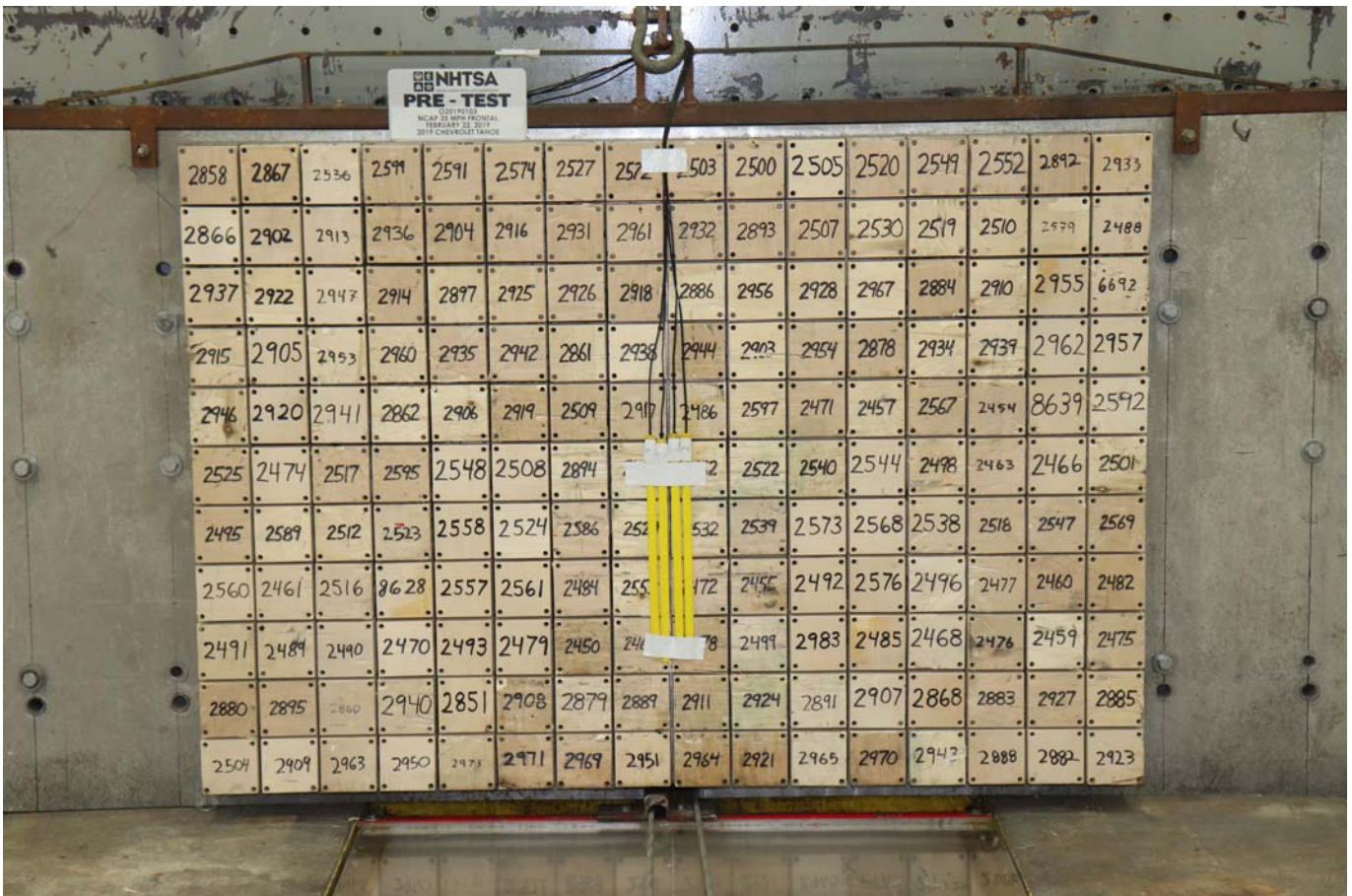
Photo No. 002 - Pre-Test Load Cell Wall
