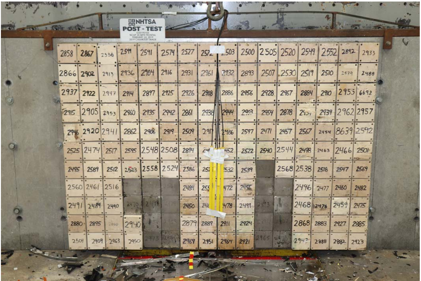
Photo No. 003 - Post-Test Load Cell Wall
