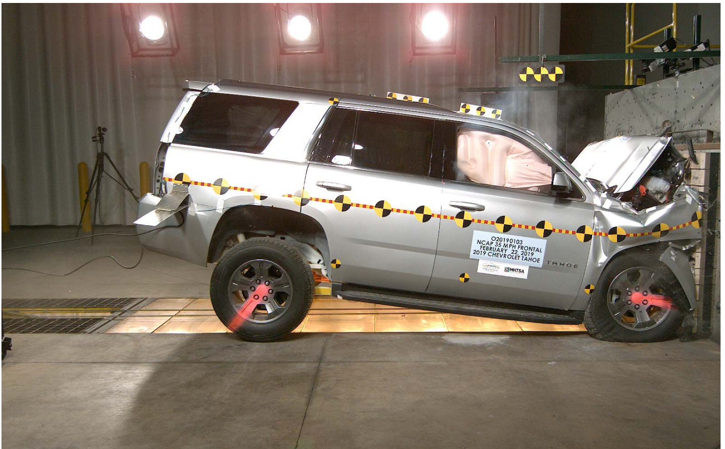
Photo No. 078 - 2019 Chevrolet Tahoe 4WD LS 5-Door SUV Frontal Impact Event
