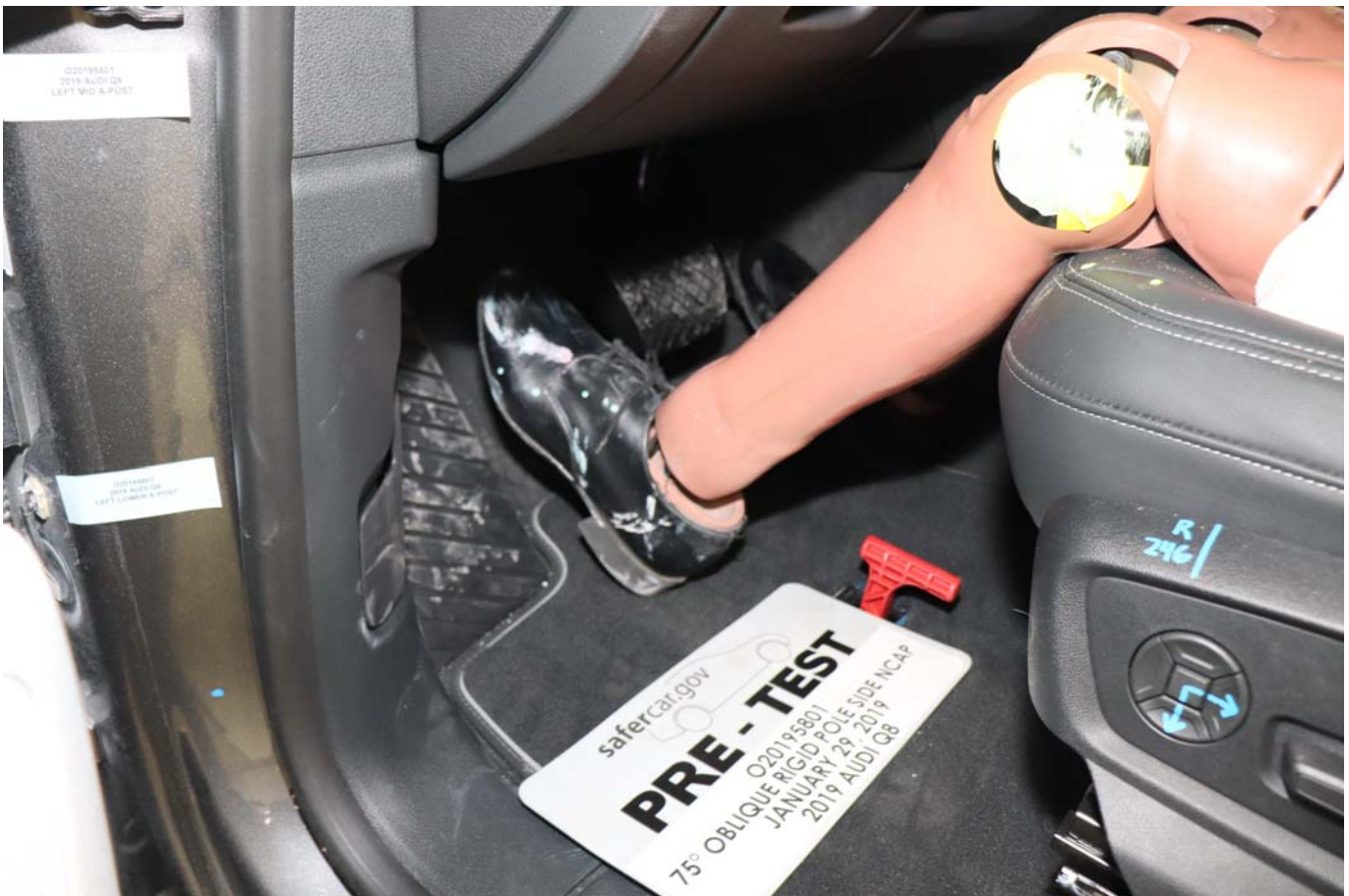
Photo No. 032 - Pre-Test Placement of Dummy Feet
