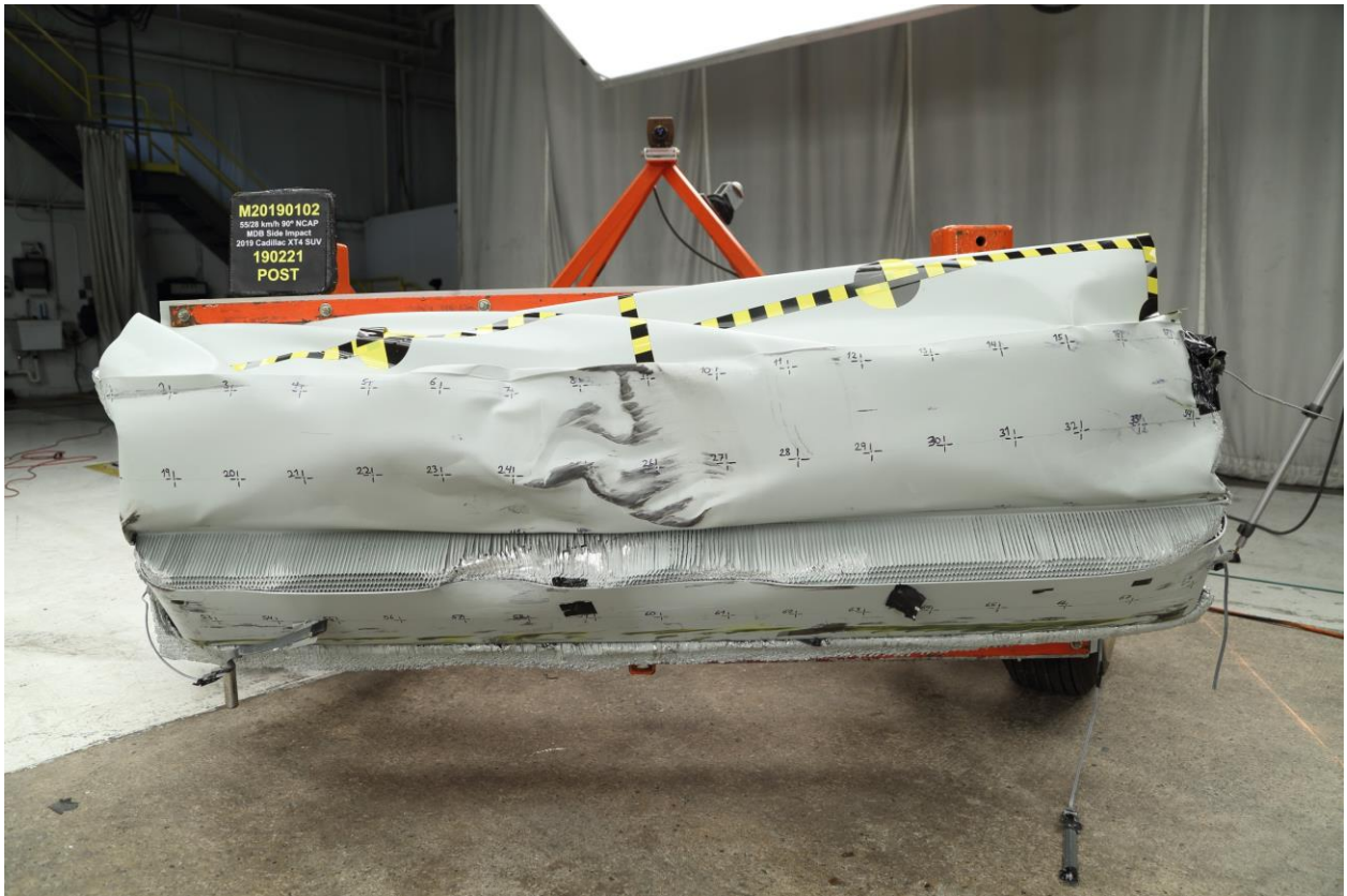
085 Post-Test Front View of MDB Impactor Face
