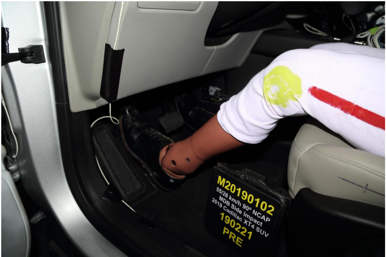
034 Pre-Test Placement of Driver's Dummy Feet
