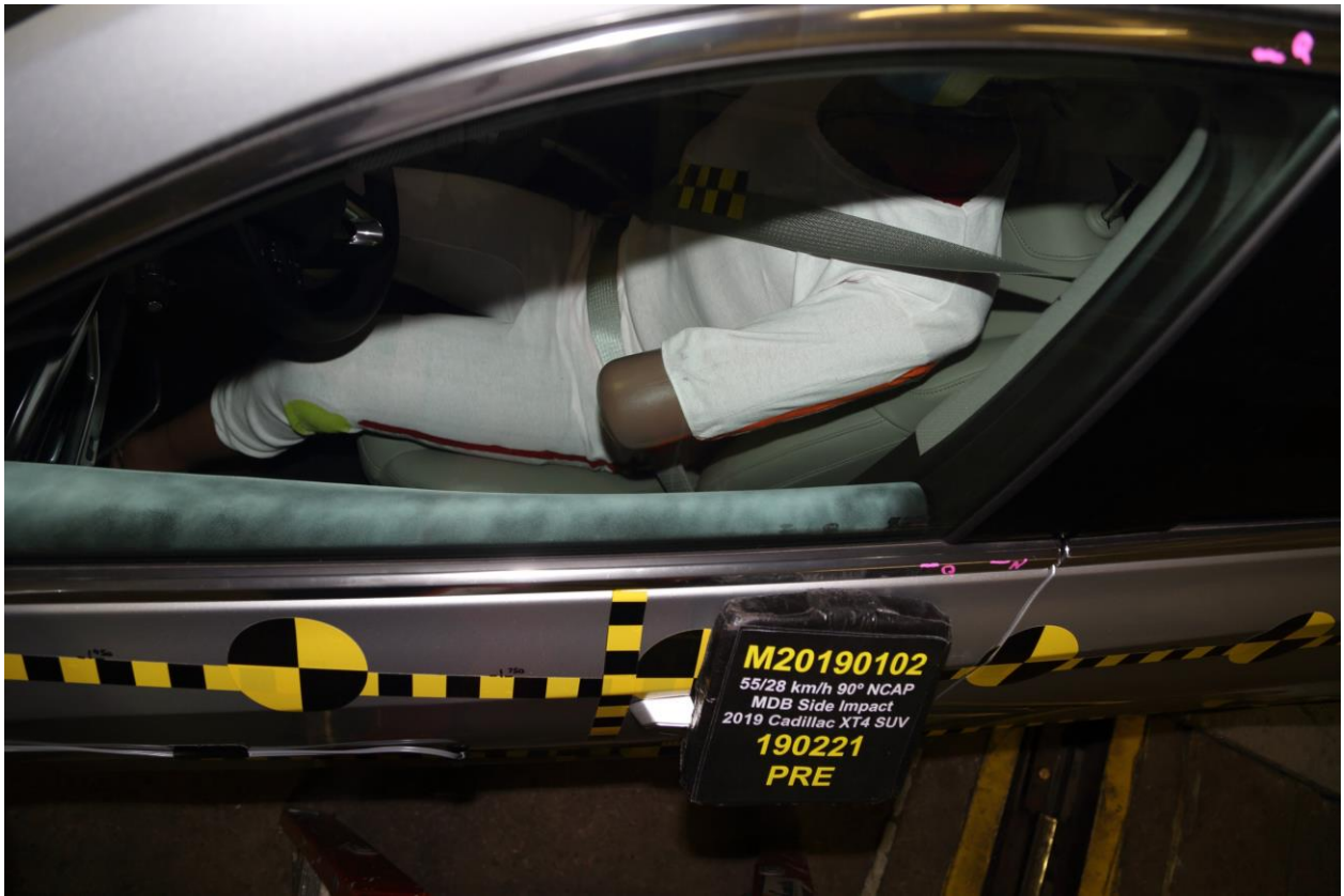
042 Pre-Test Driver Dummy and Door Clearance View
