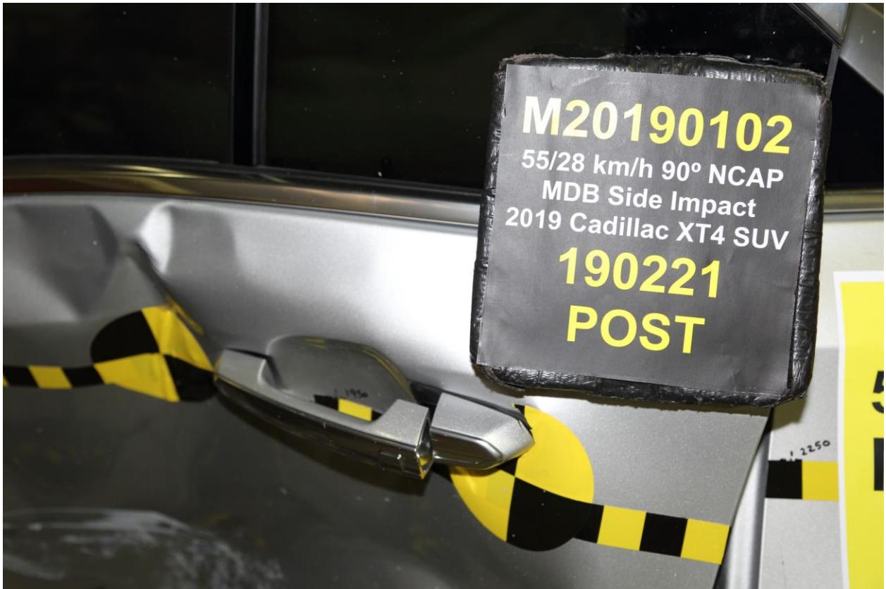
024 Post-Test Left Rear Door Latch Close-Up
