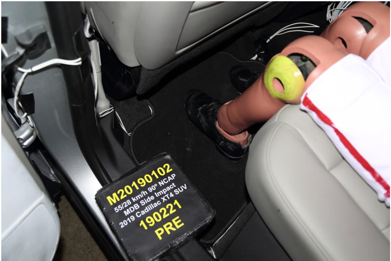
064 Pre-Test Placement of Rear Passenger Dummy's Feet
