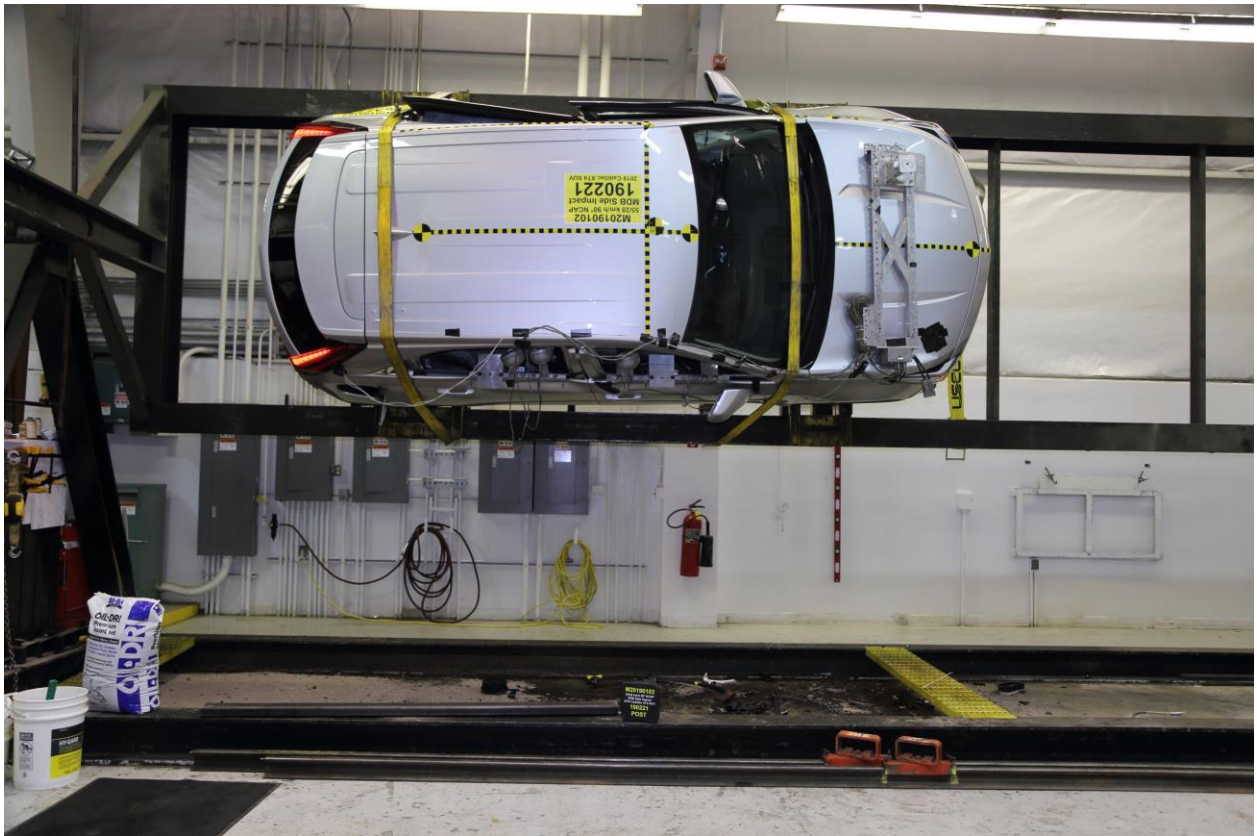
097 FMVSS No. 301 Static Rollover 90 Degrees
