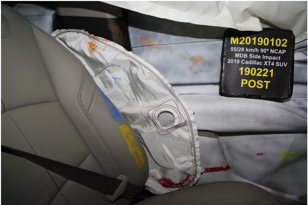
051 Post-Test Driver Dummy Close-Up Torso Contact with Side Airbag View
