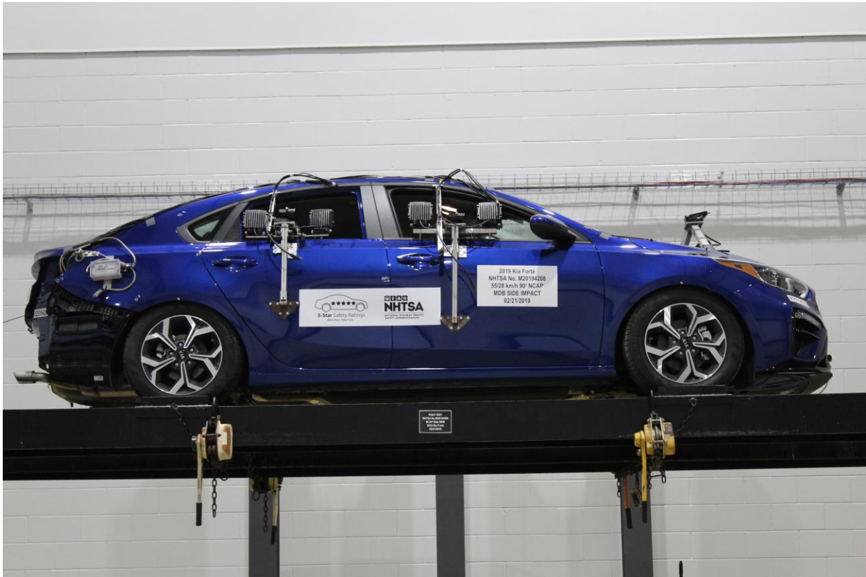
Figure A-96: FMVSS No. 301 Static Rollover 0 Degrees
