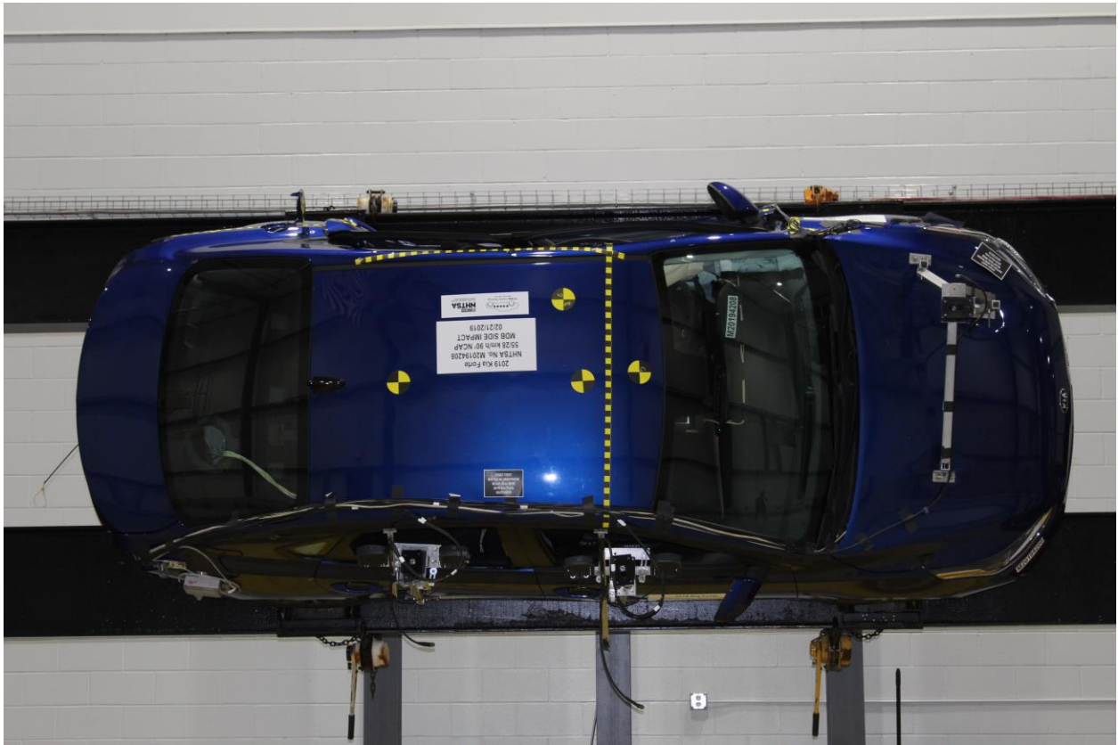
Figure A-97: FMVSS No. 301 Static Rollover 90 Degrees
