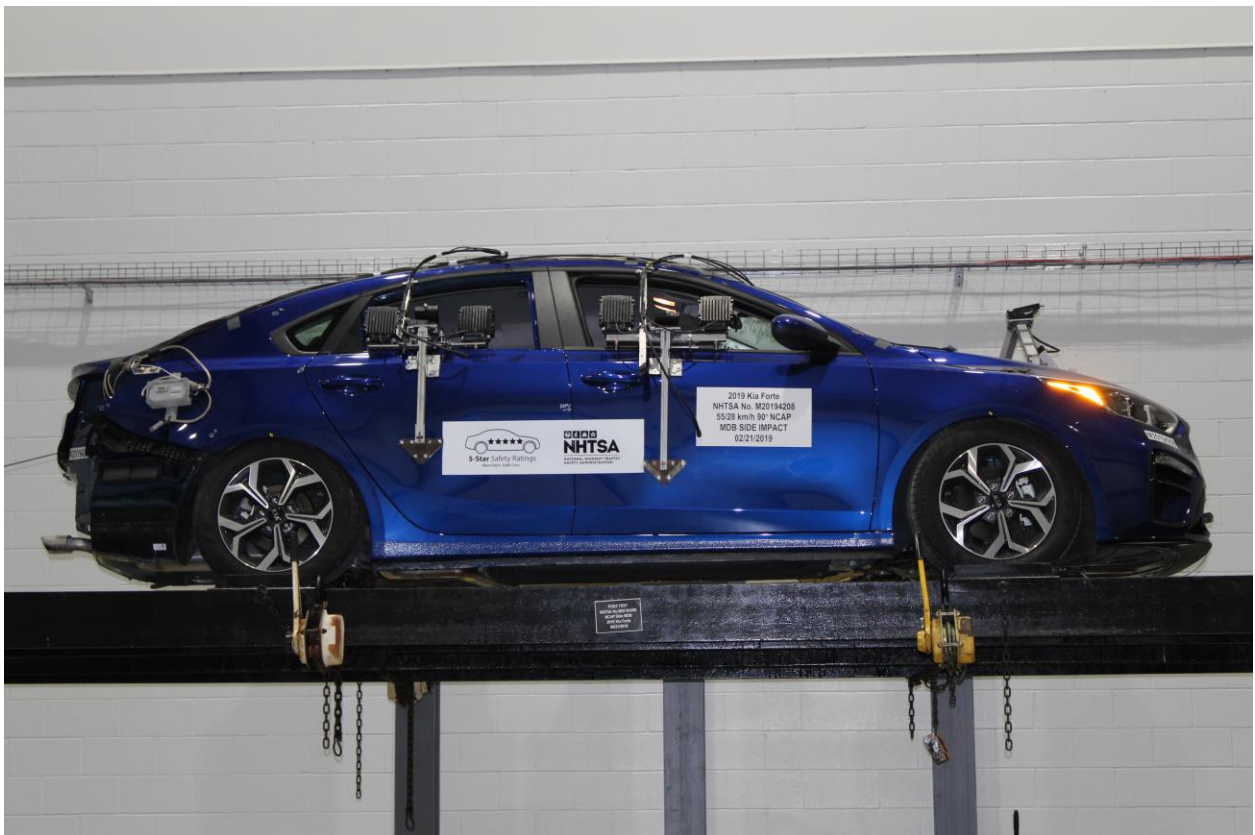
Figure A-100: FMVSS No. 301 Static Rollover 360 Degrees
